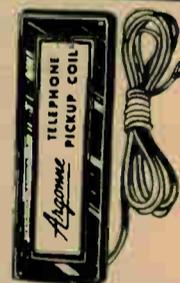
Induction telephone pickup. Telephone conversations can now be picked up with no tapping of wires or special telephone circuits. Simply place the phone base, either cradle or upright type, on the pickup platform and connect the leads to the high impedance input of any medium gain audio amplifier, or directly to any tape, disc or wire recorder. Shpg. wt. 8 oz. MS-16 Net 1.95
