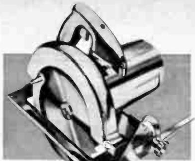
Dependable power saw provides reserve power to cut thru 2x4's with ease. Powerful 10 amp., 5000 RPM motor. Cuts up to 2 3/4" vertically and 2 3/4" at 45°. Balanced for one hand operation. Features heavy-duty bronze bearings, removable rip guide, floating blade guard, and easily set depth and angle adjustments. With combination blade included. For 115 VAC. 60 Hz. 3-cond. power cord. UL listed. Shpg. wt., 13 lbs.
