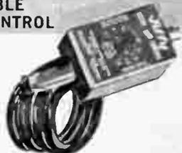
Dependable motor speed control ideal for workshop power tools using universal AC-DC and series DC motors. Assures constant speed variation from zero rpm to maximum speed. Has built-in circuit breaker. 5 amps load rating. Input: 120 volts 50-60 Hz AC. 3-wire receptacle and line cord. 3x2 1/2 x 1 1/4" D. Shpg. wt., 1 lb.
