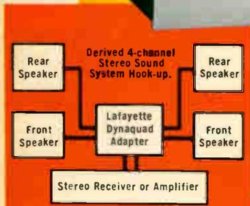
Just add the Lafayette Dynaquad adapter and two more speakers to convert your present 2-channel stereo system to a sensational derived 4-channel stereo surround system.
