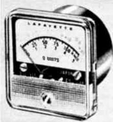
Highly accurate. Features wide viewing angle and 3-color scale. Front panel zero adjustment. Calibrated scales (1 MA full scale), 0 to 100% modulation, "S" units 0-9, also +10 and +30. Linear full scale markings of 0 to 5. Dimensions: dial face, 1 5/8"; depth 1 1/4" overall. Supplied with 4 mounting screws and lugs. For 6 or 12 volts. Dust resistant case. Shpg. wt., 8 oz. Imported.
