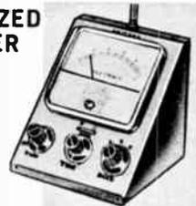
Covers 2.530 Mc to 57,000 Mc in 3 bands. Ideal for use with ham, Citizens Band or other transmitters within this frequency range. Enables user to tune his transmitter and antenna for maximum RF output. 200  $\mu$ a meter is calibrated from 0 to 10. Earphone jack provided. Front panel controls: gain on-off switch, tuning, and band selector switch. Battery powered—can be operated anywhere. With telescoping antenna and battery. Imported. Shpg. wt., 2 lbs.
