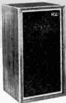
Features Frequency Discriminating Decoupling which results in considerable reduction in distortion plus smooth response free of phase shift. Response: 35-20,000 cps. ±3 db. Special 8" linear-travel piston cone woofer; hi-flux mylar dome tweeter. Impedance: 8 ohms. Power: 6 watts min. to 60 watts max. Oiled walnut finish. 22¾x13x11¾". Shpg. wt., 35 lbs.
