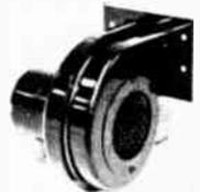
Efficient, quiet, dependable and economical. Usable in many applications—air distribution in confined areas, exhaust fumes and gas, etc. Suitable for ventilation equipment in home, marine and commercial use. Welded pressed steel housing. Shaded-type motor for efficient, quiet operation. Moves 150 cubic feet of air per minute. Mounting flange, 5 1/2" x 4". 10" AC line cord and plug. 110V, 60 cycles; 1.4 amp. Shpg. wt., 7 lbs.
