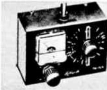
A miniature wavemeter for checking transmitter output. Determines relative strength of fundamental frequency and any harmonic or parasitic radiation. Complete and self-contained, requires no power. Telescoping antenna is included. Tunes 1.6 to 150 mc in four calibrated bands. Only 3 1/4" x 2 3/4" x 1 1/2" D. Antenna is 10 3/4" extended. 3/4" telescoped, is fitted with a banana plug and is removable. Total shpg. wt., 8 oz. Imported.
