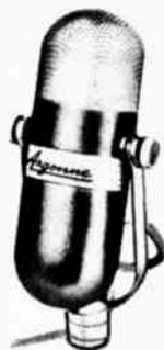
Omnidirectional microphone has a swirl ridged aluminum diaphragm completely sealed and gasketed against high humidity and temperature conditions, for a wide variety of applications. The 360° stirrup shaped bracket provides for mounting with any  $\frac{5}{8}$ "-27 thread stand. Finished in an attractive gunmetal grey with 4½" shielded cable. Shpg. wt., 1 lb. Imported
