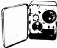
The Intermatic lawn sprinkling system time controls permit completely automatic pre-programmed watering of up to 3 zones. A 24 hour time dial can be set to initiate sprinkling any time during the day while skipper wheels serve to eliminate watering on selected days. Time durations per area are adjustable from 5 to 60 minutes. May be manually operated. Both models are rated at 120 volts, 60 cycle, 5 amps. Gray hammertone case measuring 7¾x5x3". Shpg. wt., 3 lbs.
