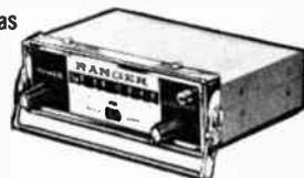
Insert It in its mounting case and it operates on car or boat 12 volt power supply . . . slip it out and you have a powerful lightweight portable with a metallic gold finish, powered by its own penlight batteries (not included). Radio locks in place in car or boat, prevents theft. 8 transistors, diode plus thermistor super-het circuit with H.F. amplifier. 3½" speaker. 12V negative ground, positive ground cars. Shpg. wt., 6 lbs.
