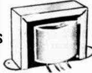
Here is an outstanding value in the most popular transistor output transformer for 10 to 11 ohm speakers. Rated power is 150 milliwatts. Primary impedance is 400 ohms, center-tapped and secondary 11 ohms. DC resistance of primary is 20 ohms and secondary .9 ohms. Size:  $\frac{3}{4} \times \frac{3}{4}$ ". Shpg. wt., 4 ozs. Imported.
