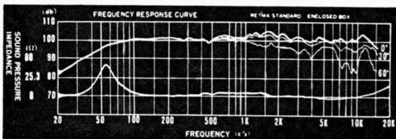
■ 20 TO 20,000 CPS (40 TO 16,000 CPS  $\pm$  3 DB) ■ HIGH EFFICIENCY ■ HIGH EXCURSION WOOFER WITH UNIQUE "CONICAL STIFFENER" ■ HANDLES HEAVY BASS PASSAGES WITHOUT "DOUBLING"
