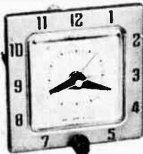
Genuine Telechron mechanism. Complete 12 hour movement. Can be set to turn on any radio, TV or similar electrical appliance at any preset time. Gold finish dial—black lettering. Timer sets from rear. On-off-auto switch in front. Size 3½" square. 1¾" deep. Set shaft extends 5½" to rear. SPST switch, rated 15 amps at 115 volts. For 110-120V, 60 cy. AC only. Shpg. wt., 2 lbs. \*Plus 10% F.E.T. Net 3.95\*
