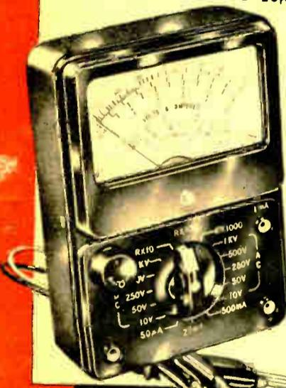
This new multitester incorporates the extra luxury features found in the most costly instruments. Easy visibility is provided by the large 3" meter with two color scales. The 40 micro-ampere meter movement permits a high input resistance on all ranges: 20,000 ohms per volt on DC; 10,000 ohms per volt on AC. This plus 1% tolerance resistors allow the measuring of voltages without unduly loading the circuit, thus preserving the accuracy of the readings.
