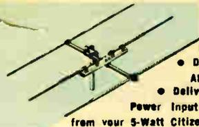
Unequaled point-to-point communications for Citizens Band operators. 9.3 db gain over dipole means the effective radiated power is multiplied by 8. This means your 5 watt Citizen's Band Transmitter can actually achieve a legal effective power input of 40 watts. Boom is 12' long with maximum turning ratio of 9.5 ft. Requires 1 1/4" mast and RG-8/U or R9-58/U Cable. Lugs are supplied for the other end. Shpg. wt., 30 lbs. AN-57WX Net 36.75
