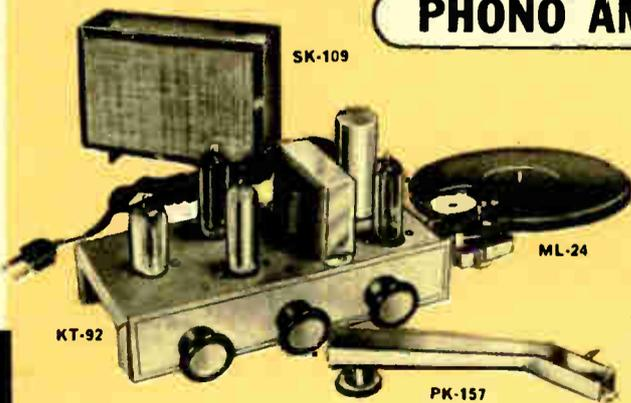
Everything required for a complete Hi-Fi system in this "easy-to-assemble" package—and Lafayette brings it to you at an unbeatable price. The system is centered about the excellent Lafayette KT-92 5 watt amplifier kit (as described above). The ML-24 4 speed turntable employs a rubber shock-mounted friction drive motor for quiet dependable operation. Tone arm is the Lafayette PK-157 containing turnover crystal cartridge with dual sapphire
