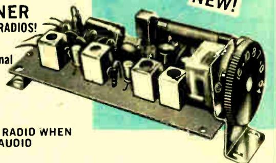
A deluxe 3 transistor subminiature AM broadcast tuner that features 3 dependable transistors, 3 IF plus 1 oscillator transformer, and ferrite antenna in a super efficient, completely wired superheterodyne circuit on a sturdy printed-circuit board.
