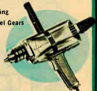
An outstanding value featuring a universal series wound motor that won't burn out. Top handle and 2-position rear handle are removable. Top quality construction with precision hobbled steel gears. 1/2" capacity in steel, 2" in wood. No-load speed 600 rpm; full load 400 rpm. AC-DC momentary contact switch with locking pin; special alloy self-oiling bronze bearings. Lustrous hi-polish finish with rich black crackle trim. Overall length 14 1/2". Shpg. wt., 12 lbs. Net 21.33 HO-999
