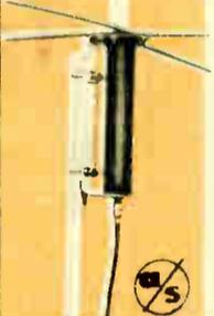
Compact vertical radiator with an actual 6 DB gain over any single element omni-directional antenna. Constructed of rigid aluminum and cadmium plated steel, it is corrosion resistant, waterproof and fits on most masts or directly into wooden areas. Hi-Q phasing transformer provides proper resonance over entire CB band. Direct ground lightning protection. 50 ohm feed. Total height is only 18" 2", (17" 3" radiator, 4-54" radials. Shpg. wt., 12 lbs. HE-487WX
