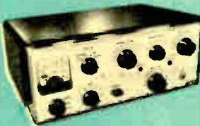
Brand new 90 watt band switching rig for 80 through 10 meters. Features a 6146 Final amplifier for 90 watts CW input, up to 65 watts phone with external modulation. 6AQ5 clamper tube protects final in case of loss of excitation. Variable pitch Pi-net output matches 50-100 ohm loads. Oscillator keying permits full break-in operation. Panel meter indicates exact operating currents and helps in tuning up. Its "novice limit" calibration safeguards the novice against exceeding the 75 watt power
