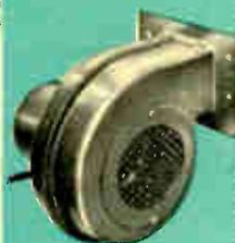
Efficient, quiet, dependable and economical. Usable in many applications—air distribution in confined areas, exhaust fumes and gas, etc. Suitable for ventilation equipment in home, marine and commercial use. Welded pressed steel housing. Shaded-type motor for efficient, quiet operation. Moves 200 cubic feet of air per minute. Mounting flange, 5 1/4"x4", 2-ft. AC line cord and plug. 110V, 60 cycles; 1.4 amp. SP-279 Shpg. wt., 7 lbs. Net 9.95
