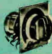
New L pads for use as "brilliance" controls to vary tweeter level, or as "presence" controls to vary mid-range speaker level. Both wirewound elements are concentrically mounted within one plastic housing. With gold-finished metal escutcheon plate, mtg screws, and attractive black knob. Size: 1 3/4" dia., 7/8" deep (less shaft), 2 1/2" deep overall. Shpg. wt., 6 oz.
