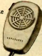
Features a high impact styrol case, hang-up clip and flexible single conductor shielded cable. Omnidirectional pattern mike has output impedance of 300 ohms and output level of -73 db at 1000 Hz. Grey and black case, with push-to-talk switch. Imported. Shpg. wt., 1 lb.
