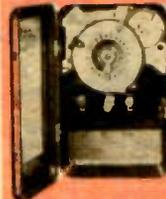
Turns equipment "on" and "off" once in 24 hours, or from 1-12 "on" and "off" operations a day can be obtained by use of extra trippers—can be added without removing dial. Min. on or off time 1 hr., max. 23 hours. Can be turned on or off manually with reset SPST switch rated at 40 amps. 4375 watt capacity. Mounting holes and knockouts. Gray steel case. UL Listed. Operates on 110 volt 60 Hz AC. 7 3/4 Lx5Wx3" D. Shpg. wt., 4 lbs.
