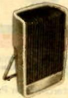
An outstanding Lafayette microphone for home use. Frequency response: 100-10,000 Hz  $\pm$ 10 db. Output level: -57 db at 1000 Hz. Impedance: 50,000 ohms. Complete with 5' shielded cable. Size 2"W x 3"H x 7 $\frac{1}{2}$ "D. Imported. Shpg. wt., 8 oz.
