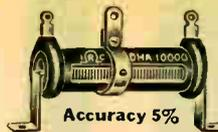
For all industrial and Radio uses. Dissipate heat rapidly, withstand heavy overloads, have great mechanical strength. All (except 10 watt units) are supplied with a NEW highly improved contact band that has a stainless steel spring spot-welded to it. The spring carries a silver contact button on which the pressure never varies—no torn resistance wire, no corroded contacts. Band is threaded. Mounting brackets with all but the 10 watt units.
