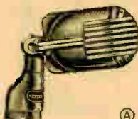
**(A) Model 708-A.** Stratoliner for good reproduction of voice and music. Genuine Bimorph crystal. Frequency response 60-8000 cps. free from undesirable peaks. High output of -53 db. Tilting head for directional or non-directional use. Pearl Gray finish. With 7 ft. cable. Hi-impedance.
