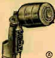
**(A) Model 630.** Moving coil dynamic. Acoustalloy diaphragm. High quality reproduction of speech and music, indoors and outdoors. Flat frequency response from 40-9000 cps. Output -53 db. Tilting head for directional or non-directional use. Built-in cable connector and switch. Complete with 20 ft. cable. Shpg. wt. 5 lbs. Hi-impedance.
