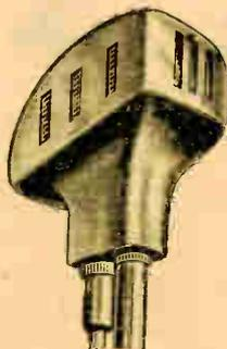
**Studio Ribbon Microphone,** for broadcasting, recording, and public address. Will not become "boomy" on close talking. Pickup angle 120° at front and back with practically no frequency discrimination. Ruggedly constructed for indoor or outdoor use. Not affected by wind. Frequency response from 40-14,000 cps. Output -56 db. Chrome finish. Complete with switch, 25 ft. cable and connectors. Shpg. wt. 8 lbs.
