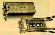
Standard iron core 455 kc. midgets. Compression tuned, exceptionally high gain due to specially designed powdered iron cores. For general replacement and new set construction of small receivers and portables. Dimensions of can 3/4" square by 1 7/8" long.
