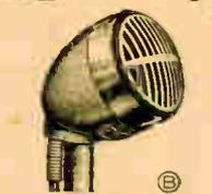
**(B) Model 707-A.** Mechanically isolated moisture proofed Bimorph crystal. For amateur phone transmitters, public address and call systems. Frequency response suitable for voice and music reproduction. Output -53 db. Pearl Gray finish. Hi-impedance. With 7 ft. cable.
