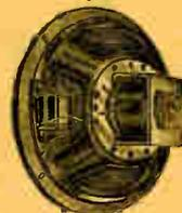
5" dynamic speaker for general replacement in radio receivers, call and intercommunication systems. Also used for light public address work. When properly baffled has a practically flat response covering from 100 to 4500 c.p.s. Formed one piece cones. 3000 ohm field. Less transformer. Shpg. wt., 3 lbs. **\$1.59**
