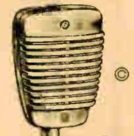
**Model 52 "Econodyne"** sturdy dynamic microphone that offers quality performance at low cost. Frequency response from 60-8000 cps. Output -52 db. With 15 ft. cable. Hi-impedance. Similar in appearance to Model 707-A.
