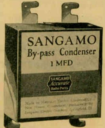
Meets the need for a durable condenser that is mechanically strong and capable of standing heavy electrical surges without breakdown. Tightly wound with high-grade aluminum foil and special insulation on patent-protected machines. This process eliminates varying tension with consequent air and ozone bubbles, which cause a variation in surface contact and therefore a fluctuating capacity.
