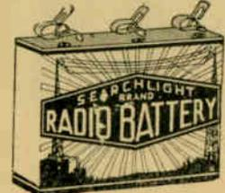
No. 3-C—The purpose and uses of this battery are three-fold. It may be used as an "A" (Filament) battery or serve as a "B" (plate) battery. It is, however, primarily designed to act as a "C" (grid biasing battery).
