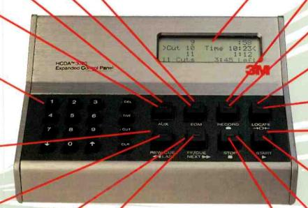
**Display** This 4-line x 20- character LED display provides feedback on Kevpad instructions. cut number, track information, time, signal status (EOM & AUX), error status, and overlevel conditions
