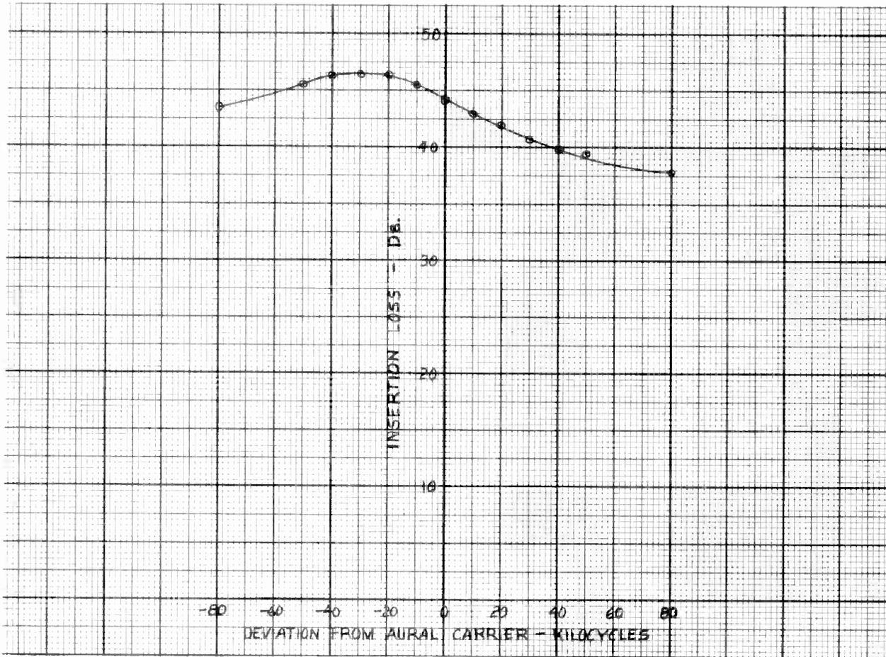
Figure 4. Isolation of Visual Channel from Aural Channel
