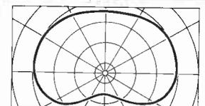
Similar to the Type 1040 Slotted-ring Antenna, but with pattern shaping members connected to alternate active rings, the Type 1030 provides a controlled pattern adjustable to service requirements. Pattern and antenna shown are of **WEAT-TV, Channel 12, West Palm Beach, Florida.**
