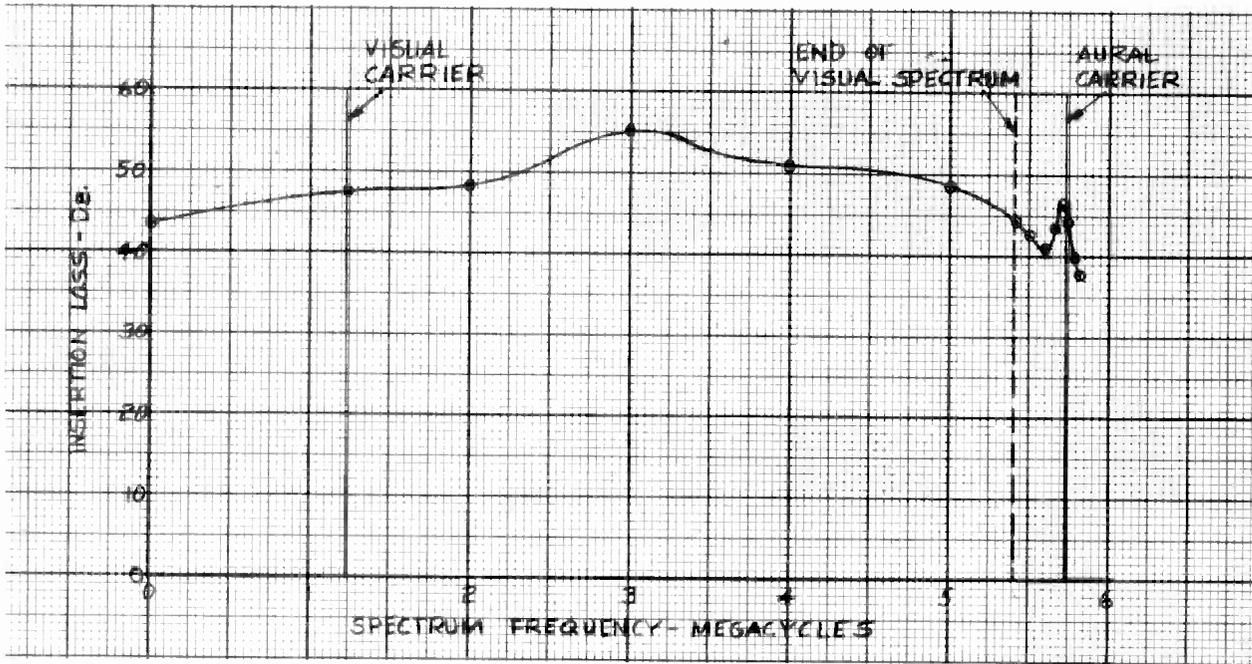
Figure 3. Isolation of Aural Channel from Visual Channel
