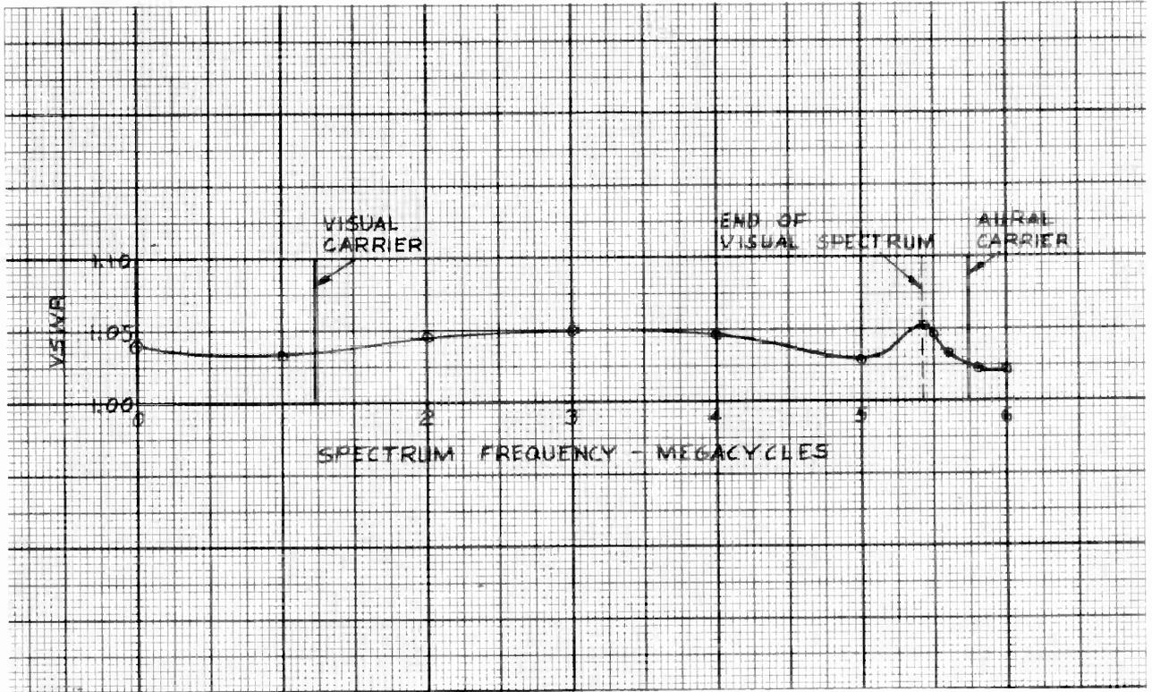
Figure 1. Visual Channel Input Voltage Standing Wave Ratio
