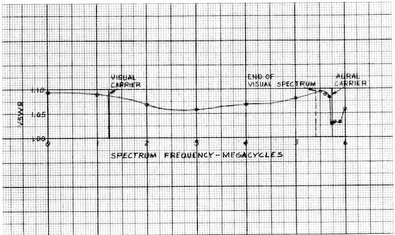
Figure 2. Aural Channel Input Voltage Standing Wave Ratio
