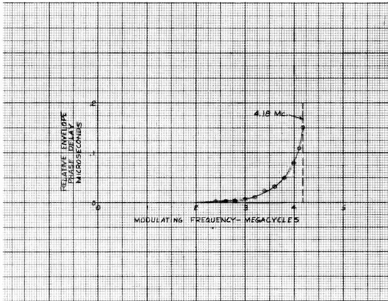
Figure 7. Relative Envelope Phase Delay Introduced into the Visual Channel
