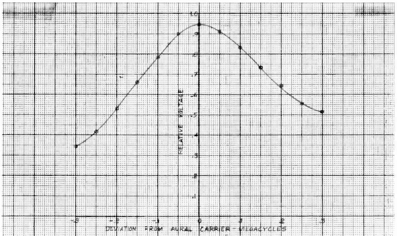
Figure 6. Aural Channel Amplitude Response
