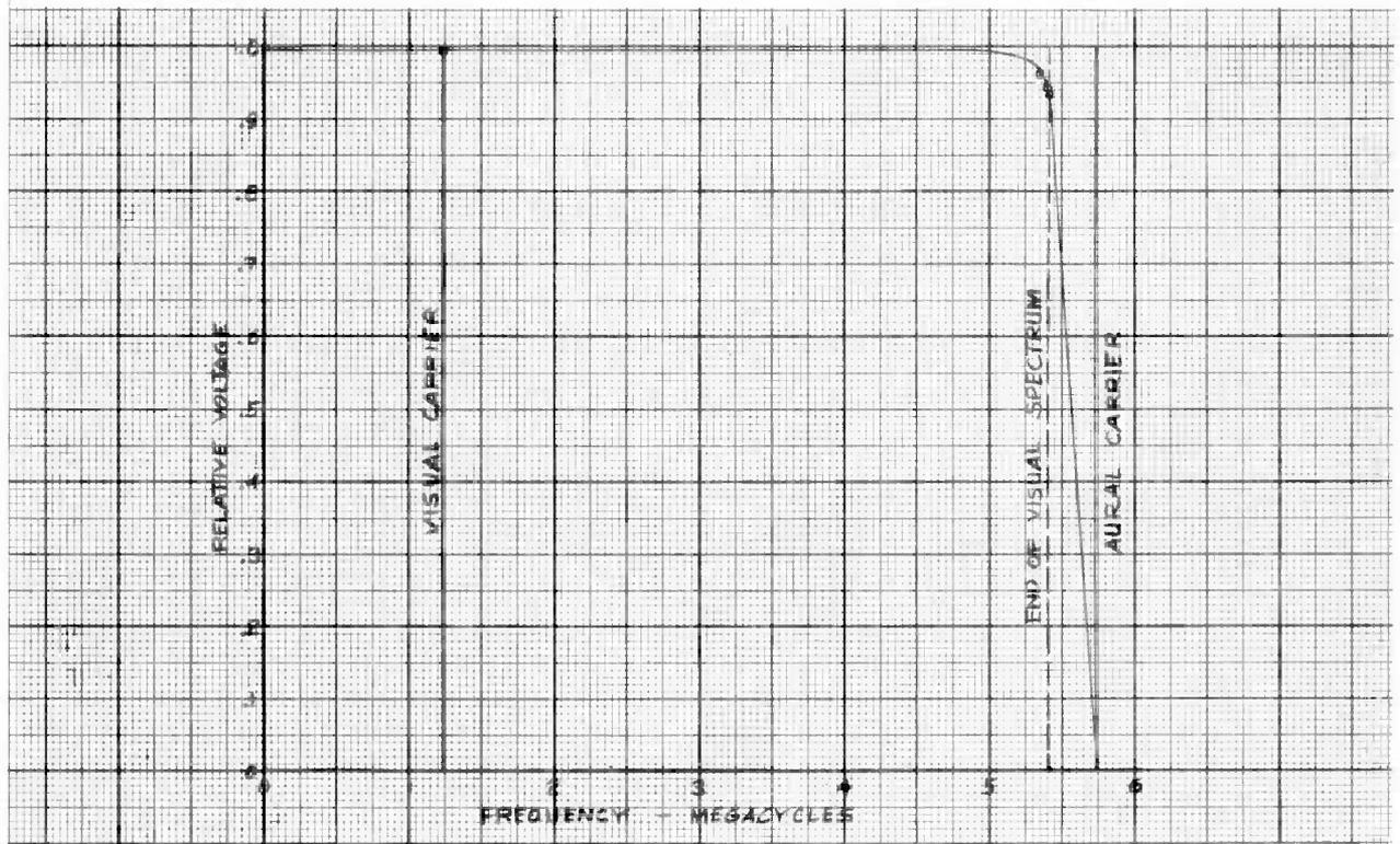
Figure 5. Visual Channel Amplitude Response
