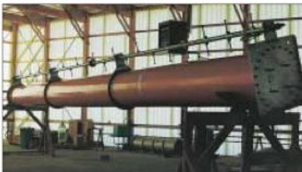
GUIDELINER antenna for WTU channel 30 undergoing inspection.
