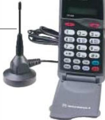
Innovative adapter allows easy connection to both the external antenna and rubber spike antenna.
