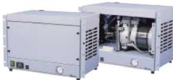
The **MT300 series** automatic membrane dehydrators are equipped with the unique Andrew uni-mount system allowing for rack, wall or free-standing mounting without additional parts. They are designed to supply dry air at a dewpoint of -45°C (-50°F), or better, under the ambient conditions of 95% RH at 49°C (120°F).
