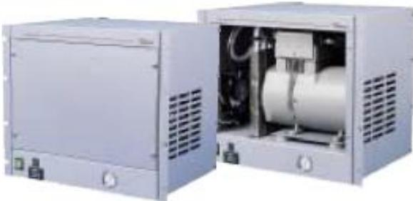
The **MT-600** series automatic membrane dehydrators are designed to provide the same features and benefits to large microwave and broadcast applications as the smaller MT300. They are equipped with the unique Andrew uni-mount system allowing for rack, wall or free-standing mounting without additional parts and are designed to supply dry air at a dewpoint of -45°C (-50°F), or better, under the ambient conditions of 95% RH at 49°C (120°F).
