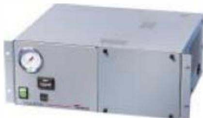
This small compact fully automatic membrane dehydrator is ideal for earth station, small microwave and cellular systems from 0.1 to 20 ft<sup>3</sup> (560 liters) in volume. It requires only 4 RUs, 7 in (178 mm) of space in a 19-inch rack and meets the new European N-3 standards for complete front access for installation and routine maintenance.
