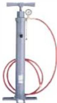
**Hand pumps** are lightweight portable air drying systems capable of pressurizing up to 30 lb/in<sup>2</sup> (210 kPa). Removal of moisture is accomplished by passing ambient air through a cylinder of color indicating silica gel desiccant. The pump contains a sight glass to view the moisture condition of the desiccant. When the dark blue color changes to amber, it is time to replace or regenerate the desiccant. Do not use the pump after the desiccant turns amber.
