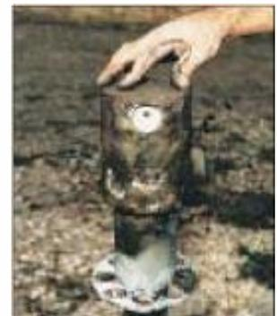
Burned PTFE shows the conductive path formed by dust-laden moisture. As the path arcs over, the transmission line fails.
