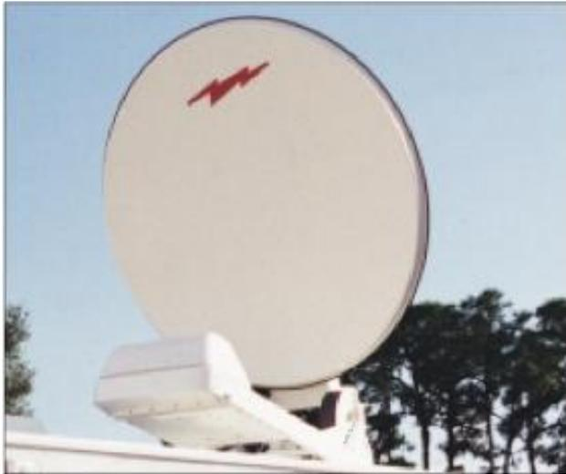
2.4-Meter Transportable SNG Antenna
