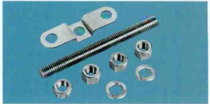
**Threaded Rod Support Kit** of 5 pieces. 1/2" x 12" (305 mm) threaded rods, ceiling mounting plates, nuts and washers for suspending 5" cable hangers. All parts are stainless steel except galvanized ceiling mounting plate .....Type **31771-5**
