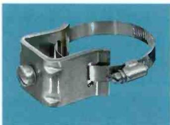
**Round Member Adapter/Tower Standoff Kit** of 10 pieces. For mounting 5" cable hangers to round support members. HELIAX cable to clear tower leg flanges. Provides 2.5 in (60 mm) standoff. All parts are stainless steel or galvanized.
