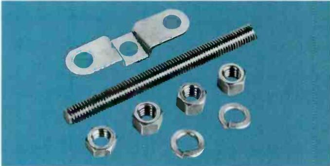
**Threaded Rod Support Kit.** Use to mount hangers away from supporting structure, under cable bridge and inside equipment room. Includes 3/8" diameter threaded rod, galvanized ceiling mounting plate, nuts and washers. Attach to angle tower members with 31768A angle adapters. Attach to round tower members with 30848 series tower standoffs. All components are stainless steel, except ceiling mounting plate.
