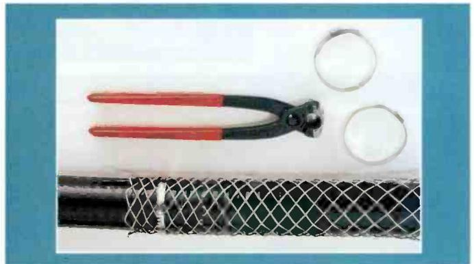
**Support/Hoisting Grip.** Use at 200 ft (60 m) intervals to raise cable and provide permanent cable support. Basic kit includes one grip and one support clamp. Support clamps are also available in kits of 10. Installation tool is required. The tool includes a kit of 10 support clamps.
