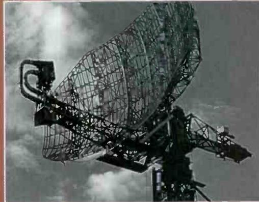
L-band Primary Surveillance Air Traffic Control Radar
