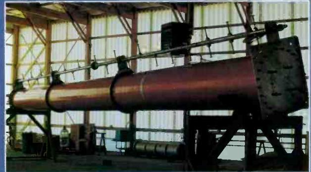
GLIDELINER antenna for WTU channel 30 undergoing inspection.
