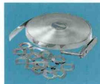
**Stainless Steel Wraplock** 100 feet complete with fasteners. Use to attach 1/4" - 7/8" insulated hangers to round members. Not to be used to attach cable or waveguide directly to towers.....Type **12395-1**
