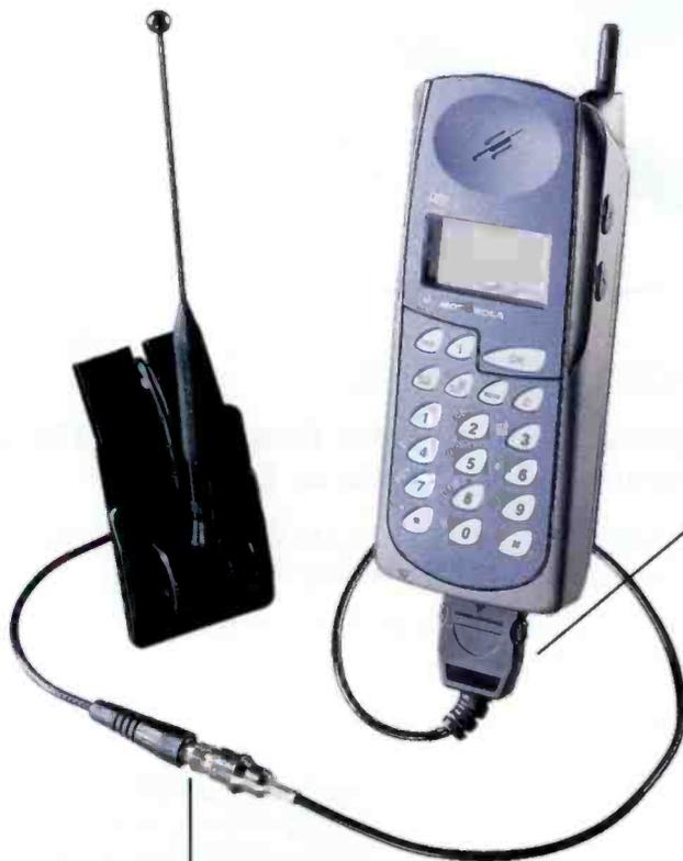
ACC adapter allows easy connection to window, glass, magnet and roof mounted antennas.
