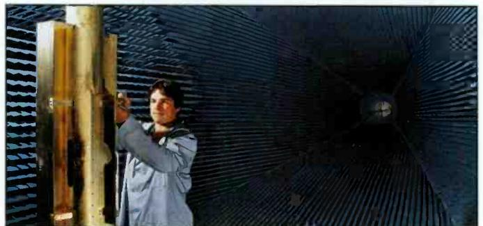
Full Size antenna section undergoing azimuth pattern test in one of two Andrew anechoic chambers dedicated to broadcast products.
