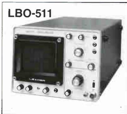
The LBO-511 is an economical, general-purpose oscilloscope. Ideal for basic electronics courses, it is also widely used in industry and for TV servicing. Features include: a 9-step calibrated vertical input, 10 Hz to 100 KHz sweep frequencies (plus TV-H and TV-V), 2-axis, internal calibration signal, and inputs for color TV vector display.
