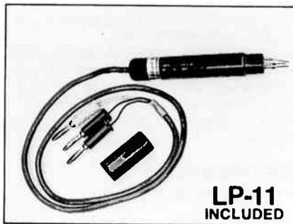
The LP-11 Three-Point Probe permits convenient, one-handed connection to transistors installed on printed circuit boards. The probe is equipped with three flexible, spring loaded, pointed tips which are easily manipulated for simultaneous connection transistor leads.
