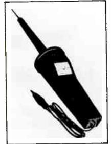
The LHM-80A permits easy and safe measurement of voltages up to 40,000 Vdc. It is widely used for checking CRT accelerating voltages, testing and servicing X-ray machines, and other high voltage equipment. Completely self-contained (no batteries or external power required), it is made of high-impact polystyrene with a special corona safety shield. Full-scale accuracy is  $\pm$  3%. It is supplied with ground wire and heavy-duty cap.
