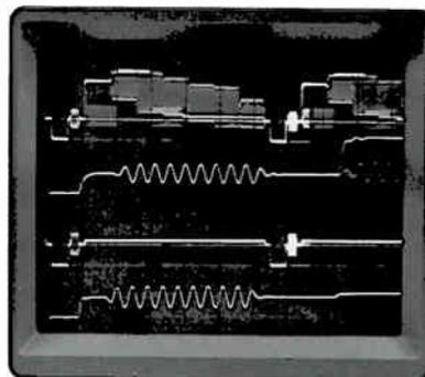
The alternate time-base mode permits viewing the main and delayed time bases for both channels simultaneously. The main time-base is shown with the delayed time-base portion intensified.
