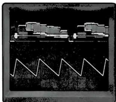
Alternate triggering permits a stable display of two asynchronous signals.
