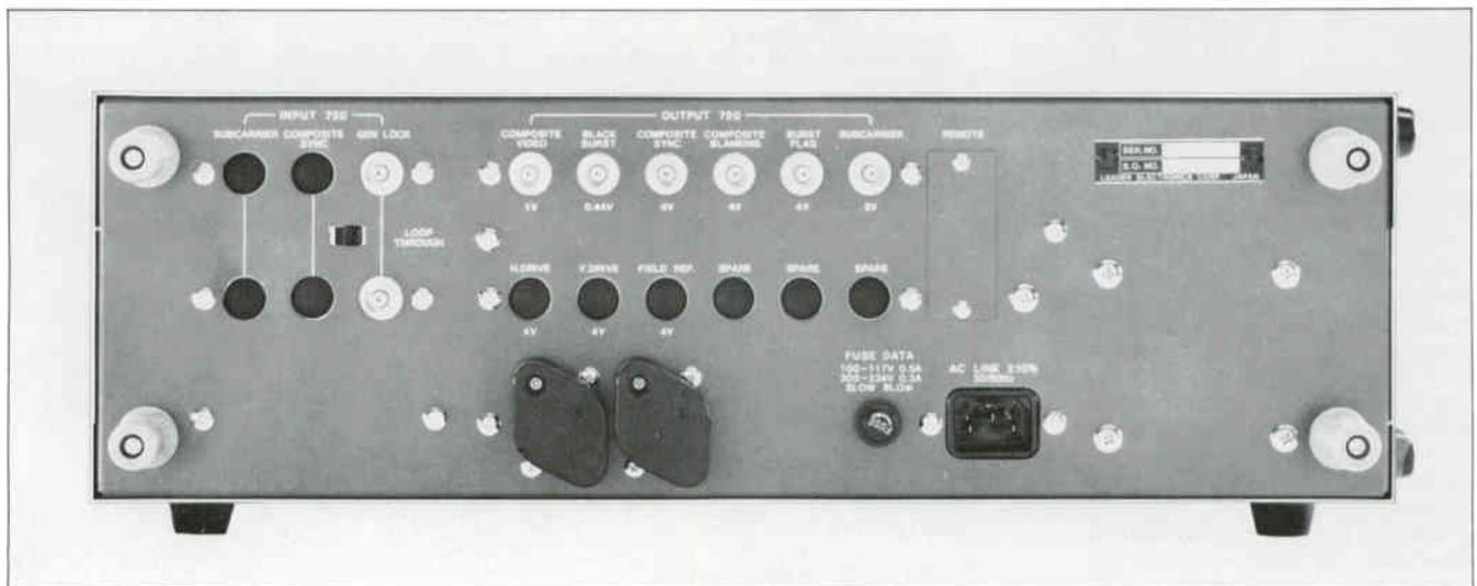
The LCG-400 provides both gen-lock and internal synchronization with the full range of video signals needed for testing and adjusting monitors, cameras, VTR's and overall performances of color and B&W TV systems. It is available with either multiburst (LCG-400M) or sweep-marker (LCG-400S) generators. The LCG-400 will sync with all standard composite video signals including those from quad head and helical scan VTR's.
