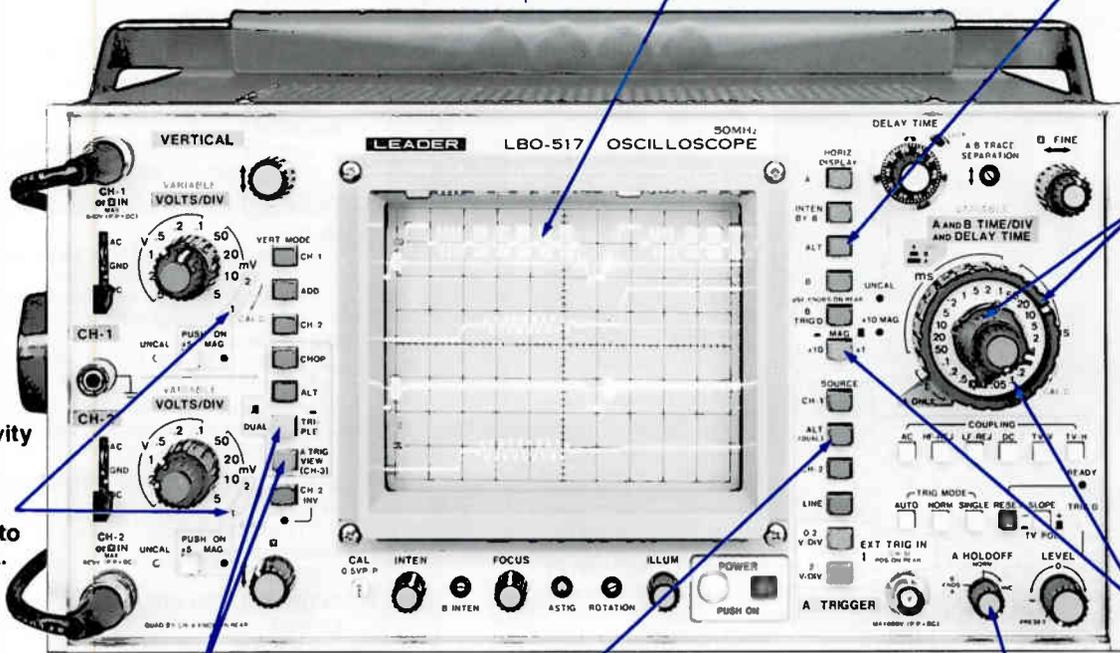
Third and fourth channel trigger view permits observing both the main and delayed time-base trigger wave forms. Channel 4 (input and position control on rear panel) may be used as an additional independent display channel when the delayed time-base is not triggered.
