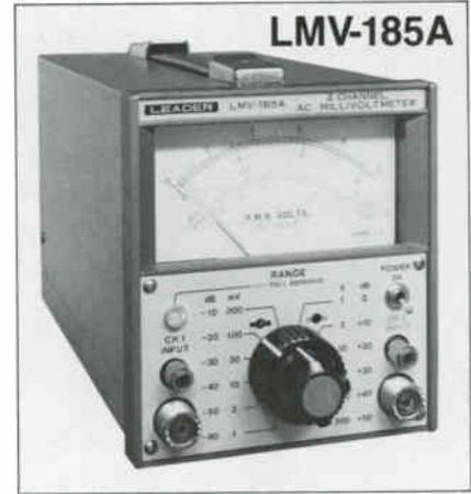
The LMV-181A and LMV-185A are general purpose average responding ac voltmeters with a measurement range of 100  $\mu$ V to 300 V. The LMV-182A is an average responding ac voltmeter with increased sensitivity featuring an effective measurement range of 30  $\mu$ V to 100 V. Bandwidth is 5 Hz to 1 MHz permitting use in a broad range of applications including audio, IF and ultrasonic circuits and systems.
