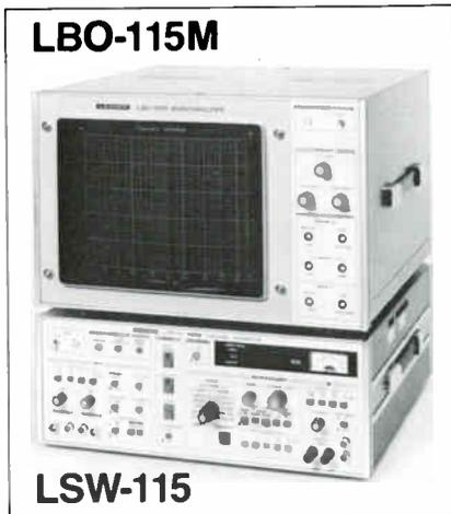
The LSW-115 is a 2-channel Audio Frequency Sweep Generator designed for use in observing the frequency response characteristics of a wide range of audio equipment and devices. It employs a digital waveform storage capability to provide stable displays at slow sweep rates. Response curves may be reproduced on an X-Y Recorder or on the Model LBO-115M CRT Display.
