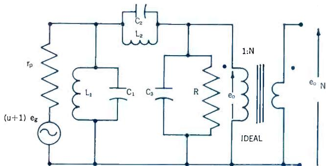
Figure 15 — Class A triode wide-band transformer stage network.
