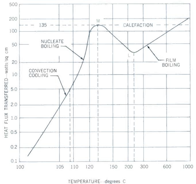
Figure 4 — Nukiyama Heat Transfer Curve For Boiling Water.
