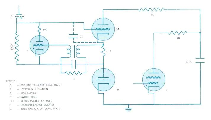
Figure 3 — Circuit showing a thyratron in a switch tube grid circuit. The switch tube is cut off when load tube arcs by firing the thyratron, T, by voltage developed across 0.1 ohm resistor.
