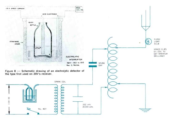
Figure 9 — Schematic drawing of the 3BV transmitter.
