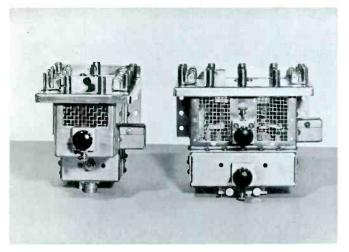
Figure 1 — Tuned line tripler stage (left), tuned line amplifier stage (right) of Translator Models HTU-100 and U-HTU-100.
