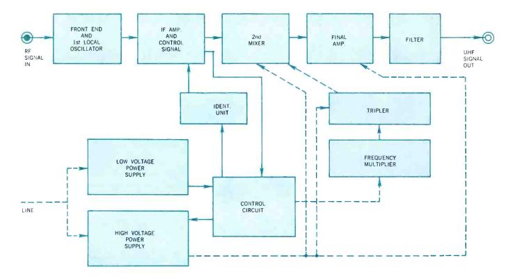
Figure 3 — Block diagram of HTU-100 Translator.
