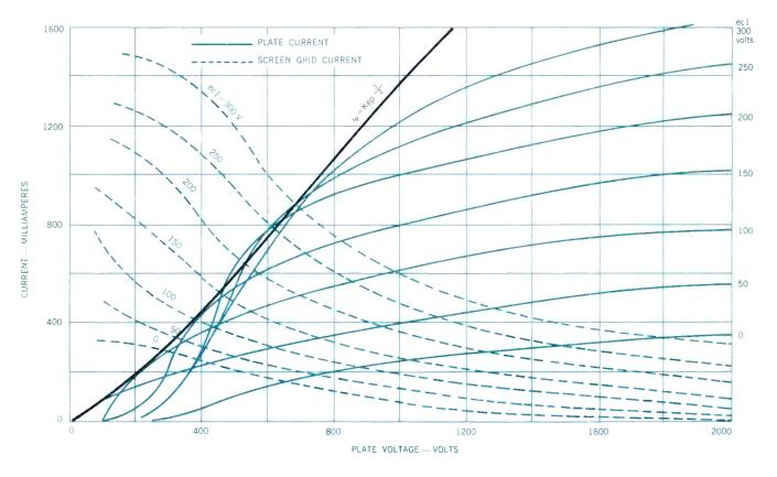
Figure 4 — Typical Constant Grid Voltage Characteristics. Line labelled  $i_{\rm p}$  = Kep^{3/2} shows plate current drawn from virtual cathode formed between screen grid and plate.
