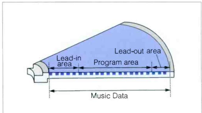
Fig. 8 Cross-sectional Representation of Disc Substrate
