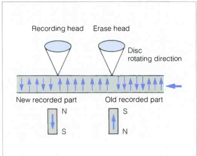
Fig. 20 Data Rewriting with One Laser in Two Rotations
