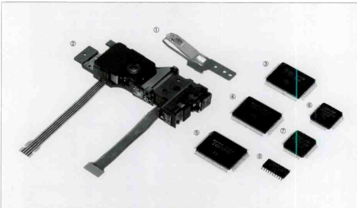
These specialized LSI and key components have been developed specifically for MiniDisc applications:
