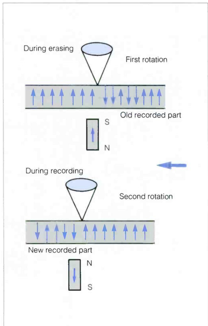
2. A single laser is used for these two tasks, with old data erased in the first rotation, and new data recorded in its place on a second rotation. (Fig. 20)
