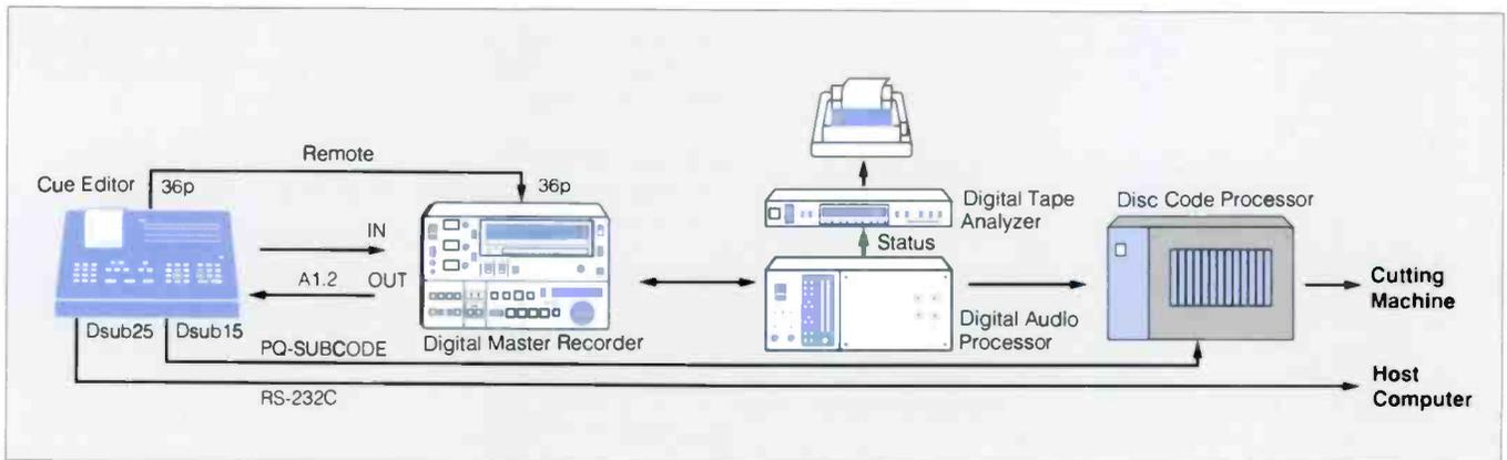
Fig. 28 MiniDisc Mastering System
