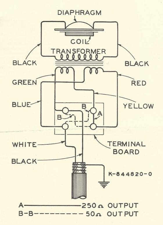
MICROPHONE CIRCUIT (Schematic K-844820)
