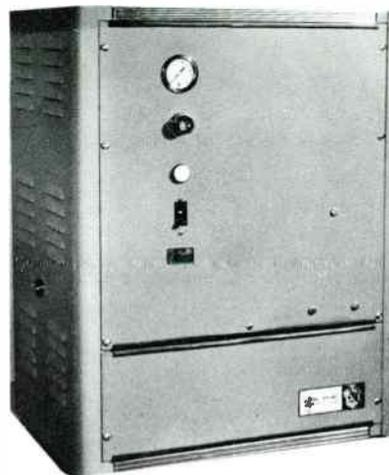
Engineered and manufactured specifically for pressurizing RF transmission lines, these two compressor/dehydrator units differ only in output capacity and physical dimensions. The units deliver dry, compressed air at the rate of one or two cubic feet per minute (0.028 or 0.056 m<sup>3</sup>).
