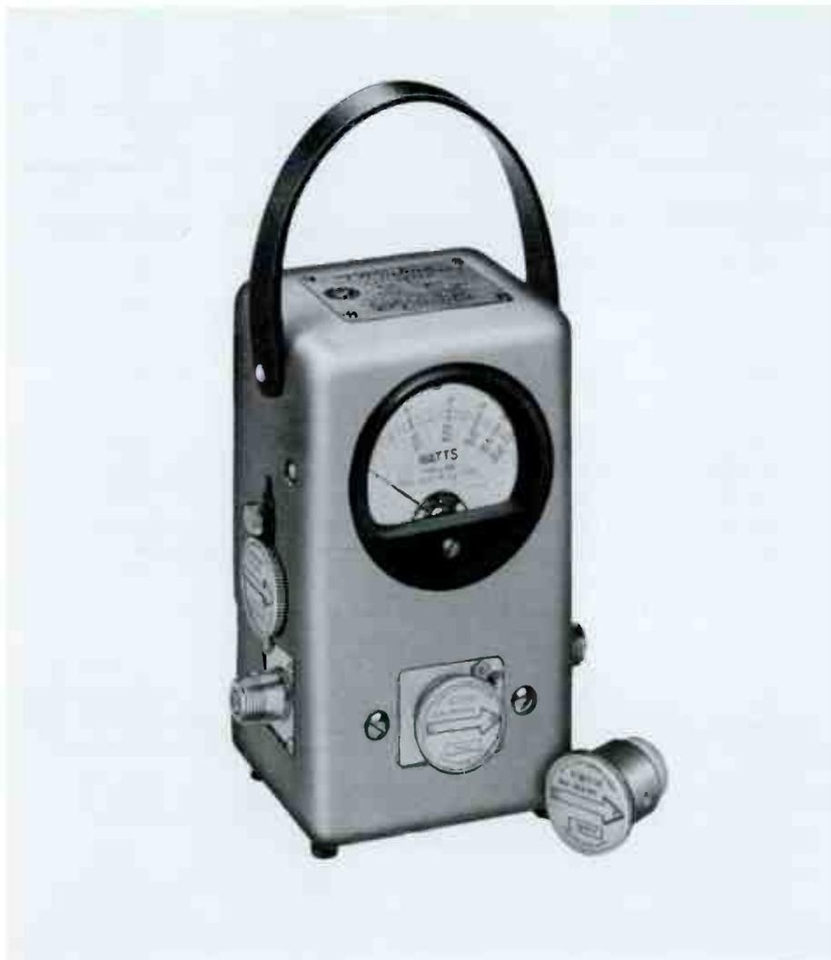
The loads and wattmeters described here are dual-purpose units. As non-inductive dummy loads, they aid in transmitter tune-up without radiation; as wattmeters, they terminate the transmitter output and indicate an accurate measure of power output.
