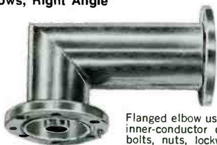
Flanged elbow uses swivel flanges and includes inner-conductor connector, O-ring gasket, six bolts, nuts, lockwashers. Unflanged elbow includes inner-conductor connector only.
