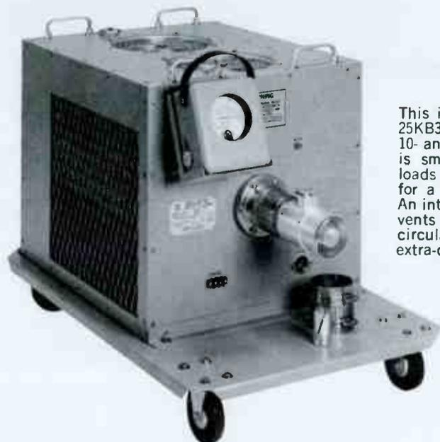
This is the 20 kW system (Bird 8644/4805/25KB3/5-726) and is representative of the 10- and 40-kW loads as well. The 10-kW load is smaller while the 40- is larger. These loads require a source of commercial power for a coolant pump within the enclosure. An interlock connection, properly used, prevents application of power without coolant circulation. Dolly shown is optional as an extra-cost accessory.
