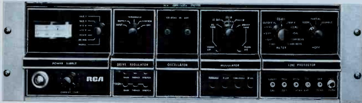
Exciter/modulator unit. Completely solid-state, this unit is used in all RCA Amphase transmitters. Available separately for use as a spare. See Accessories.
