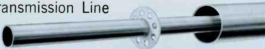
Unflanged line is a hard tempered copper transmission line designed for unpressurized indoor applications in AM and FM. It employs a low loss Teflon dielectric and operates with high efficiency. A complete line of components in 1 5/8-, 3 3/8- and 6 1/8-inch nominal diameters provides installation versatility for a wide power range.
