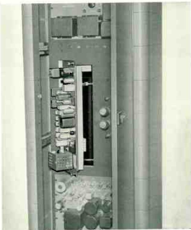
Hinged construction of the Exciter unit is a service and maintenance feature of new RCA STL equipment.
