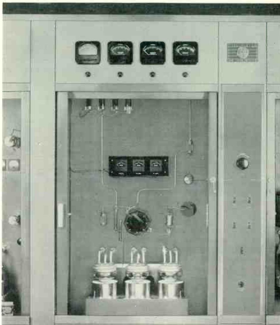
The Power Amplifier or r-f output stage consists of two RCA-5762\* Tubes, in the BTA-5H for 5-kw operation. A third RCA 5762 is added in the final of the BTA-10H for 10-kw operation.
