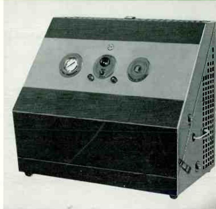
same time that air is being passed through the reactivating chamber during the last 1/2 hour of the 5 hour heating cycle. Solenoid valves also control the output of each chamber. These serve to switch the outputs either to the line or to the atmosphere for reactivation or line pressurization.
