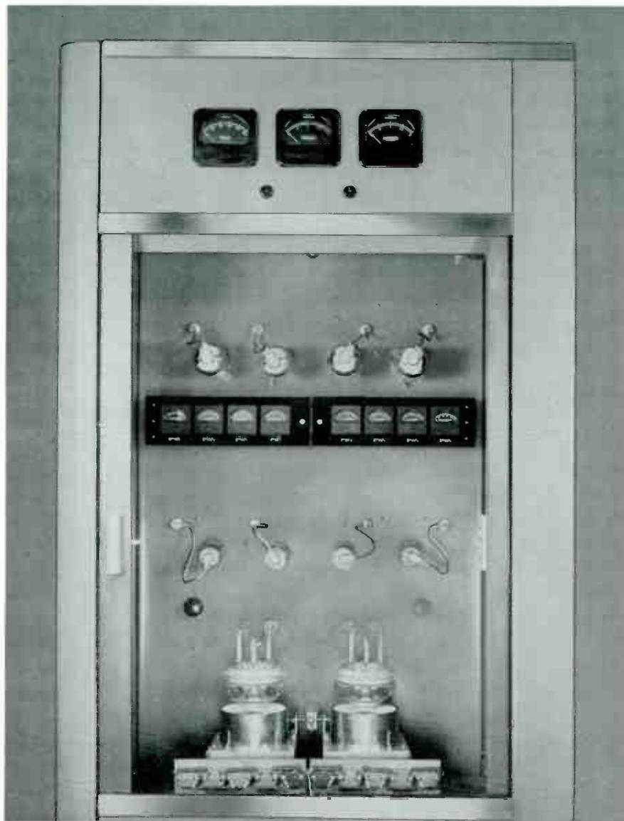
**Closeup View of the Audio and Modulator Cabinet showing the mechanical and electrical arrangement of major components. Long-life RCA 828's, 807's, 813's and RCA 5762's are employed in these stages. Bi-level modulation reduces distortion and increases fidelity to a new high in the BTA-5H.**
