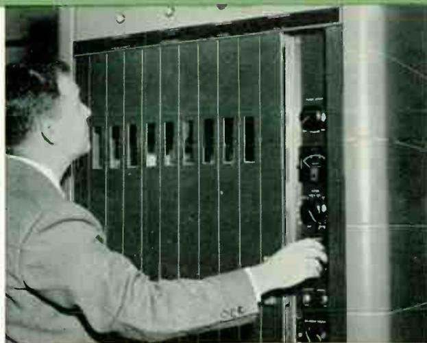
**SIMPLE TO OPERATE**—Only one tuning control—located on an easy-to-reach vertical control panel which is exposed by sliding front door to the left 4 inches.
