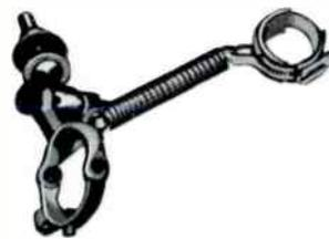
Spring hanger for single line. Requires mounting hole. Complete with clamps and pivot bolt to compensate for line misalignment. Spring must be preloaded at installation.
