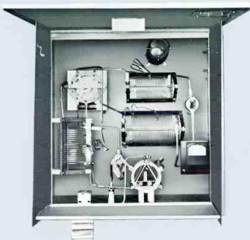
Line Terminating Unit installed in weatherproof cabinet.
