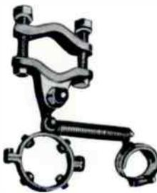
Spring hanger for single line. Complete with clamps and pivot bolt to compensate for line misalignment. Spring must be preloaded at installation.
