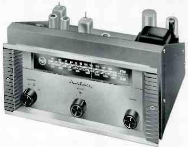
impedance range (10,000 or greater) still realizing the excellent frequency response and low distortion the receiver is capable of producing. All controls are conveniently located on the front panel. The large, legible, slide-rule type dial is edge lighted. The unit is equipped with power cord and plug.
