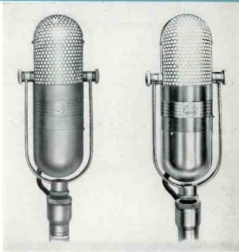
ment by positioning of a shutter to secure various areas of opening. The moving element is a thin corrugated metallic ribbon clamped at the ends and suspended in the air gap of a magnetic circuit consisting of an Alnico V permanent magnet and pole pieces. One side of the ribbon is open and the other is connected by means of a tube to a folded acoustically damped pipe contained in the center section of the microphone.
