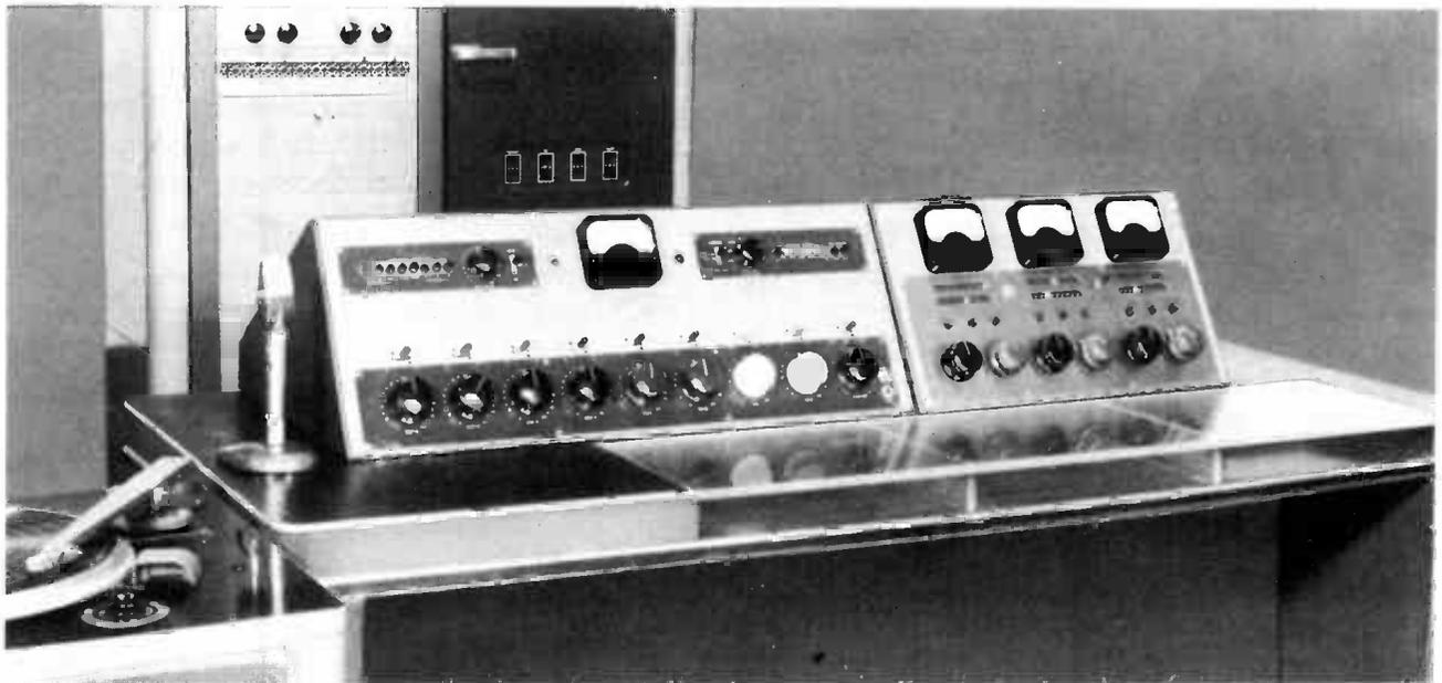
Figure 3 - Studio Console Type BC-2B with Master Switching Console Type BCS-11A
