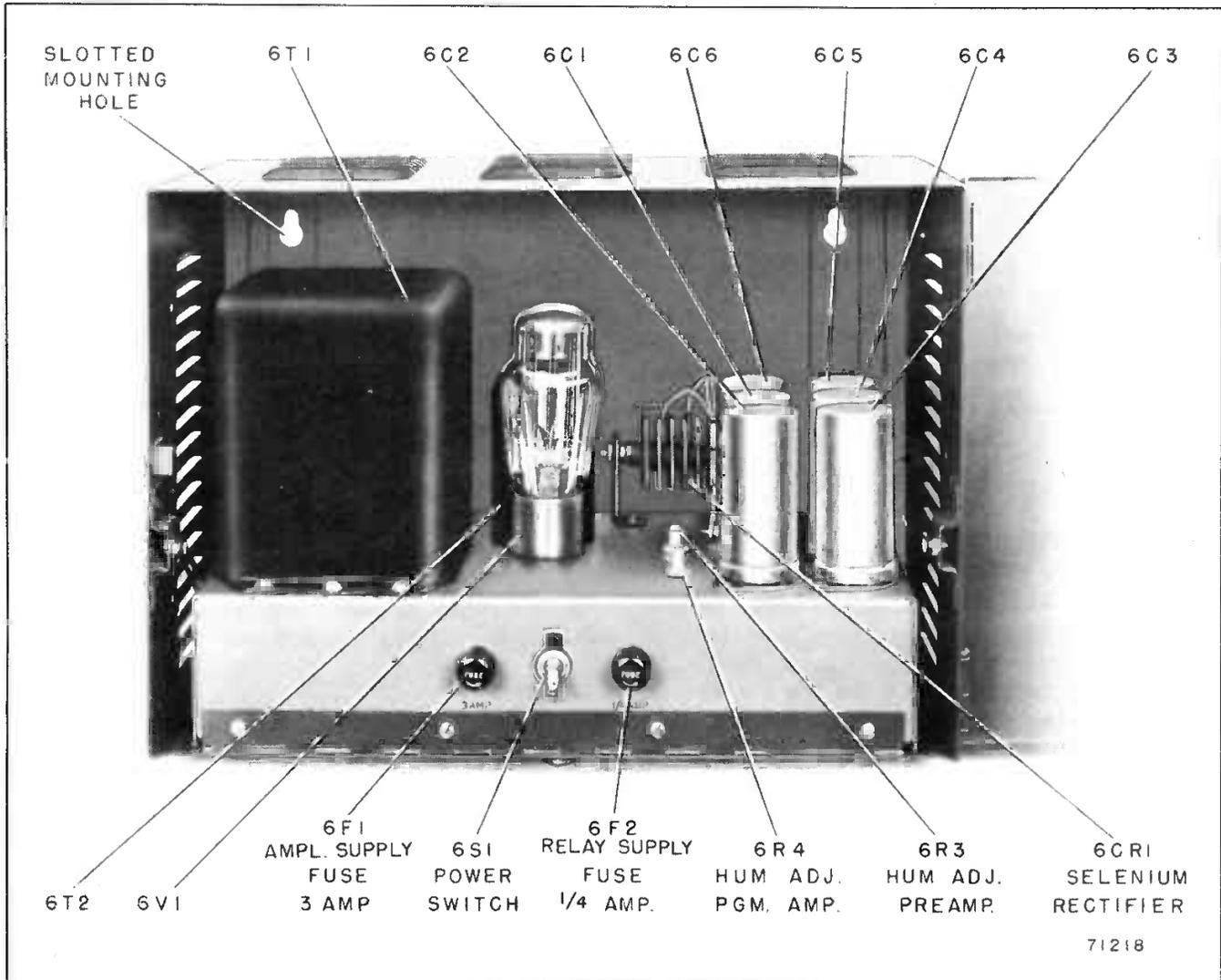
Figure 2 - Power Supply Chassis Mounted in Cabinet
