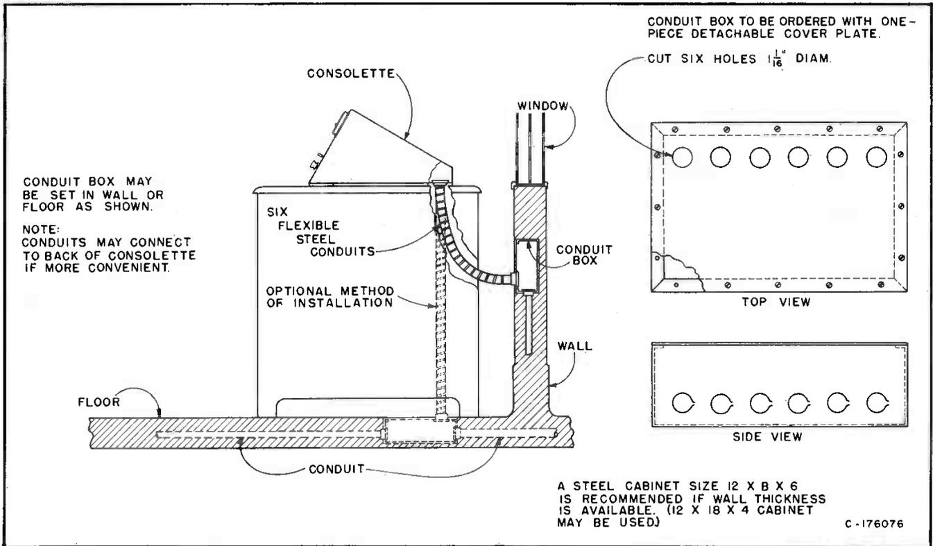
Figure 13 - Typical Installation Showing Relation of Cabinet and Conduit Box
