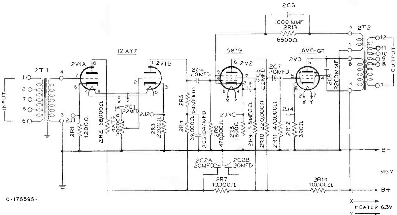
Figure 6 - Schematic for Program Amplifier
