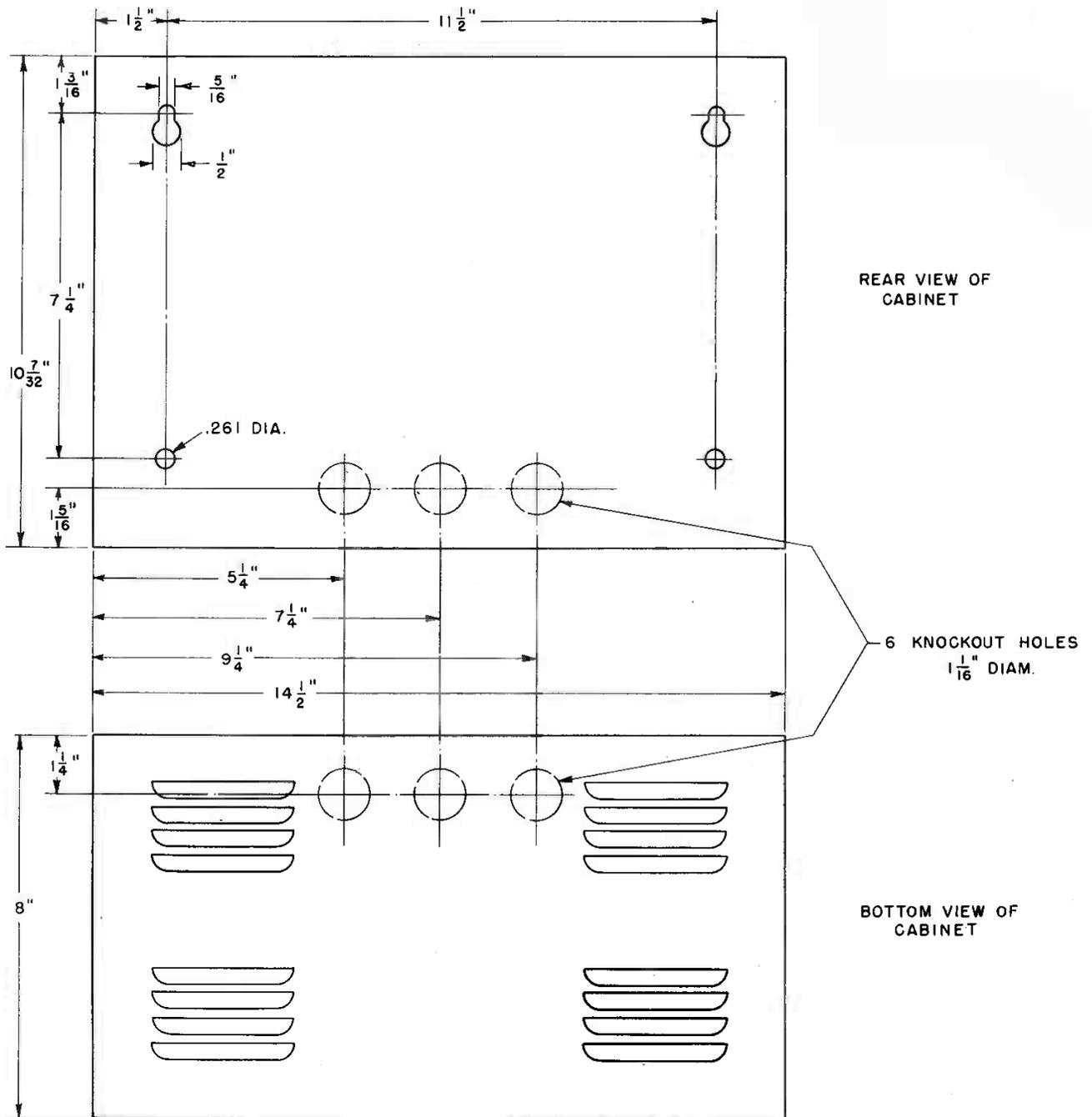
Figure 3 - Dimensional Drawing for Mounting Power Unit
