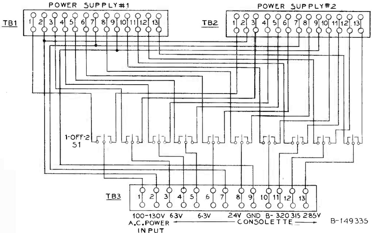
Figure 5 - Schematic for Power Transformer Switch
