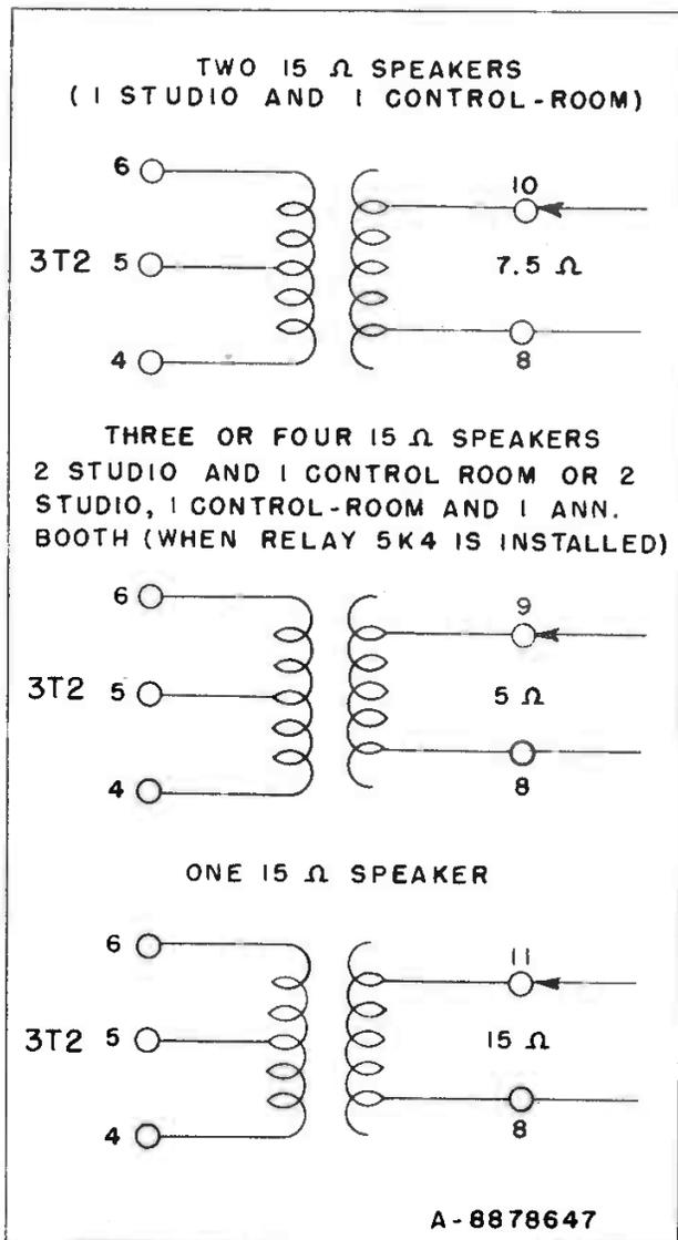
Figure 16 - Output Transformer Connections
