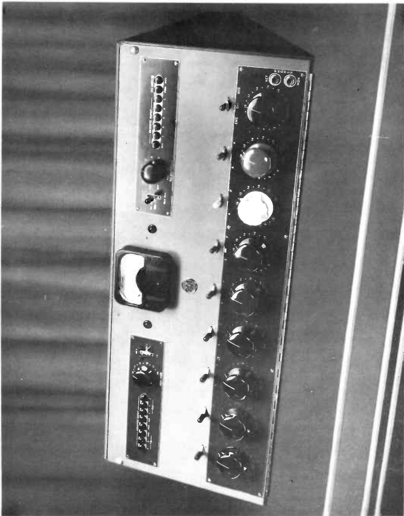
Figure 1 - Studio Consolette Type BC-2B (Signal Lights Added)
