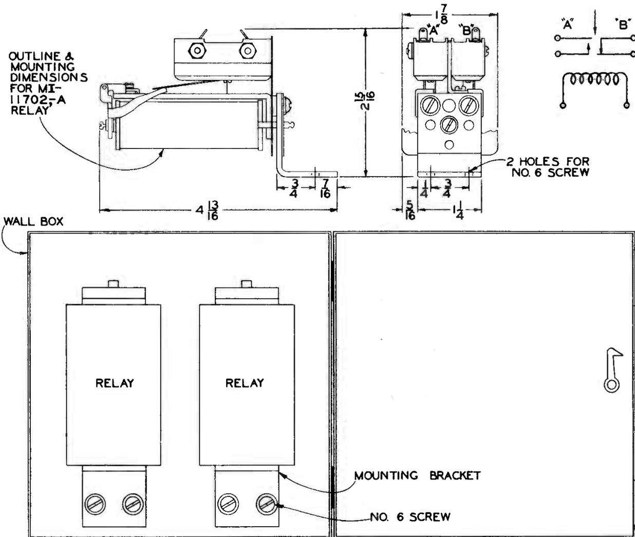
TWO MI-11702;A RELAYS MOUNTED IN A 6X6X4 STEEL CABINET.
