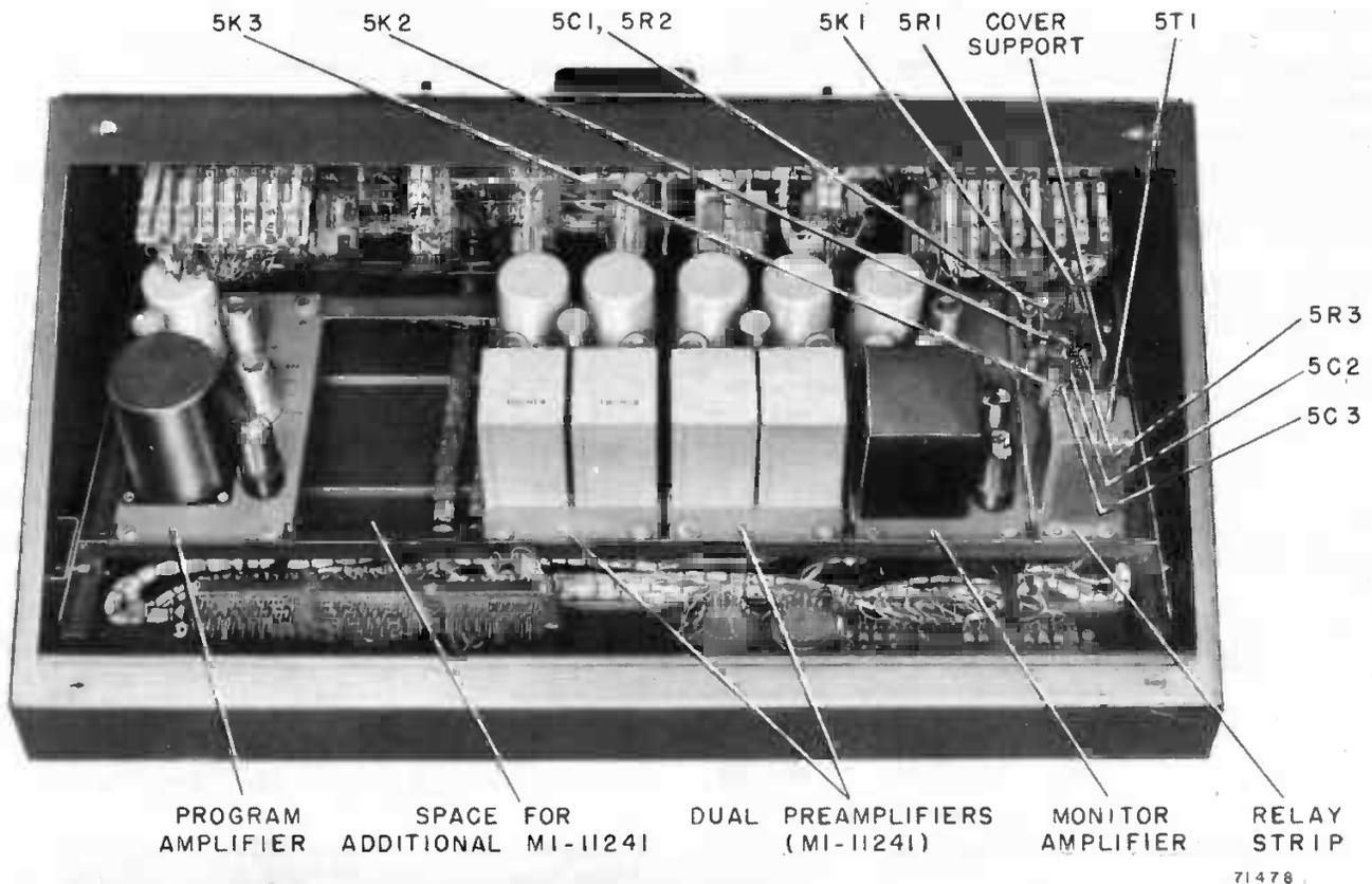
Figure 15 - Rear View, Consolette and Relay Covers Removed
