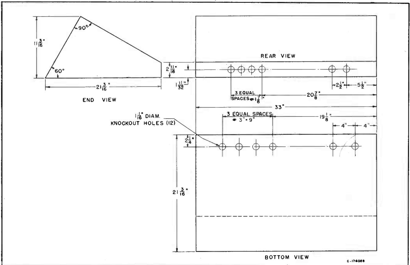
Figure 14 - Dimensional Layout of Consolette
