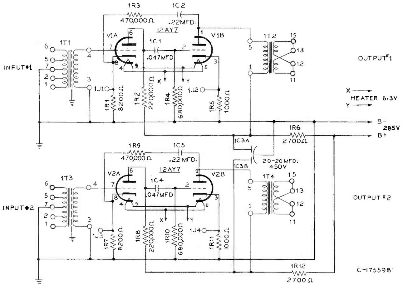
Figure 4 - Schematic for Dual Pre-amplifier MI-11241
