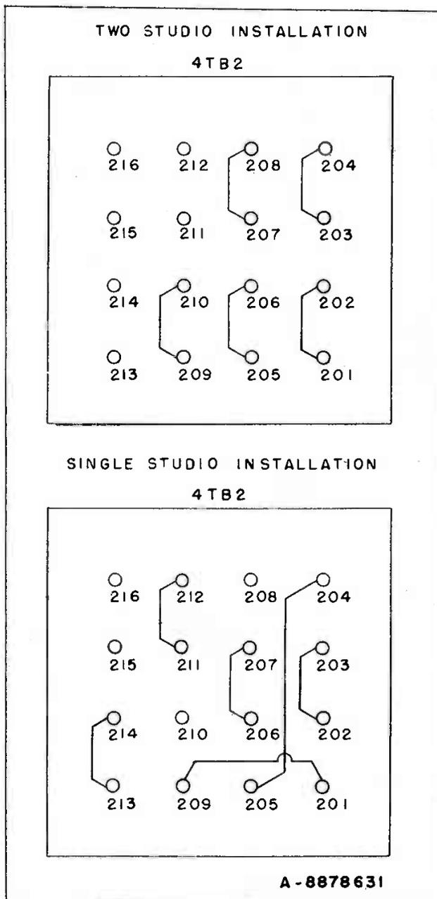
Figure 11 - Terminal Board Connections for Single and Two-Studio Operations
