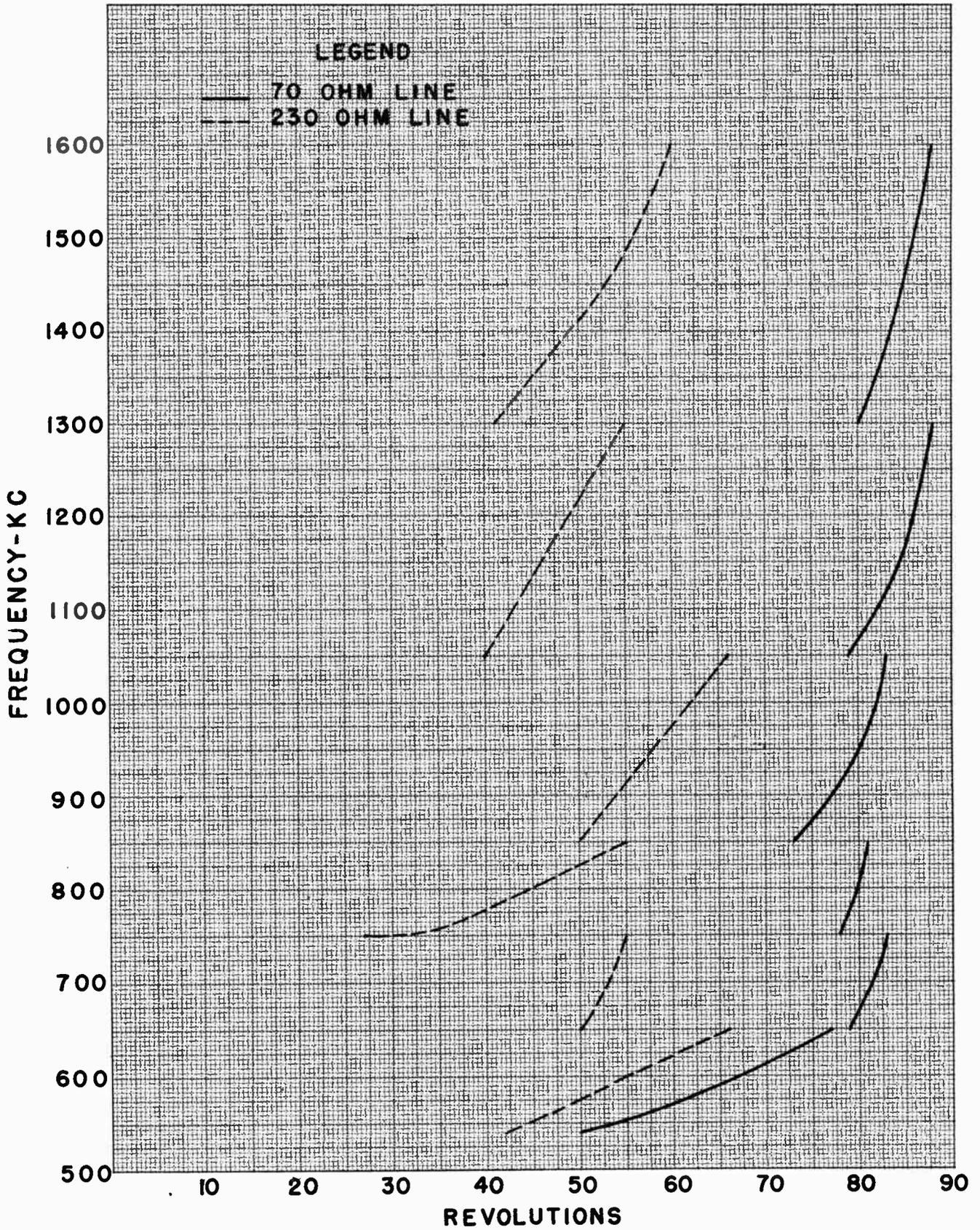
Figure 13—Antenna "LOADING" Dial (L10)
