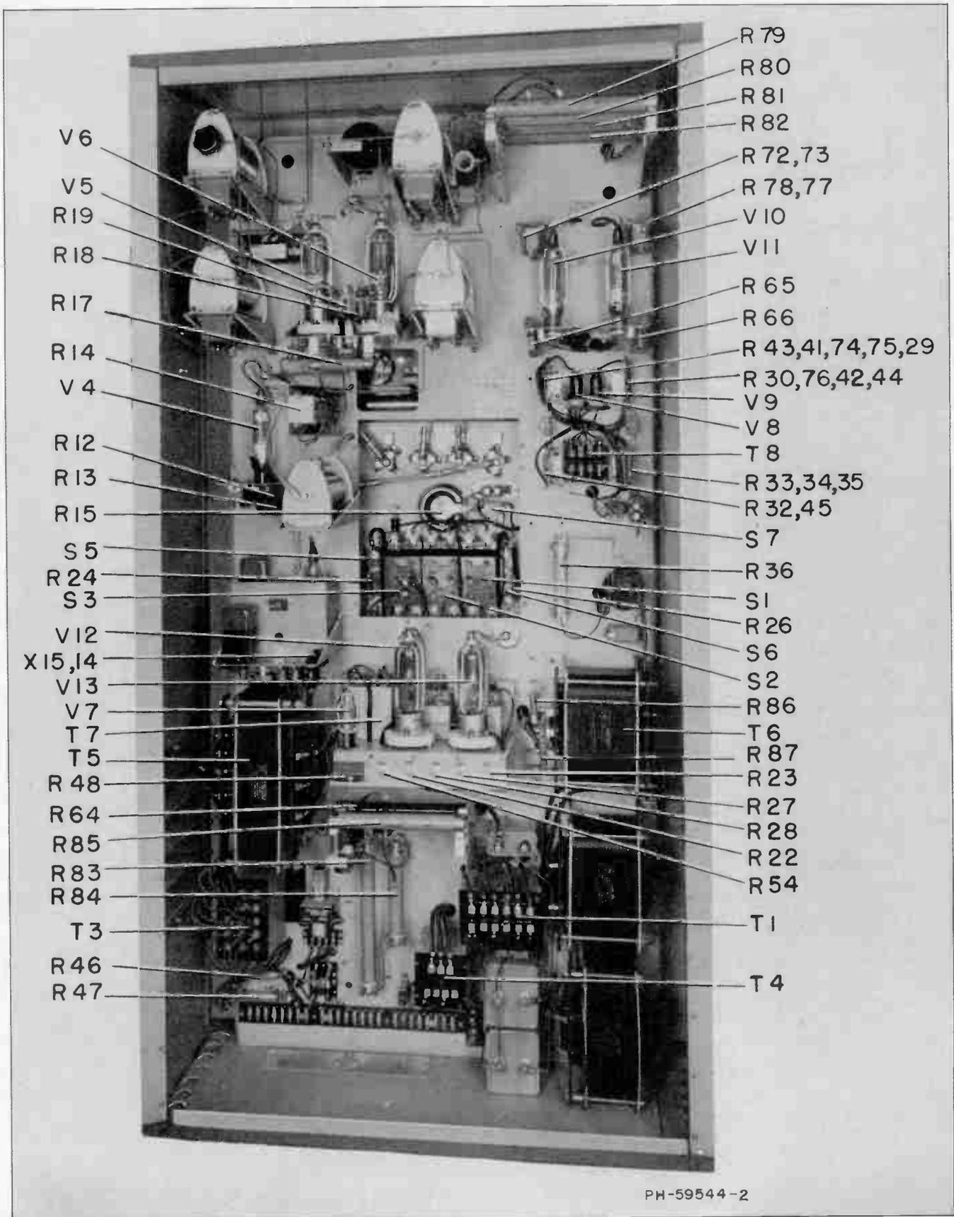
Figure 5—Transmitter Chassis
