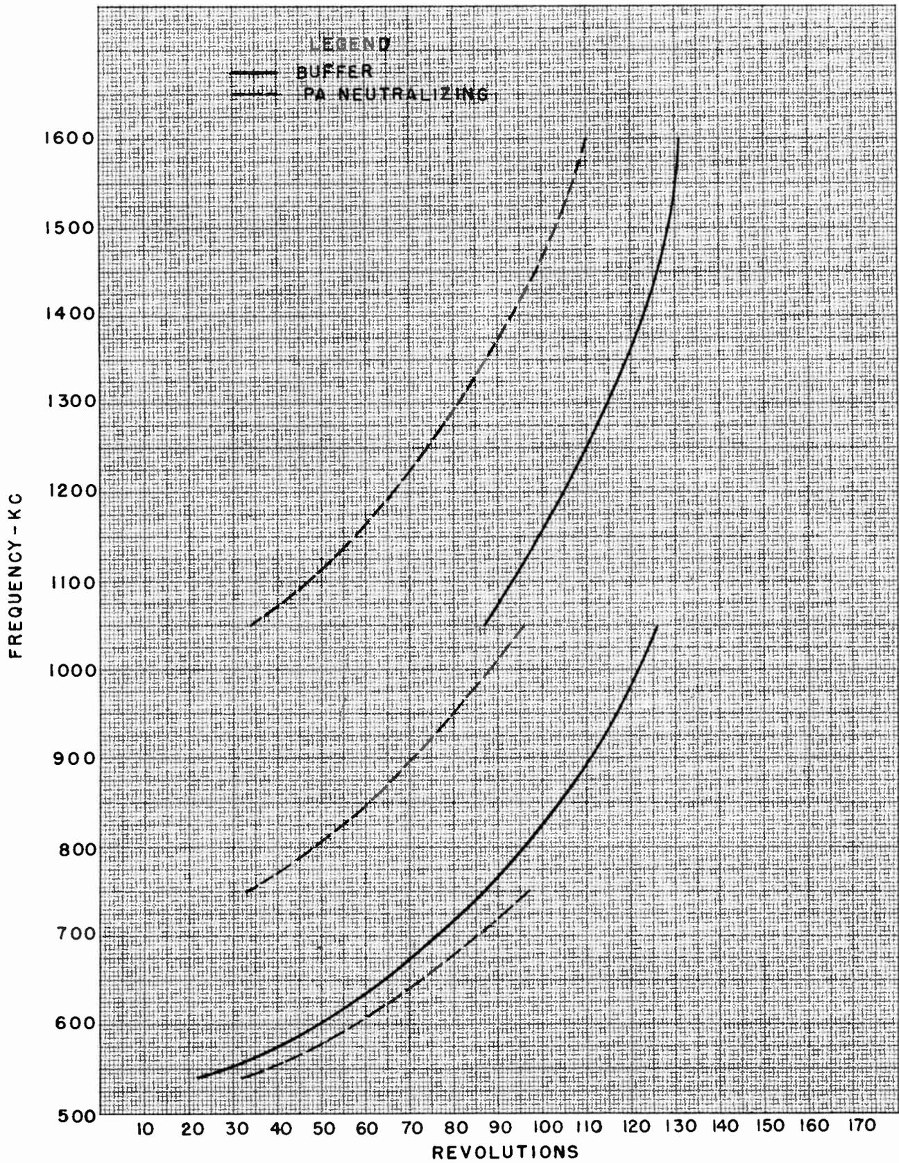
Figure 11—"P.A. NEUT." and "BUFFER" Dials (L7 and L5)
