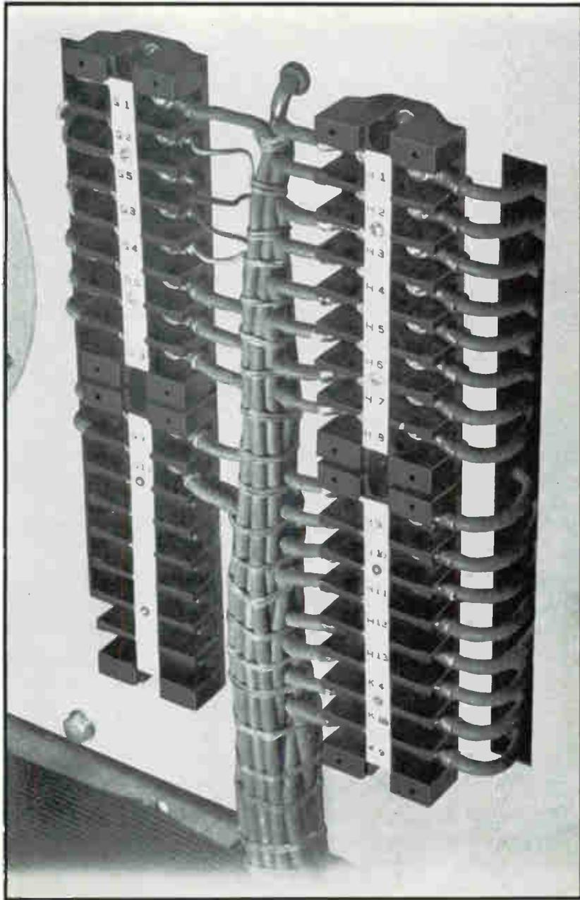
Figure 2—Interconnecting Cable Lacing
