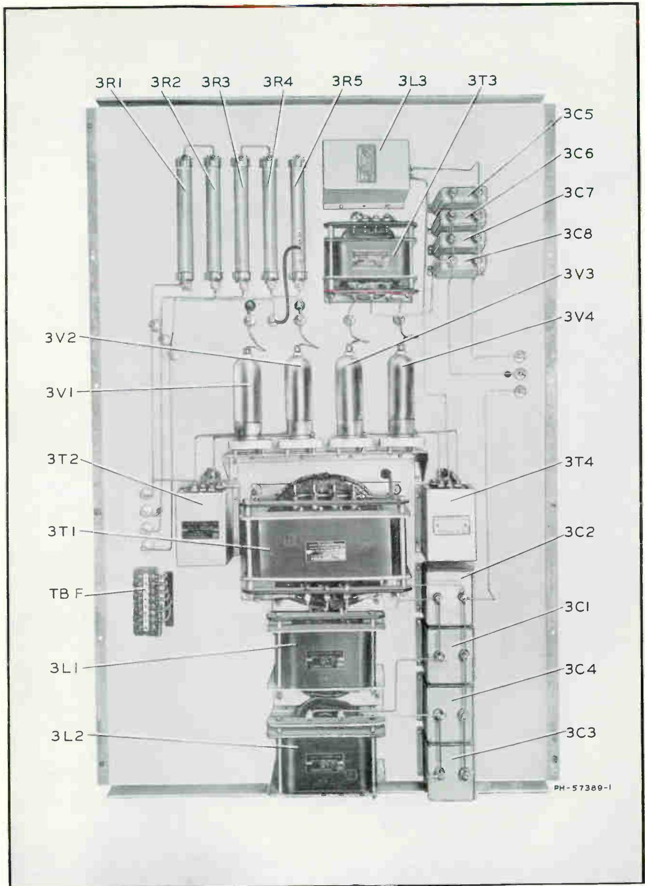
Figure 13—Bias and Auxiliary Rectifier Chassis
