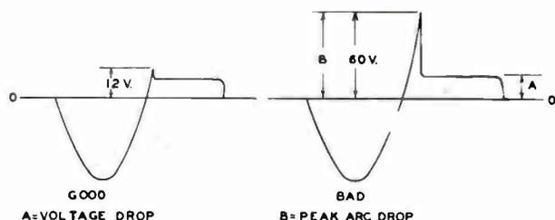
Monthly records of arc-drop measurements will provide accurate tube data at roughly 500-hour intervals. When peak arc-drop values in the region of the 30- to 40-volts are indicated, more frequent tests may be desirable. Because the oscillographic tests reveal peak arc-drop voltages and give an accurate picture of the firing characteristic, this method of testing rectifier tubes is recommended as being much more valuable than older d-c methods of measurement. If the 115-volt
