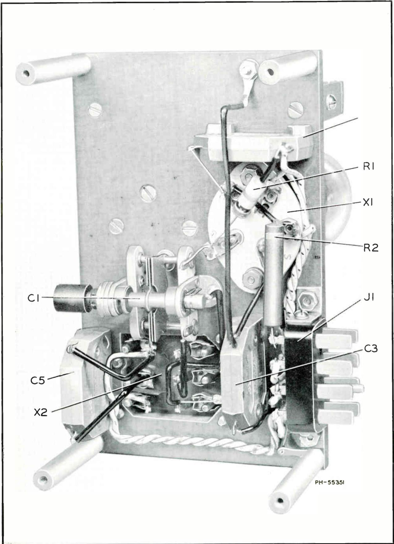
Figure 12—R-F Oscillator Unit (Bottom View, Covers Removed)
