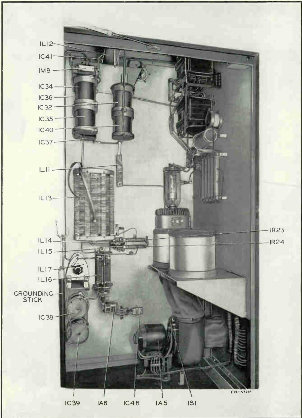
Figure 8—R-F Output Tank Chassis
