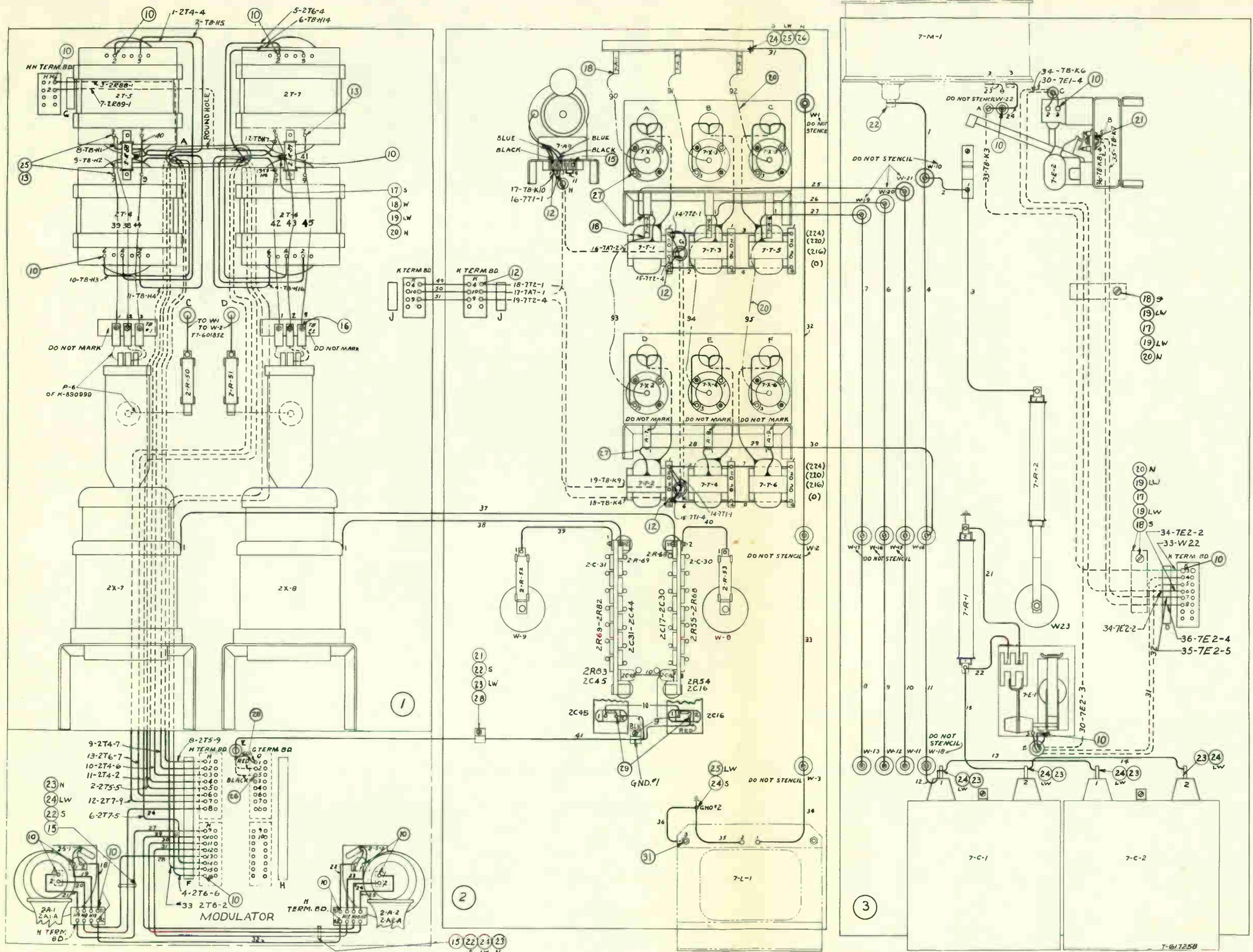
Figure 30—Modulator, Main Rectifier and Rectifier Auxiliary Chassis Connections (T-617258)
