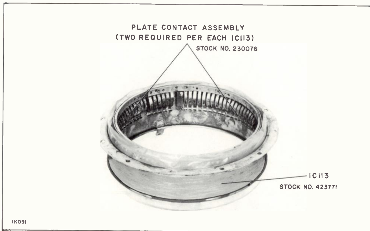
Figure 27. 1V102 Plate Contacts and Plate Blocking Capacitors
