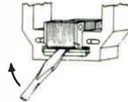
**REPLACING OPERATING COIL**
