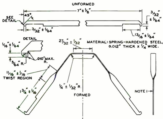
NOTE 1: BURR MUST NOT EXCEED 0.002" IN DIRECTION PERPENDICULAR TO FLAT SURFACES. THE CORRESPONDING FLAT SURFACES OF THE TWO LEGS SHOULD BE IN THE SAME PLANE WITHIN 1/16."
