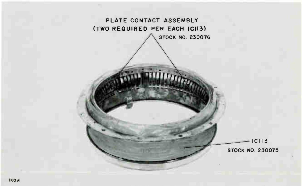
Figure 27. 1V102 Plate Contacts and Plate Blocking Capacitors
