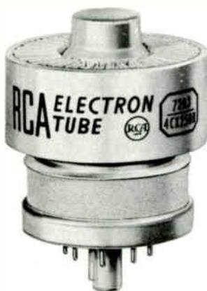
The ceramic-metal-seal construction employed in the 7203 permits operation at higher temperatures than a glass-seal construction and thus provides improved reliability. The specially designed, high-efficiency radiator which is brazed directly to the plate for better heat transfer, makes possible the maximum plate-dissipation rating of 250 watts with no sacrifice in tube reliability.
