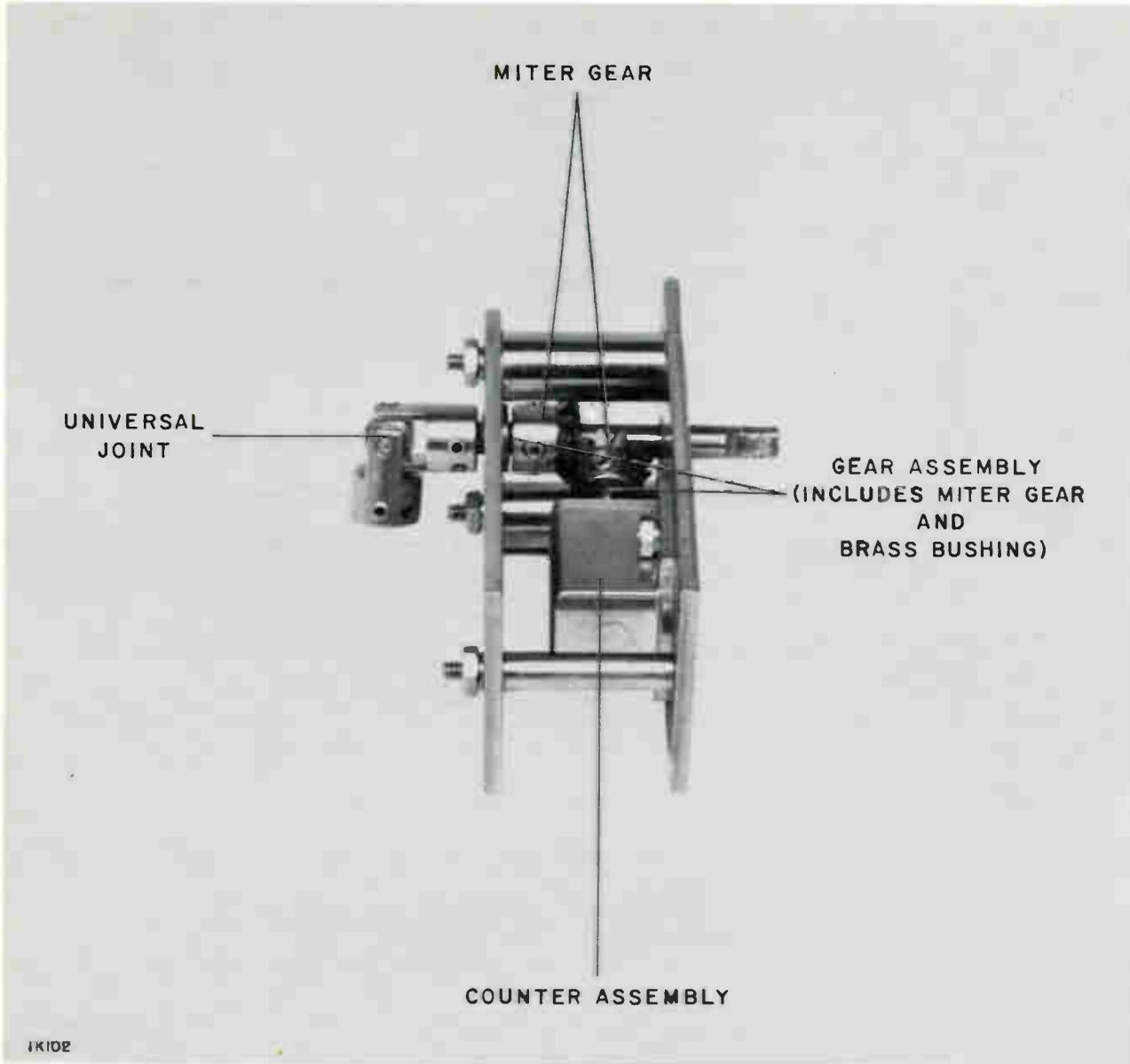
Figure 28. 1L105 and 1L106 Counter Assemblies
