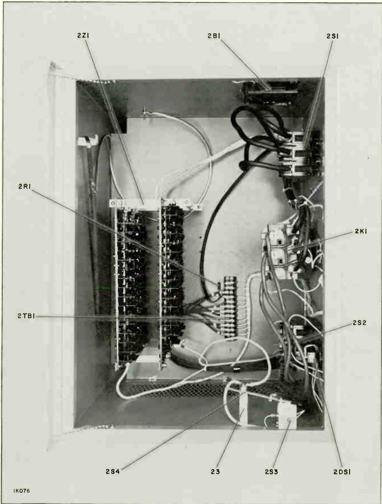
Figure 36. High Voltage Power Supply, Top View
