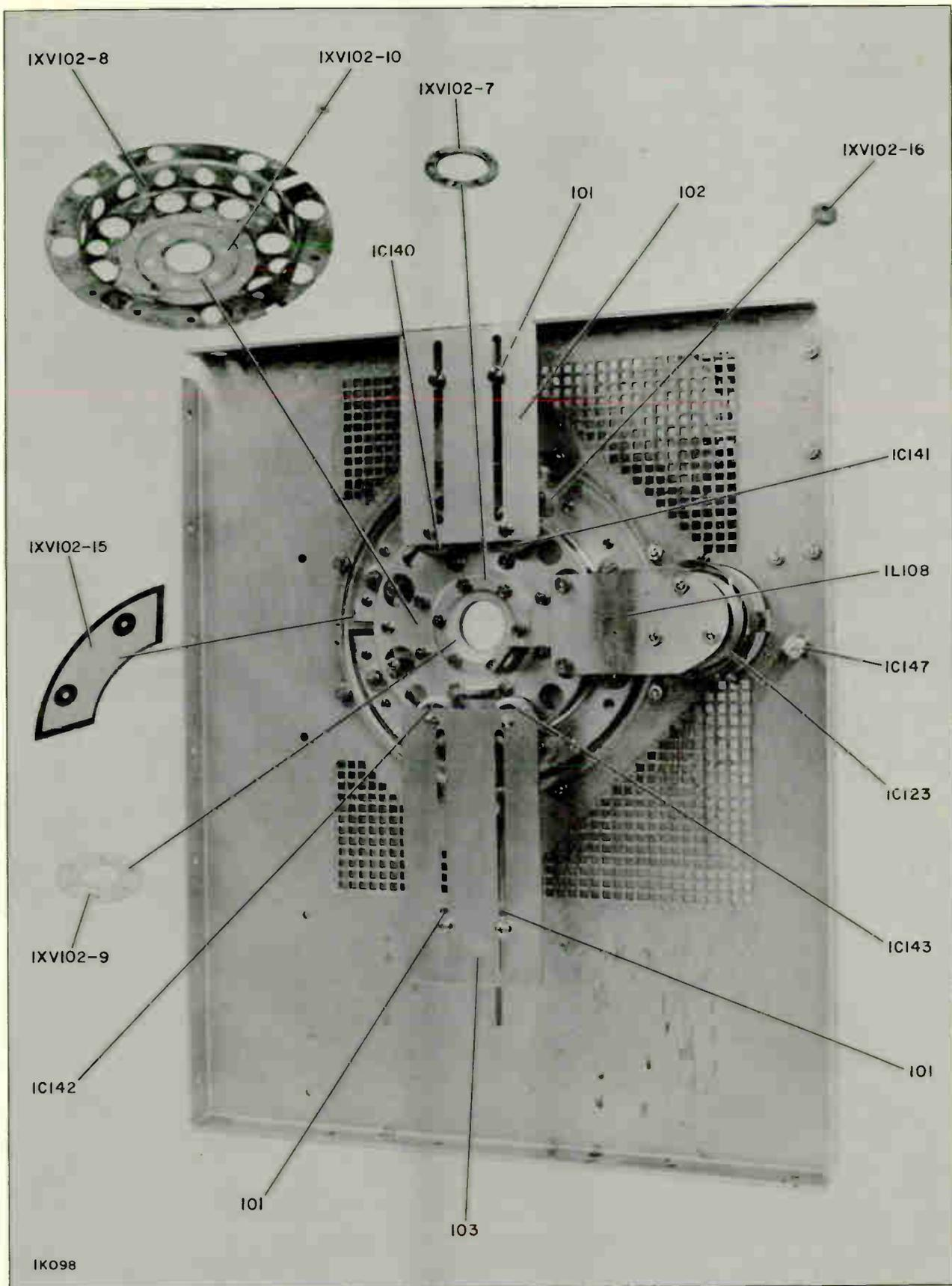
Figure 24. 1XV102 Socket Assembly, Bottom View
