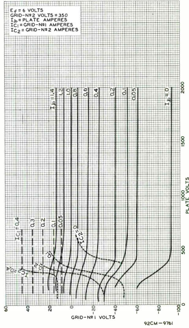
Fig. 4 - Typical Constant-Current Characteristics of Type 7203.
