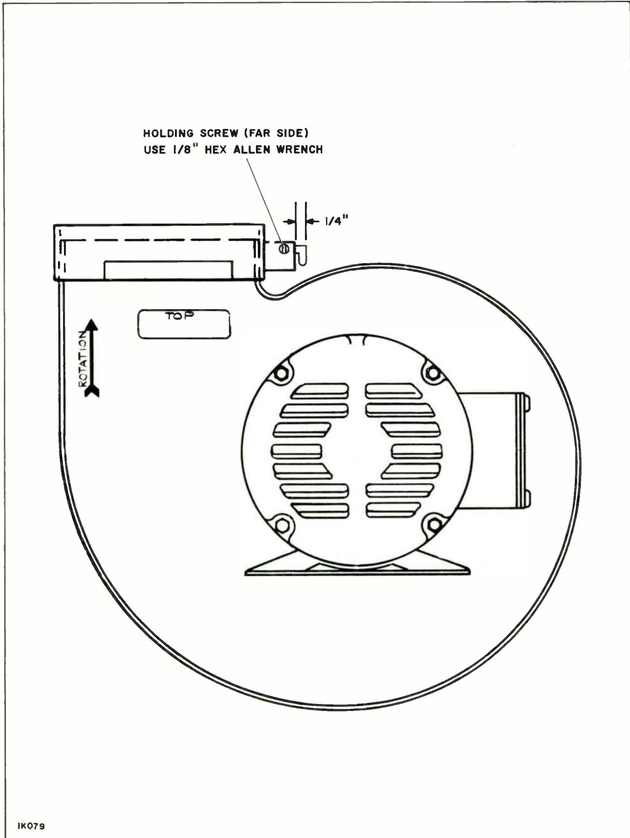
Figure 48. Blower Vane Setting
