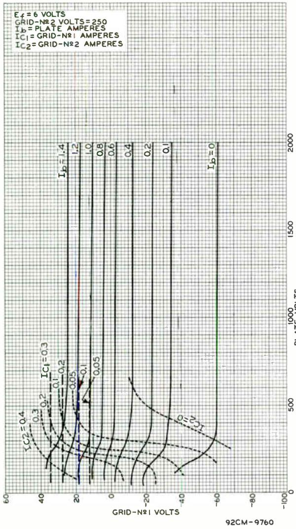
Fig. 3 - Typical Constant-Current Characteristics of Type 7203.
