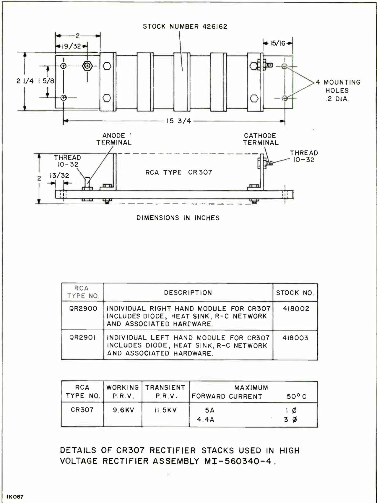
Figure 44. High Voltage Rectifier Assembly
