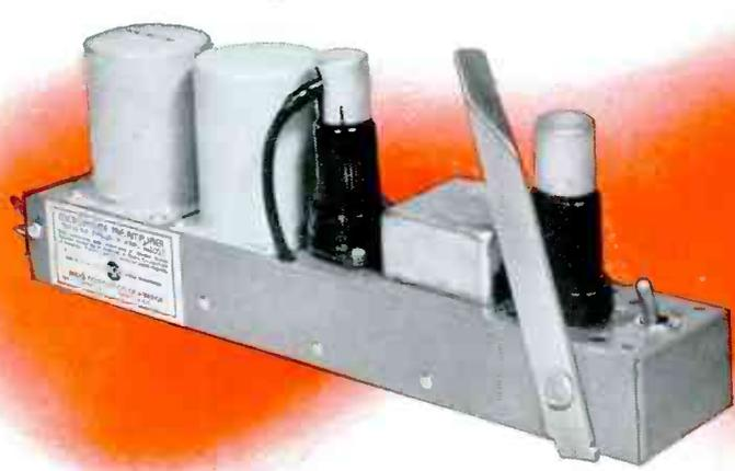
**Two-stage Preamplifier (Type BA-11A)**—Ideal for use as a microphone preamplifier, turntable preamplifier, booster amplifier, or low-level isolation amplifier. *High gain:* 40 db. *High output:* +10 db. *Low noise level:* -80 db. *Low distortion:* 0.5% rms, 50 to 7500 cycles. *Isolation factor:* approx. 90 db; over 100 db with special Volume Control Kit. *Frequency response:* ±1 db, 30 to 15,000 cycles. *Small size:* six units will fit on a 36-B or new BR-2A shelf!
