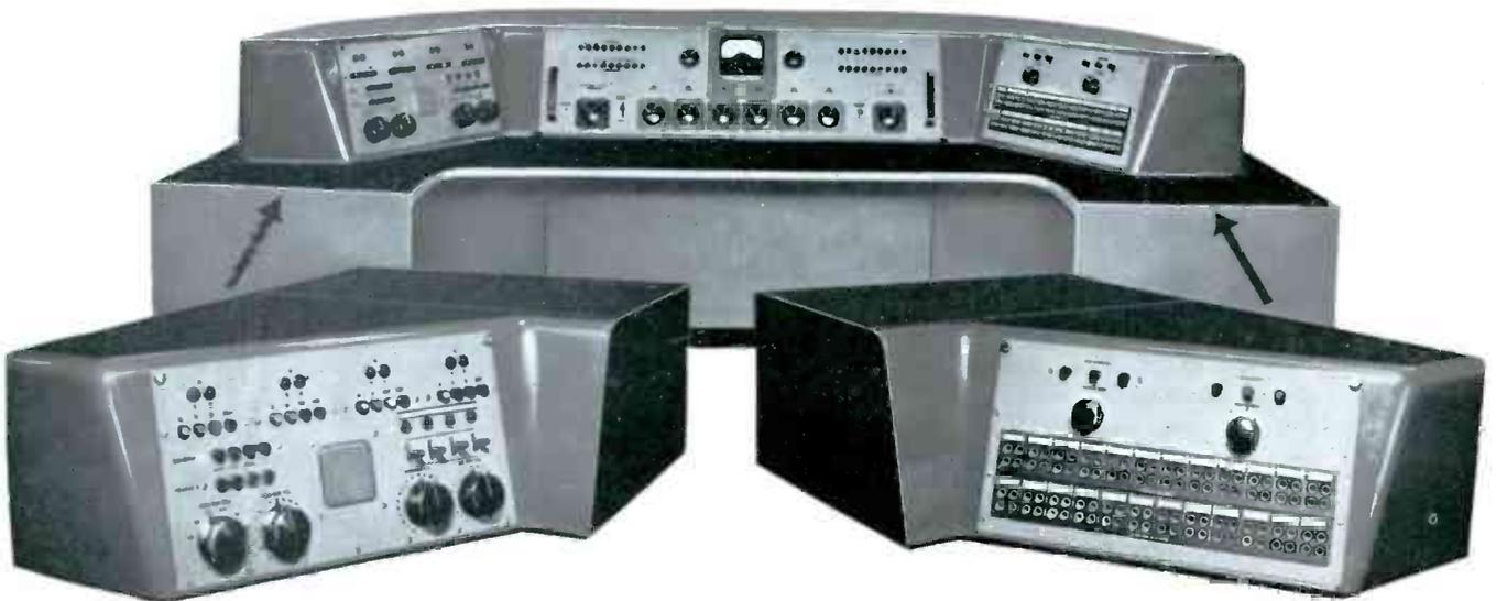
The arrangement above shows how special matching consoles are designed for desk-top use with any standard 76-series console. Such consoles may contain special talkback facilities, order wire ringdown circuits, monitor controls and signal lights. Jack panels may be included, if desired, for use with the 76 console. In addition to the special end cabinets shown here, "straight" type cabinets to match 76-series consoles are also available.
