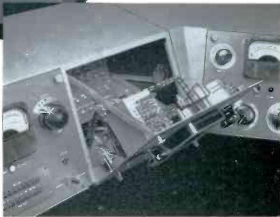
Combining master and studio control facilities, this all-metal console includes eight individual panel sections which are: l. to r. (Studio "B", Remote Line, MCR (4 panels), Studio "C", Announce and Studio "D".) Front cover panels in lower desk sections are removable to provide access to relays, terminal boards and coils. Desk design and panel spacing permits four video monitors to be mounted directly on top of the center section.
