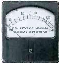
**REMOTE ANTENNA AMMETER, MI-7184-A-150**
