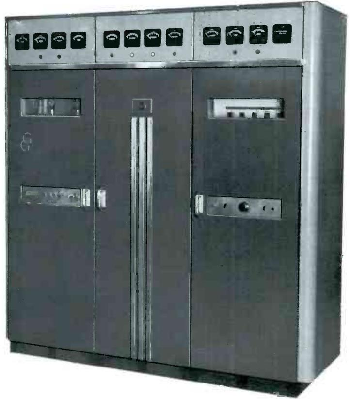
The entire transmitter is housed in three fabricated steel frames which are bolted to a base frame. Each compartment has both front and rear doors which are provided with observation windows. End shields and meter panels complete the cabinet type enclosure which has been styled functionally to present a pleasing and dignified appearance. Filtered air, supplied through individual air inlet openings and removable filters are provided in the base frame. Warm air is expelled through the roof.
