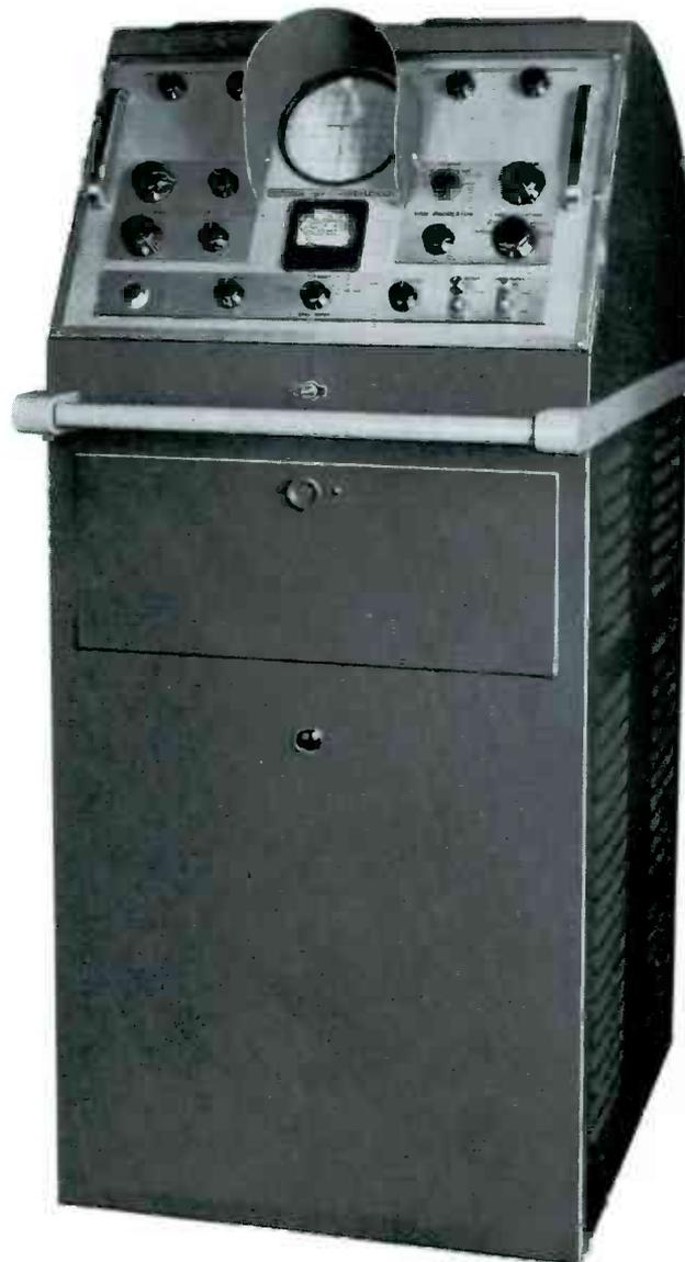
Triggered Sweep Speed—2 to 100,000 microseconds per inch
