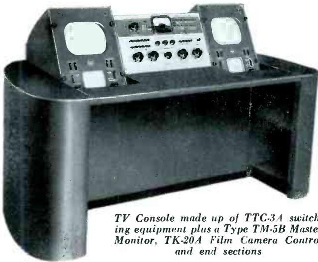
TV Console made up of TTC-3A switching equipment plus a Type TM-5B Master Monitor, TK-20A Film Camera Control and end sections
