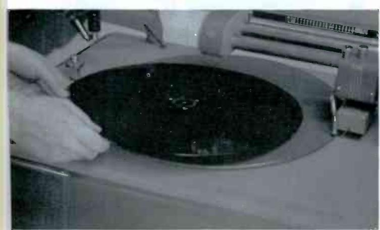
**ANY TYPE BLANK** may be used with the single driving pin provided. Here, recording blank is placed in position.
