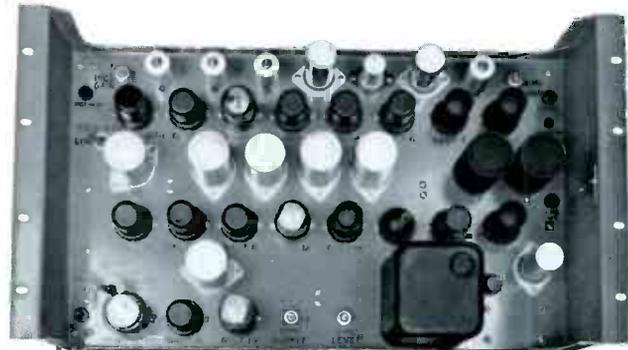
A two-position attenuator at the input accommodates a range of input signals from 0.25 volt to 15 volts, peak-to-peak. The output of the amplifier is designed to deliver the standard level of picture and blanking signal (1.5 volts, peak-to-peak) with a maximum sync of 1.5 volts peak-to-peak. The amount of sync can be adjusted independently to any value between 0 and 1.5 volts, peak-to-peak.
