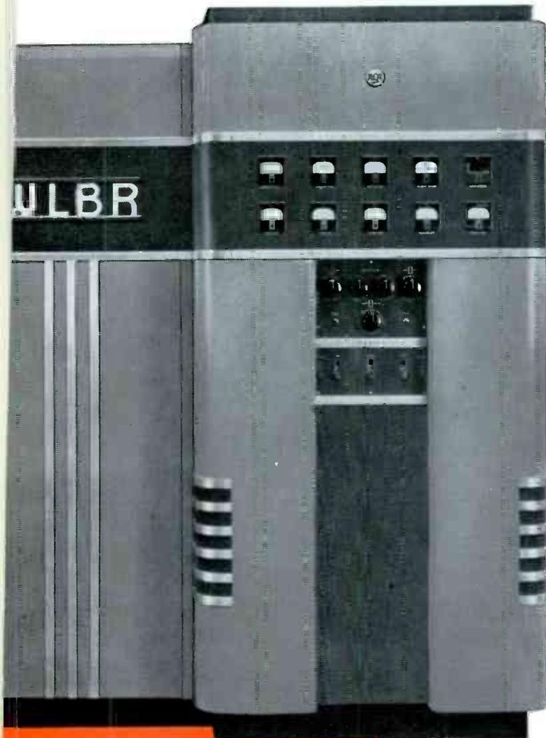
... add on this 1-kw Power Amplifier type BTA-1L for high power later
