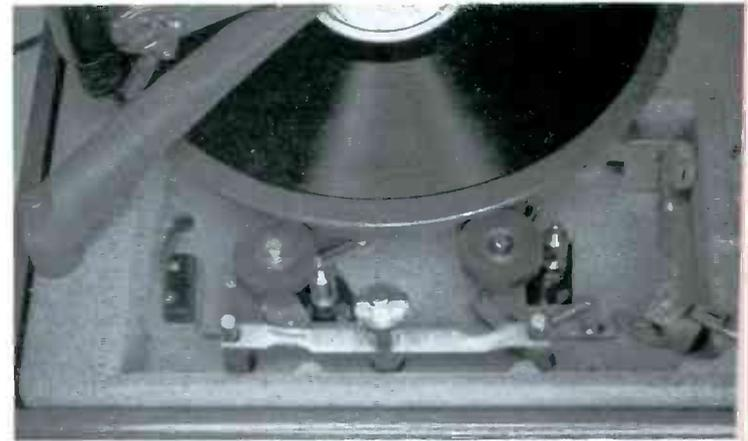
**ON-78 RPM**—In "ON" position, the brake shoe moves away from turntable rim and rim and rubber idlers are now in active contact with drive wheel and turntable rim.
