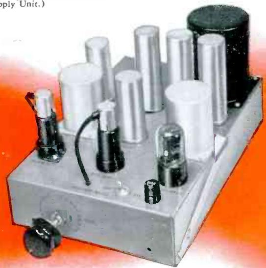
**Booster Amplifier (Type BA-2C)**—A two-stage unit having applications similar to those for the BA-1A; also valuable where a high-gain amplifier between announce microphone and limiting amplifier is required. *High gain:* 50 db. *Low noise level:* -68 db. *Low distortion:* 0.75% rms, 40 to 15,000 cycles. *Frequency response:* ±1.5 db, 30 to 15,000 cycles. *Compact:* two units can be mounted on one 36-B or BR-2A shelf. Features plug-in capacitors and built-in power supply.
