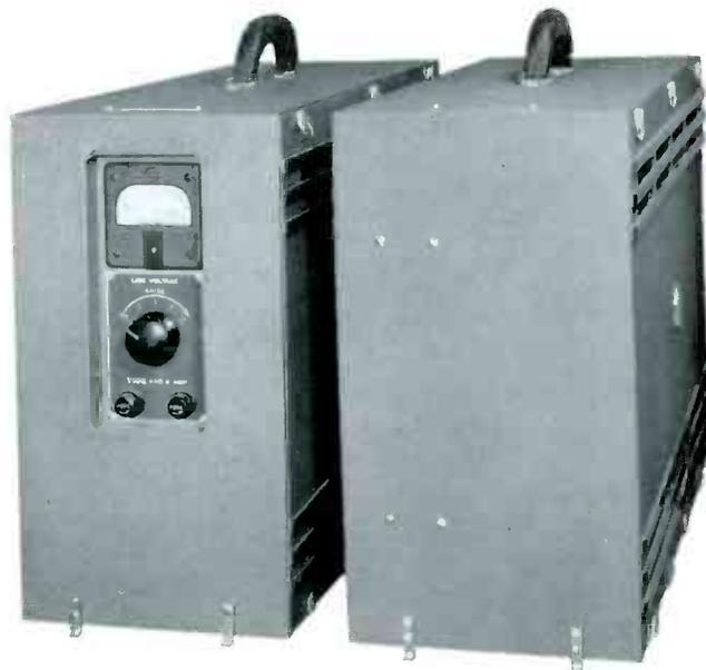
series of counters for stepping this master frequency down to line frequency (15,750 cycles) and to field frequency (60 cycles), and an automatic frequency control circuit for locking the synchronizing generator to the power supply frequency. A crystal oscillator operating at 94.5 kc. is provided as an alternative means of controlling the frequency of the generator where the power supply system is not stable enough to serve as a reference.
