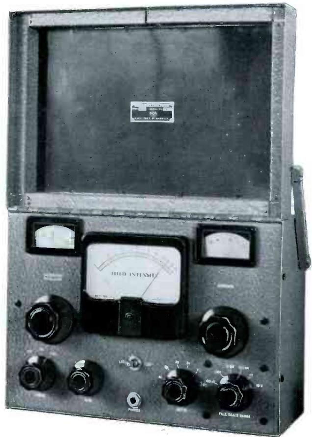
The direct reading feature of the WX-2C simplifies field intensity measurements and eliminates the needs of the usual attenuator readings, meter readings and multiplication factors. A wide sensitivity range, 10 volts per meter to 10 microvolts per meter, permits maximum flexibility of operation within the range of 540 to 1600 kc.
