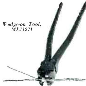
All frayed edges are cleanly cut away and a perfect electrical and mechanical connection results.
