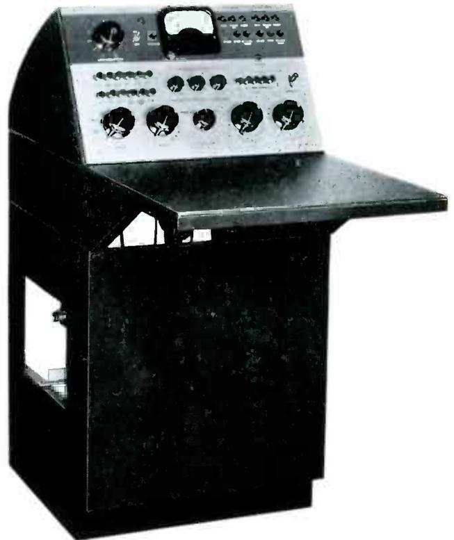
Picture gain, picture clipper and sync level controls are extension controls for remote operation of the RCA TA-5C Stabilizing Amplifier. The video gain control remotely controls the video gain fader in the transmitter.
