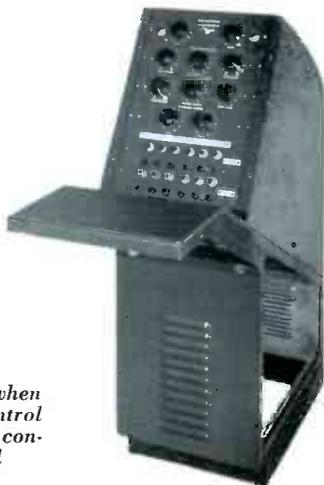
*The MI-26223 Panel, when mounted in Remote Control Console MI-26252, provides convenient Master Control facilities.*
