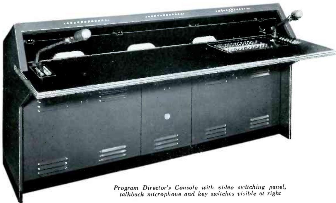
*Program Director's Console with video switching panel, talkback microphone and key switches visible at right*
