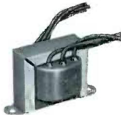
This transformer is ideal for operating a number of medium power speakers with a voice coil having 6 or 2 ohms impedance. The primary winding has three taps for 4000, 8000 and 16,000 ohms. It is designed for bracket mounting and has 10" connection leads. The same transformer, hermetically sealed for tropical use, is available as MI-12374.
