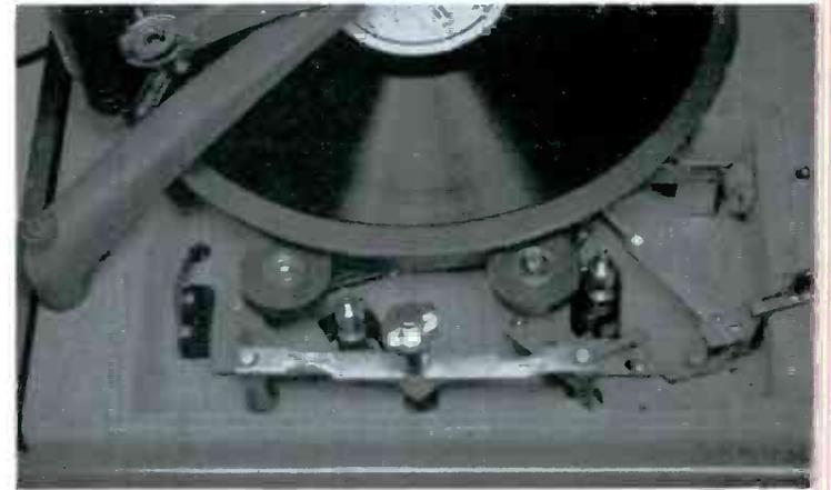
**AT- $33\frac{1}{2}$  RPM**—With speed change knob "UP," rubber idlers are moved vertically to low-speed position of drive wheel (note drive wheel has "lo- and hi-speed" shoulders of different diameters).
