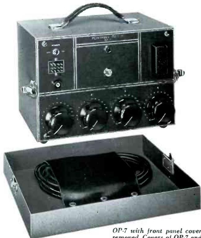
OP-7 with front panel cover removed. Covers of OP-7 and OP-6 provide space for carrying interconnecting cables.
