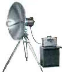
**RCA Microwave Relay Transmitter TTR-1A.** Transmits the picture signals from field to studio (or from studio to transmitter). It includes a parabolic antenna with hook-shaped wave guide, built-in transmitter, and remote control unit. Matching receiver unit at the station picks up the microwave relay signal.
