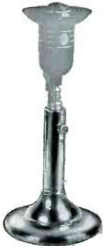
This smartly designed table stand features a built-in microphone switch and is suitable for use with all RCA pressure type microphones. The switch is of the D.P.D.T. long leaf anti-capacity type and permits turning the microphone on and off right at the microphone stand. It may also be used for 'push-to-talk' operation or lock-in "Talk" position.
