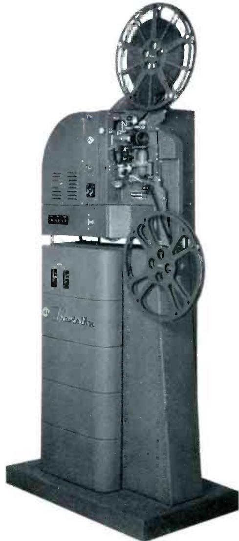
The film feed arrangement of the TP-16B is identical to that of the standard projector with the exception that the pull-down claw works at a greater speed. Film is fed from the upper reel under a large sixteen-tooth feed sprocket and through the precision made film gate. Light, controlled by a rotating shutter, is projected through the film at this point. The film is pulled down through the gate, a single frame at a time, by the pull-down claw just below the gate.
