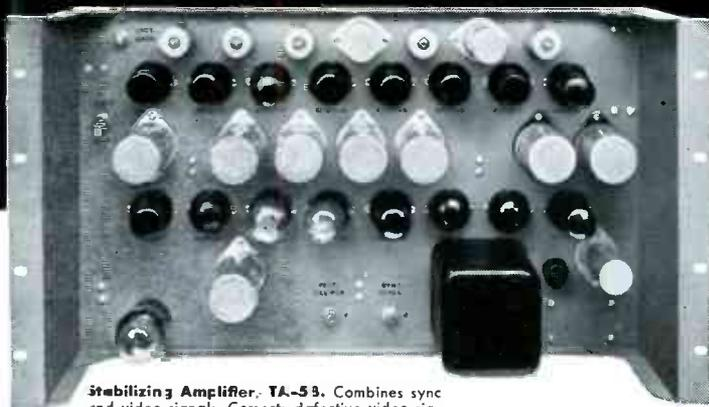
**Stabilizing Amplifier, TA-5B.** Combines sync and video signals. Corrects defective video signals. Eliminates rum. Corrects low-frequency response. Improves signal-to-noise ratio of sync signals.
