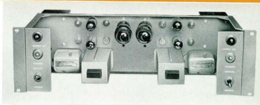
The remote power indicator also operates from the output reflectometer circuits. Two cathode follower circuits are used. One provides a voltage reference level, and the other provides a low voltage which varies with the input signal (reflectometer output). The voltage appearing at the output terminals is therefore proportional to the reflectometer voltage and has good linearity due to the cancellation of Edison effect in the tubes.
