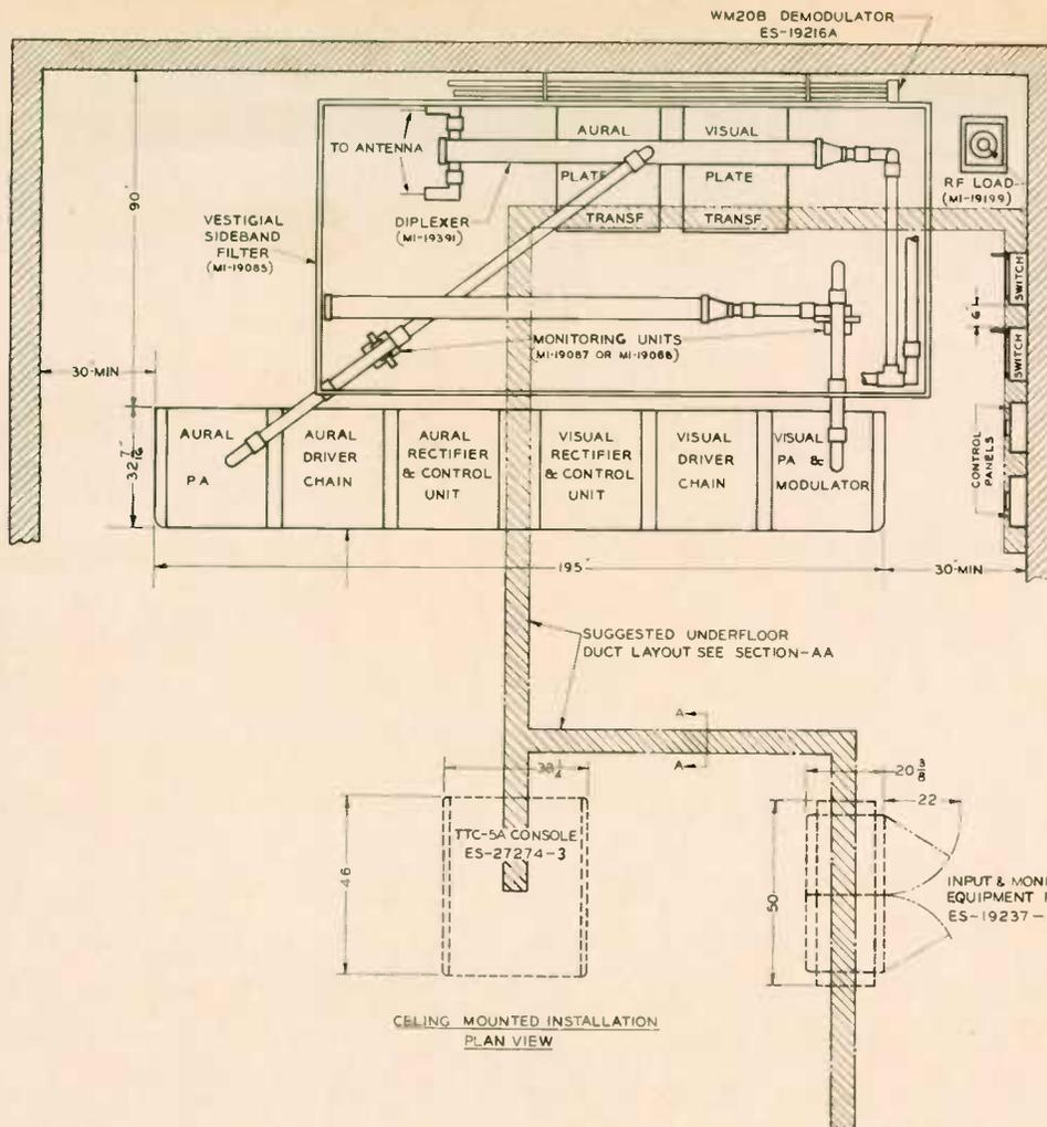
Floor Plan Layout of the TT-10AL 11-KW VHF Transmitter.
