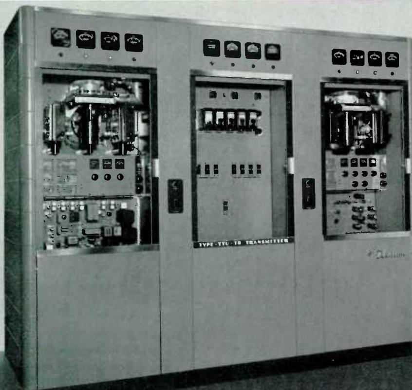
View of TTU-1B Transmitter with sliding panels open to show front panel components and controls. Cabinets left to right are: Aural, Power Control, and Visual.
