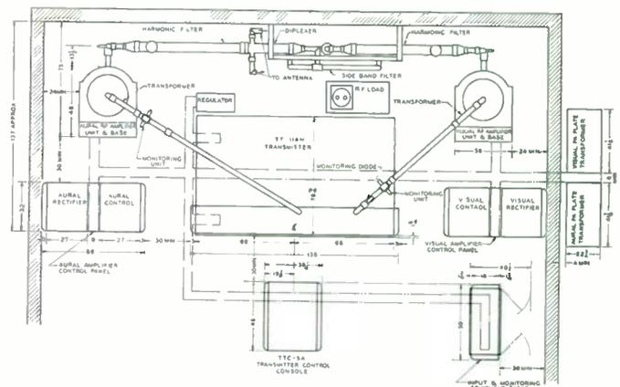
▲ Typical floor plan of TT-11AL Transmitter with TT-25BH amplifier.
