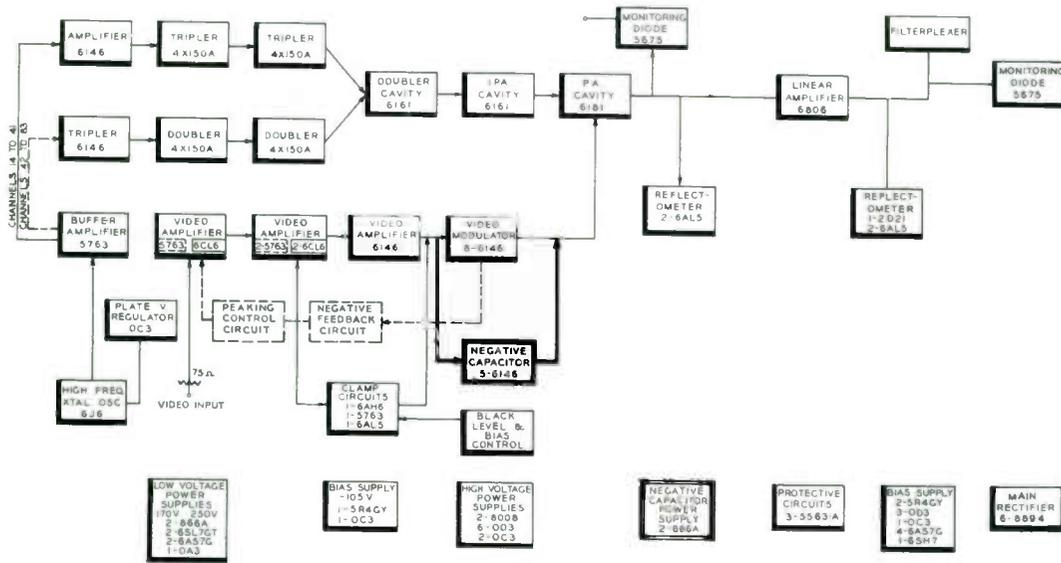
and metering of all important circuits. Operation can practically be reduced to turning "on and off" at the transmitter. Power output meters are supplied for both picture and sound transmitters. These meters also indicate VSWR. Facilities are provided to permit continuous picture monitoring (which is necessary to assure proper adjustment for color) at various points in the system.
