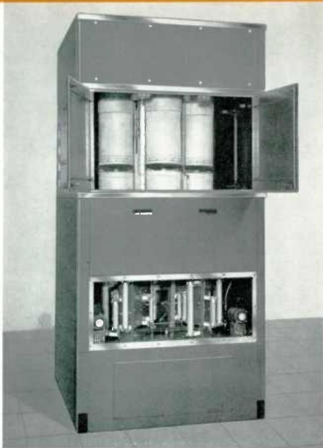
Rear view of the 50-KW Power Amplifier showing RCA type 6166 tetrodes with protecting air ducts above, and circuit components below.
