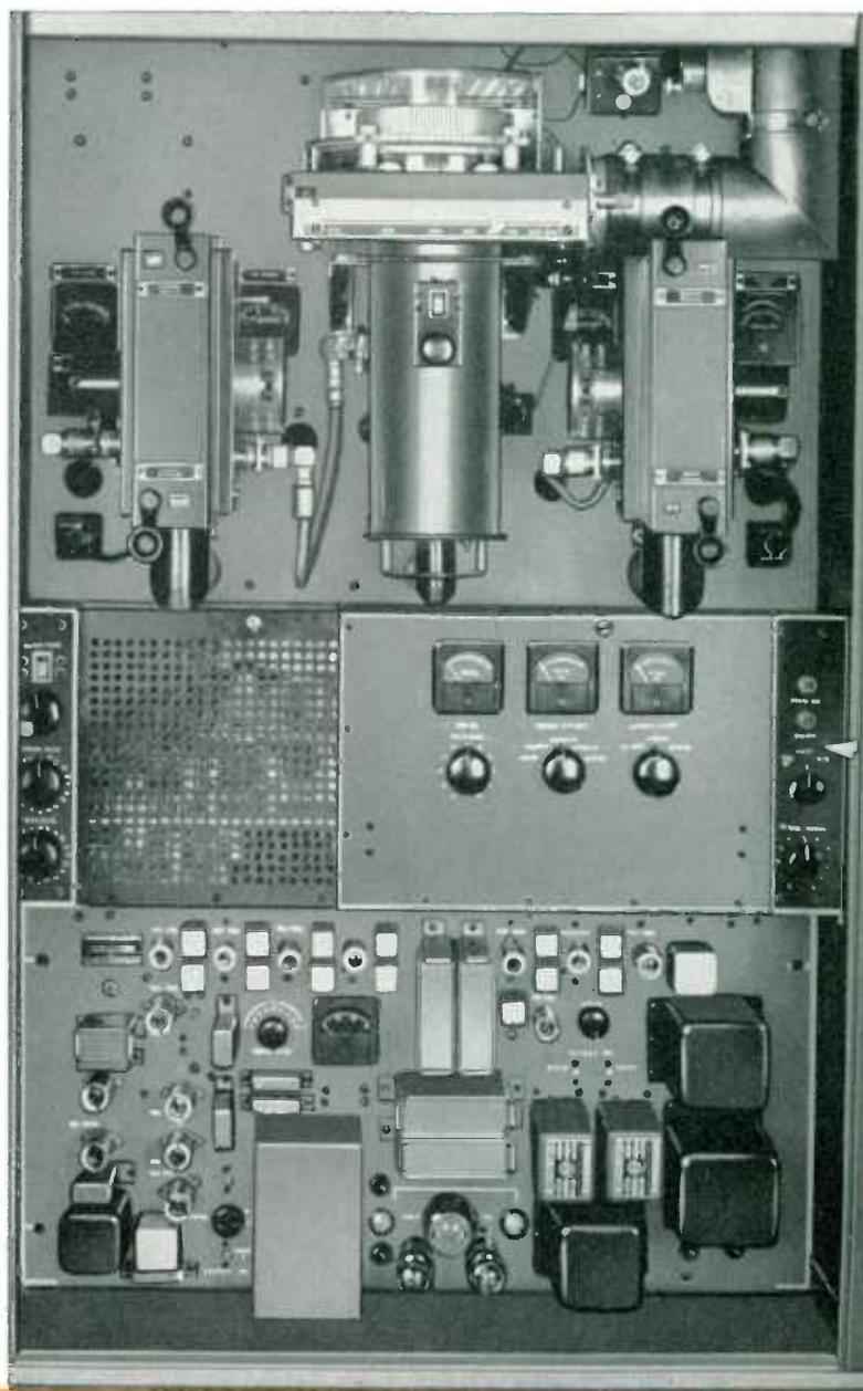
Power Amplifiers. Associated with this common power supply is a high-voltage transfer switch which enables the operator to transfer the high voltage only to the visual side. Thus emergency repairs may be performed on the aural P.A. while programming is continuing with 1-KW aural power and 25-KW visual power.
