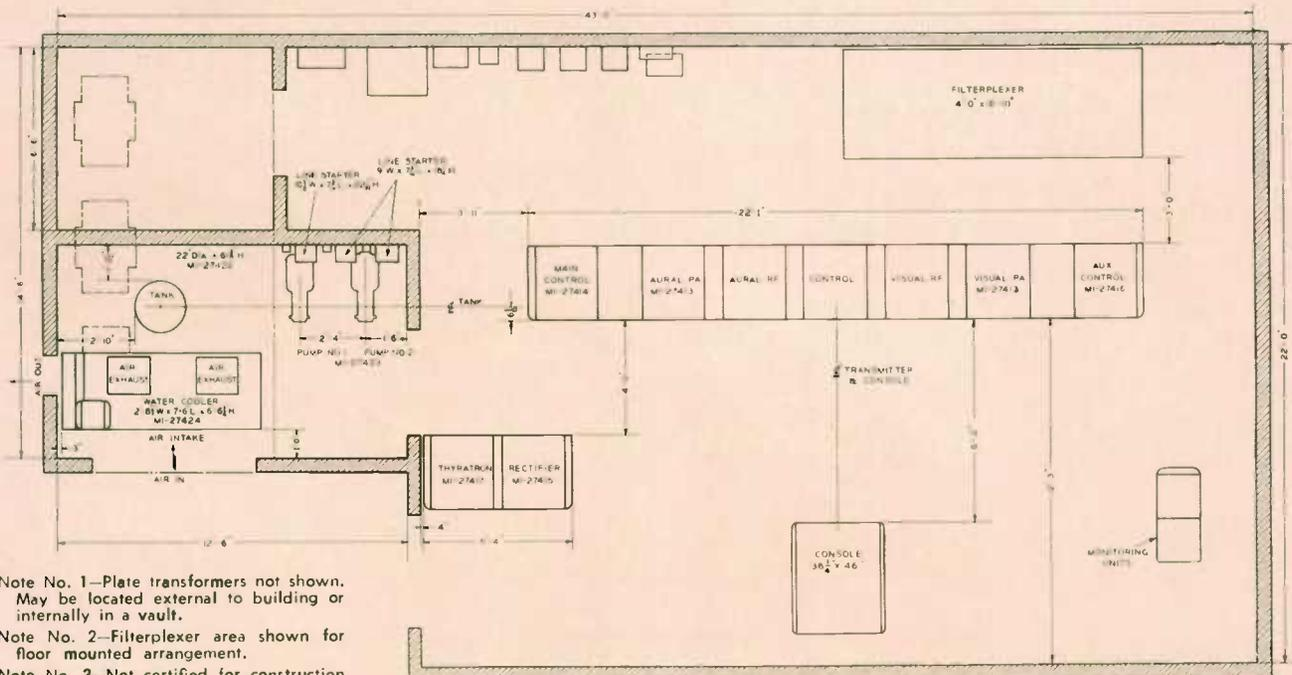
Note No. 1—Plate transformers not shown. May be located external to building or internally in a vault.
