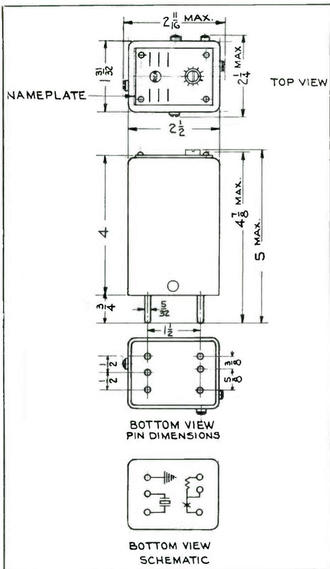
Each TMV-129-B unit employs an AT-cut low-temperature coefficient quartz plate. The crystals are pre-dimensioned to provide the maximum freedom from spurious responses. Each plate is nearly one-inch square and has a thickness depending upon frequency. In the low portion of the frequency range the crystals are relatively heavy, as much as 1/8 inch thick. In spite of this they oscillate with excellent freedom.
