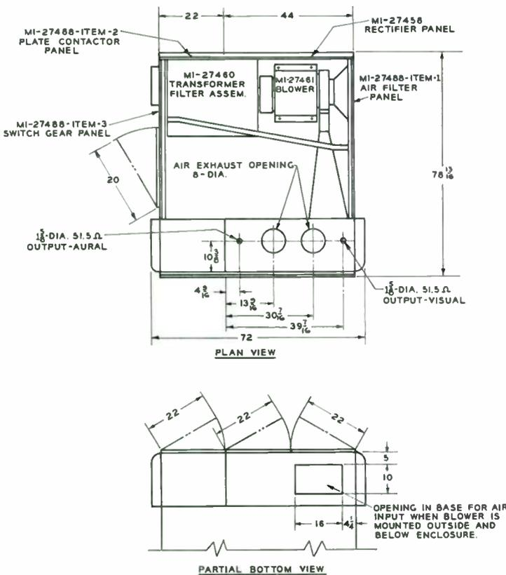
Typical floor plan for the TT-2BH VHF Transmitter showing compact equipment unit and rectifier enclosure.
