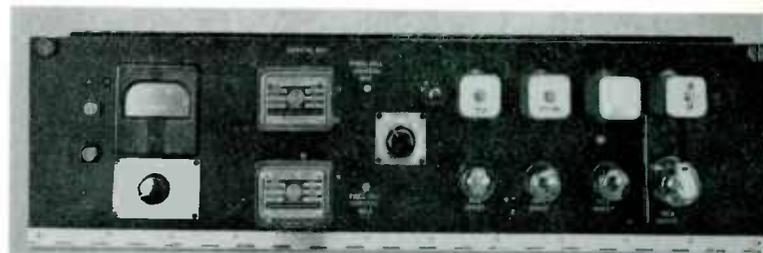
Crystal control is used to maintain frequency accuracy to  $\pm 1$  kc in the visual transmitter. This order of stability is of great importance when offset carrier operation is employed. Stability is achieved through careful application of temperature control to the crystal. The crystal is operated in a low power crystal oscillator circuit from which the output frequency  $1/6$  of the assigned frequency of the TT-10AL.
