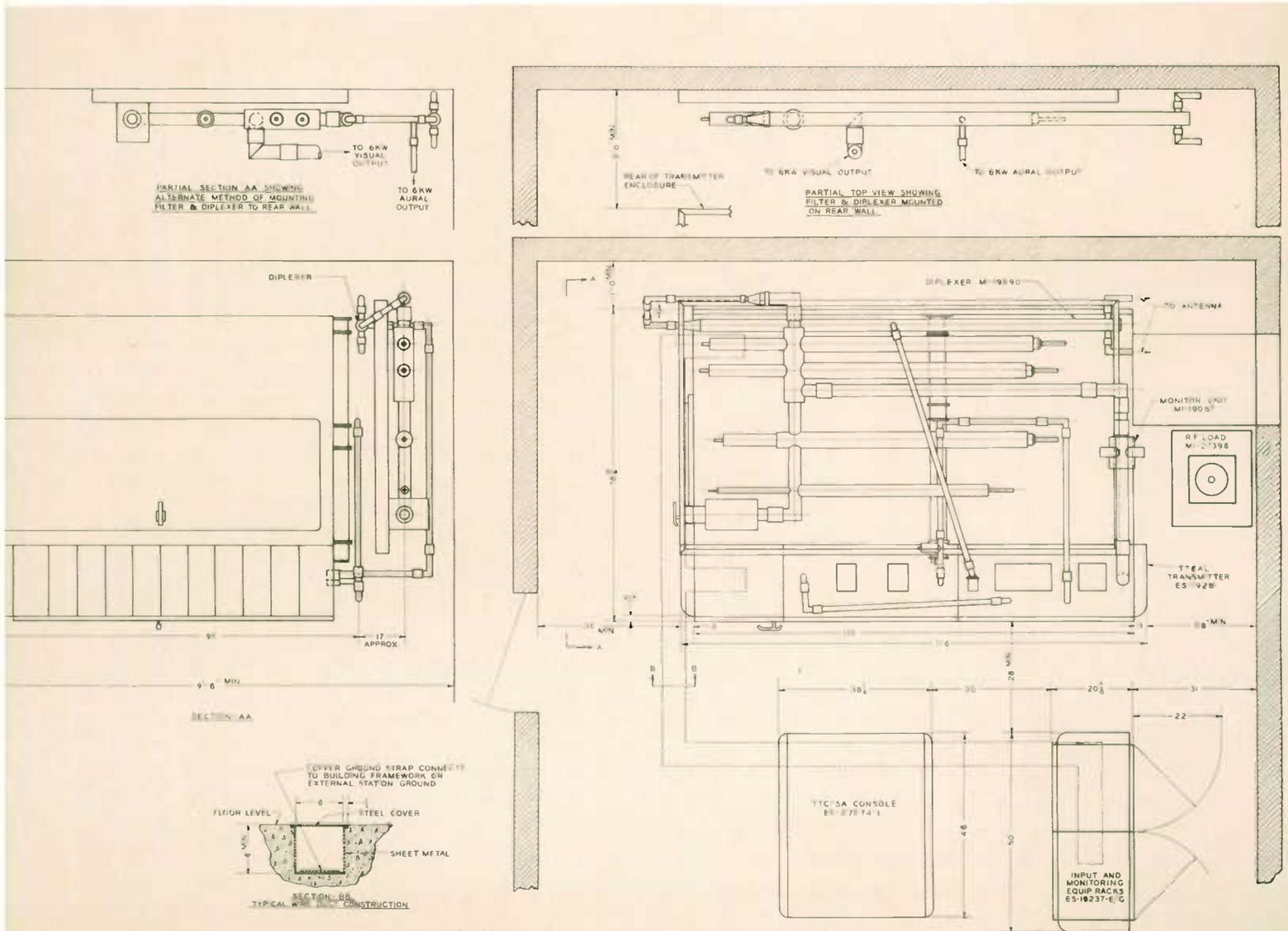
Typical Floor Plan #1 for TT-6AL transmitter with rectifier enclosure attached.
