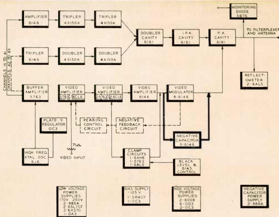
Block diagram of TTU-1B Visual Transmitter.
