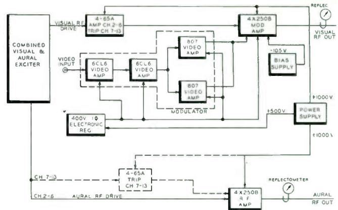
Simplified block diagram of the TTL-100AL/AH Transmitter.
