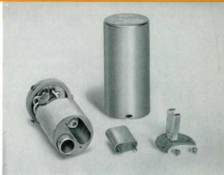
Disassembled view of an MI-27492 television crystal showing base assembly with heater oven and thermostat at left, can housing, crystal unit in two-prong cartridge case, and at right the crystal holder and semi-circular oven cover with mounting screws.
