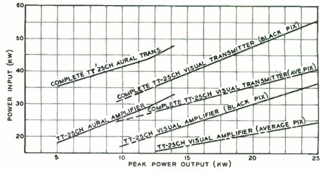
Power consumption curves showing approximate Power Input vs. Peak Power Output of the TT-25CL and the TT-25CH Visual and Aural Transmitters.
