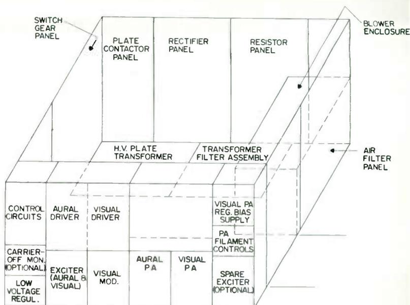
Walk-in type construction of the driver permits easy servicing. Rectifiers and cooling equipment are at the rear of the enclosure. The remaining portions of the driver are in the front line of cabinets.
