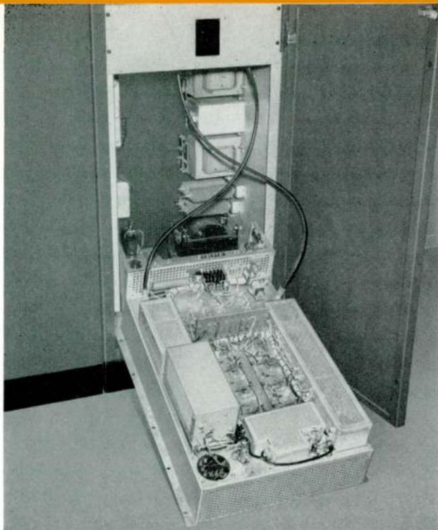
Aural and visual exciter circuits of the TTL-500AL/AH are mounted on a single hinged chassis allowing access to transformers, filter and other components housed in bottom of transmitter cabinet.
