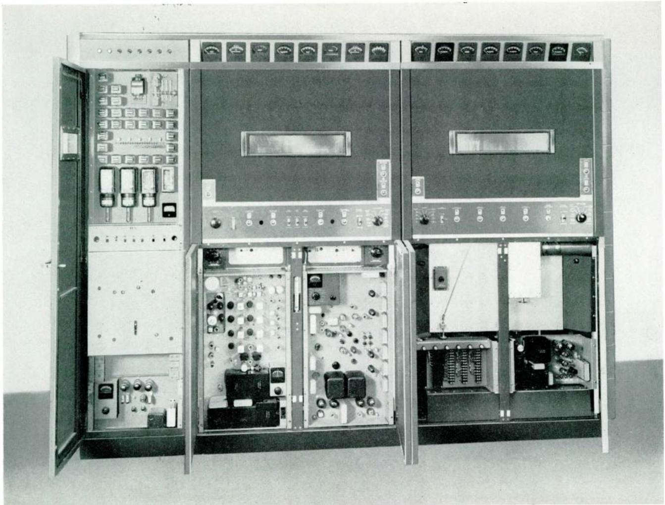
Full view of TT-6AL Driver, cabinet doors open revealing tuning controls and meters, control cabinet (left) exciter and modulators on accessible hinged chassis (center) and 6 kw PA cabinet with reflectometer switches and power supplies among lower components (right).
