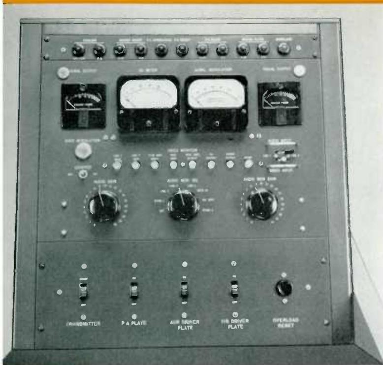
Closeup view of indicator, monitor control and transmitter control panels mounted in 22 inch console housing.
