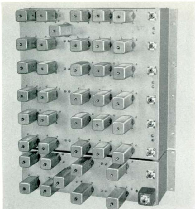
Rear view of Phase Equalizer Equipment showing one Amplitude Equalizer Unit mounted in lower right corner on the Low Frequency Chassis.
