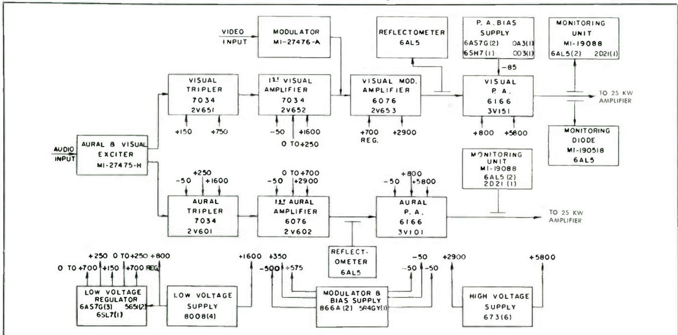
making one of these transformers variable in characteristic impedance as the outer shell is rotated through 90 degrees. With few exceptions, identical components are used for aural and visual circuits throughout the TT-25CH transmitter. It is therefore possible to reduce spare tube and parts inventory as much as 50 percent.
