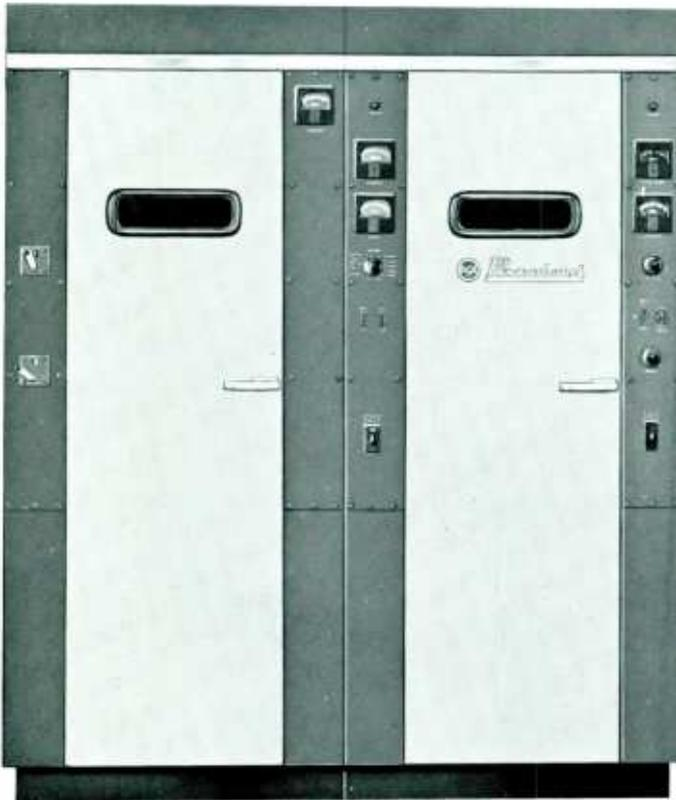
BTA-1R2 Transmitter with matching left-wing phasing cabinet.
