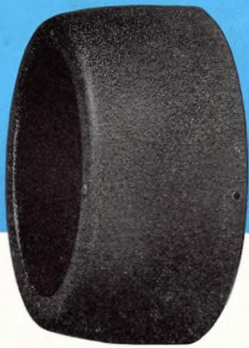
**RCA Metal Housing**—This metal speaker housing is designed for applications where rugged unit of neat appearance is desired. It is made of steel and finished in an attractive brown wrinkle lacquer. For MI 6248-A speaker unit or other 8-inch speakers of similar dimensions. It is 9 $\frac{5}{8}$ " in diameter, 4" deep, and weighs only 2 lbs. (less the speaker unit). Shipping weight, 4 $\frac{1}{2}$  lbs.
