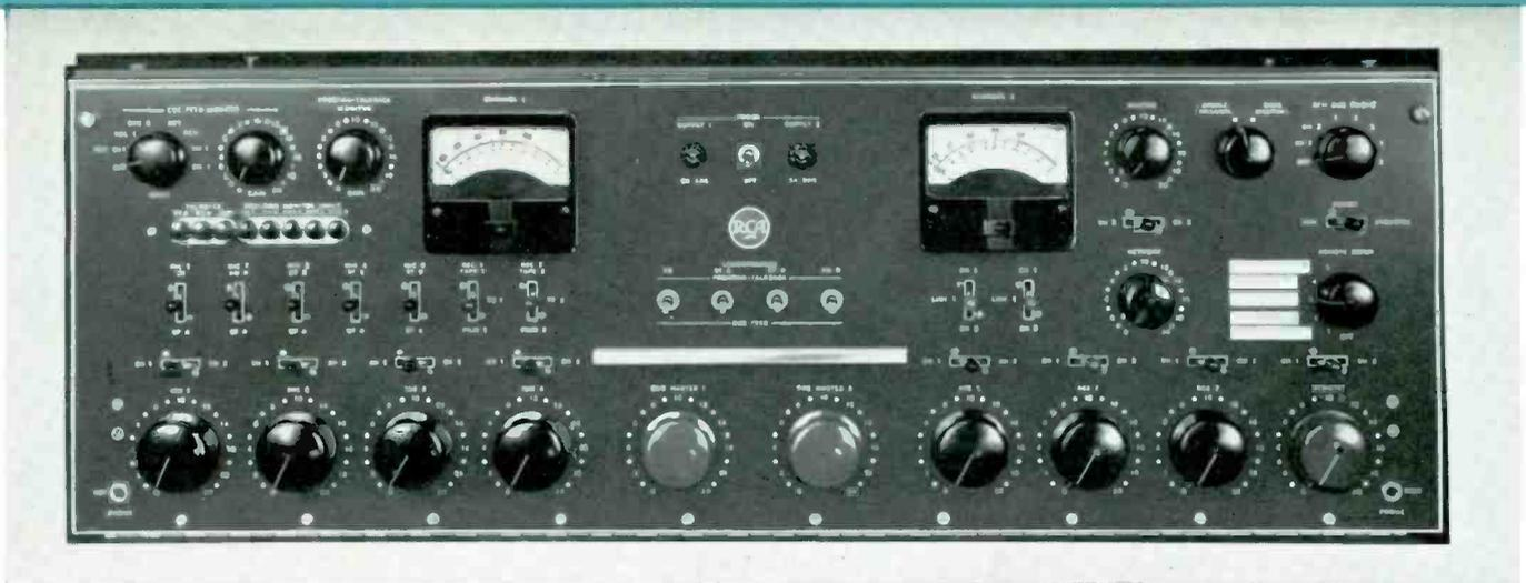
Etched front panel of the BC-6B Consolette showing entire operating facilities.
