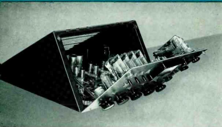
The BC-5B hinged front panel and removable top cover provide complete access to all components including amplifiers and power supply.
