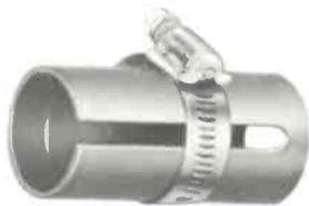
Inner and outer conductor guides that assure square cut.
