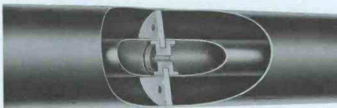
Efficient, precision-built line and line accessories. Featuring an electrically transparent Teflon insulator, this line uses the familiar bolt-flange connection. Insulator characteristics and precise inner-conductor centering allows cutting and re-flanging in the field without a change in operating impedance at the cut.
