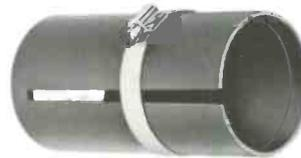
Inner and outer conductor cutoff. Guides that assure square cut.
