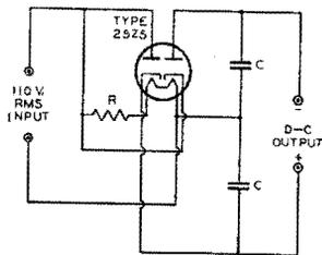
R=HEATER VOLTAGE REDUCING RESISTOR
