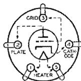
The 37 is a three-electrode tube of the heater-cathode type. The relatively low heater current of this type makes it suitable for automobile receivers and for power-line-operated sets, particularly those with a series-heater arrangement.
