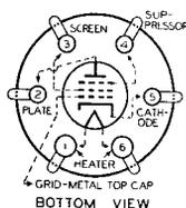
this tube to handle the usual signal voltages without cross-modulation and modulation distortion makes it adaptable to the r-f and i-f stages of receivers employing automatic volume-control. The 6D6 is constructed with an internal shield connected to the cathode within the tube.
