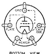
ance, and its comparatively high amplification factor. The 56 is useful in resistance-coupled audio-frequency amplifiers.
