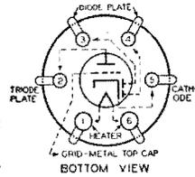
The 2A6 is a 2.5-volt heater type of tube consisting of two diodes and a high-mu triode in a single bulb. It is for use as a combined detector, amplifier, and automatic-volume-control tube in a-c receivers designed for its characteristics. For diode-detector considerations, refer to page 19.
