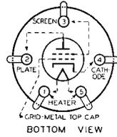
tion and modulation-distortion over the entire range of received signals. Its design is such as to permit easy control of a large range of signal voltages without the use of local-distance switches or antenna potentiometers. This super-control feature makes the tube adaptable to circuits incorporating automatic volume control. See page 11 for Super-Control feature. The 35 is interchangeable with type 51.
