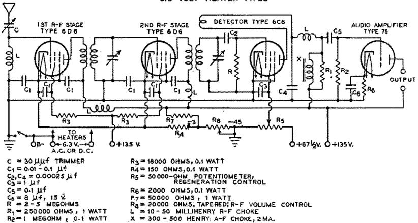
NOTE: TYPES 56, 57, AND 58 MAY BE USED IN THIS CIRCUIT IN PLACE OF THE 7B, 6C6, AND 6D6 RESPECTIVELY, PROVIDED THEY ARE OPERATED AT THEIR RECOMMENDED HEATER, SCREEN, PLATE AND GRID BIAS VOLTAGES.
