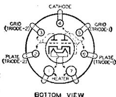
The 53 is a heater-cathode type of tube combining in one bulb two high- $\mu$  triodes designed for Class B operation. It is intended primarily for use in the output stage of a-c operated radio receivers. The
