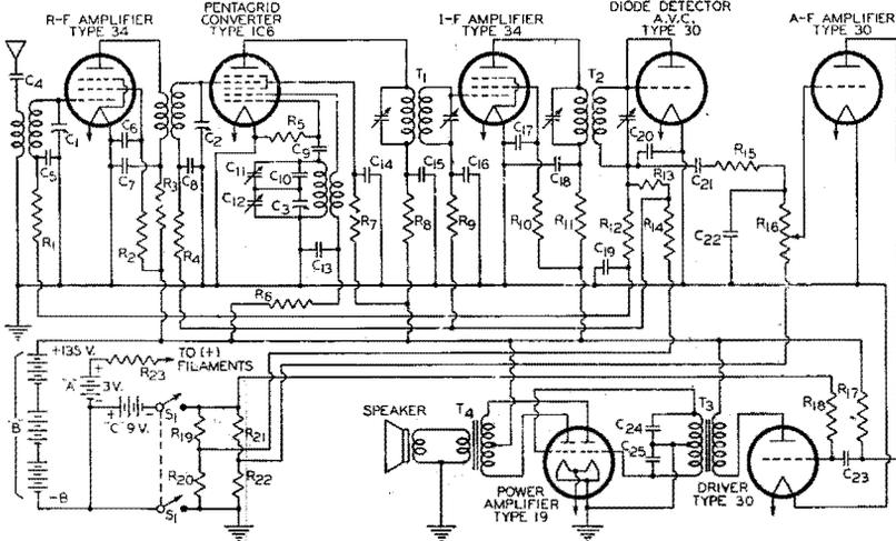
C<sub>1</sub>, C<sub>2</sub>, C<sub>3</sub> = GANGED VARIABLE CONDENSERS
