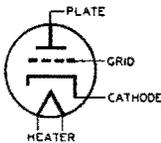
When the grid of a tube is made positive or negative with respect to the cathode, the plate current correspondingly increases or decreases. The grid is located much nearer the cathode than the plate so that a small voltage change on the grid will have the same effect on the plate current as a larger voltage change on the plate. A grid requires very little power, serving merely as a valve to control the plate current.
