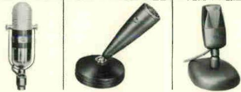
**POLYDIRECTIONAL MICROPHONE, 77-DX.** Famous for high-quality reproduction. Provides a choice of directional pick-up patterns... uni-directional, bi-directional, non-directional, three-position voice-frequency range, 60-10,000 cycles.
