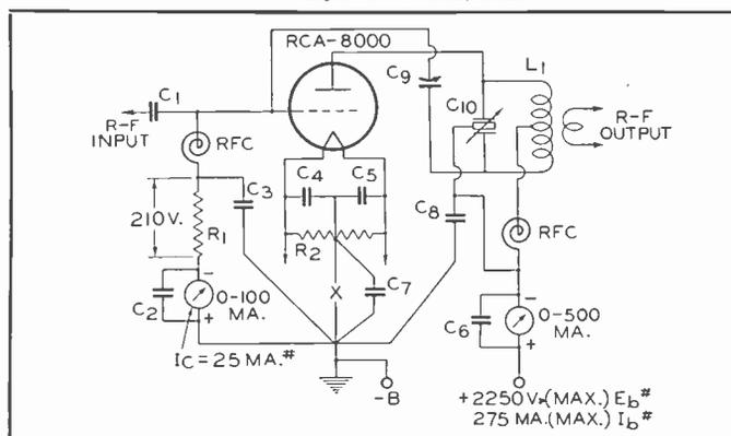
C<sub>1</sub>=0.0005  $\mu\text{f}$ , mica, 1500 v.
