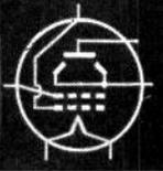
As Plate-Modulated R-F Power Amplifier—Class C Telephony
