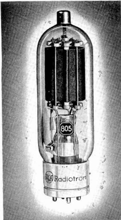
RCA-805 is a husky high-mu transmitting triode of the thoriated-tungsten filament type with a maximum plate dissipation of 125 watts (CCS). It is designed both for class B modulator service and for r-f amplifier service. Grid-bias requirements of the tube are unusually low. For example, at the maximum plate-voltage rating of 1500 volts in class C telegraphy, a bias of only -10 volts is needed to protect the tube against loss of grid-excitation voltage.
