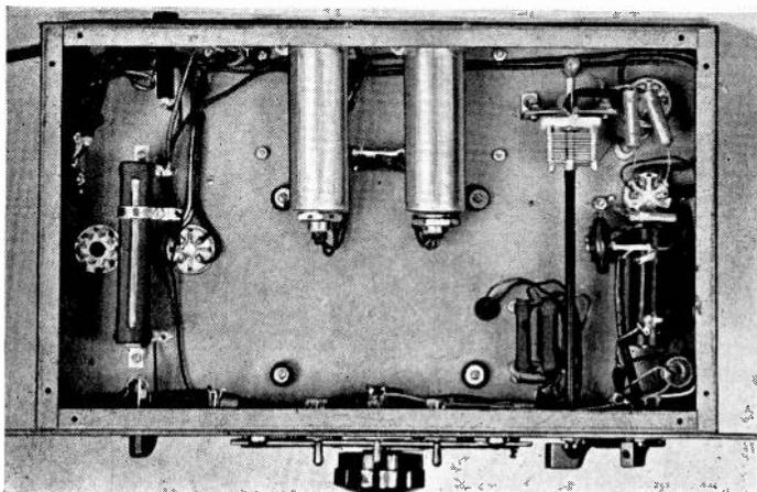
mined. The bottom cover of the can may be mounted by means of the four rubber washer assemblies. The dial and  $C_{13}$  should next be removed from the shield can and with both covers removed from the can, all holes should be drilled, all parts mounted, and all wiring completed. A small "pencil" type soldering iron will prove useful in the wiring of this unit.
