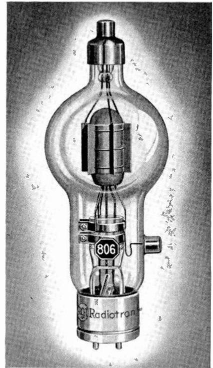
RCA-806 is designed for hard use as a high-power r-f amplifier and class B modulator. A single tube in class C telegraph service can take an input of 1000 watts and requires only 34 watts of driving power! Maximum plate dissipation of the tube is 225 watts (ICAS).
