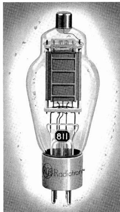
RCA-811 is a husky high-mu triode having a maximum plate-dissipation rating of 55 watts (ICAS). With a mu of 160, this tube requires no bias in class B modulator service up to a plate voltage of 1250 volts—and only -4.5 to -9 volts of bias up to 1500 volts.
