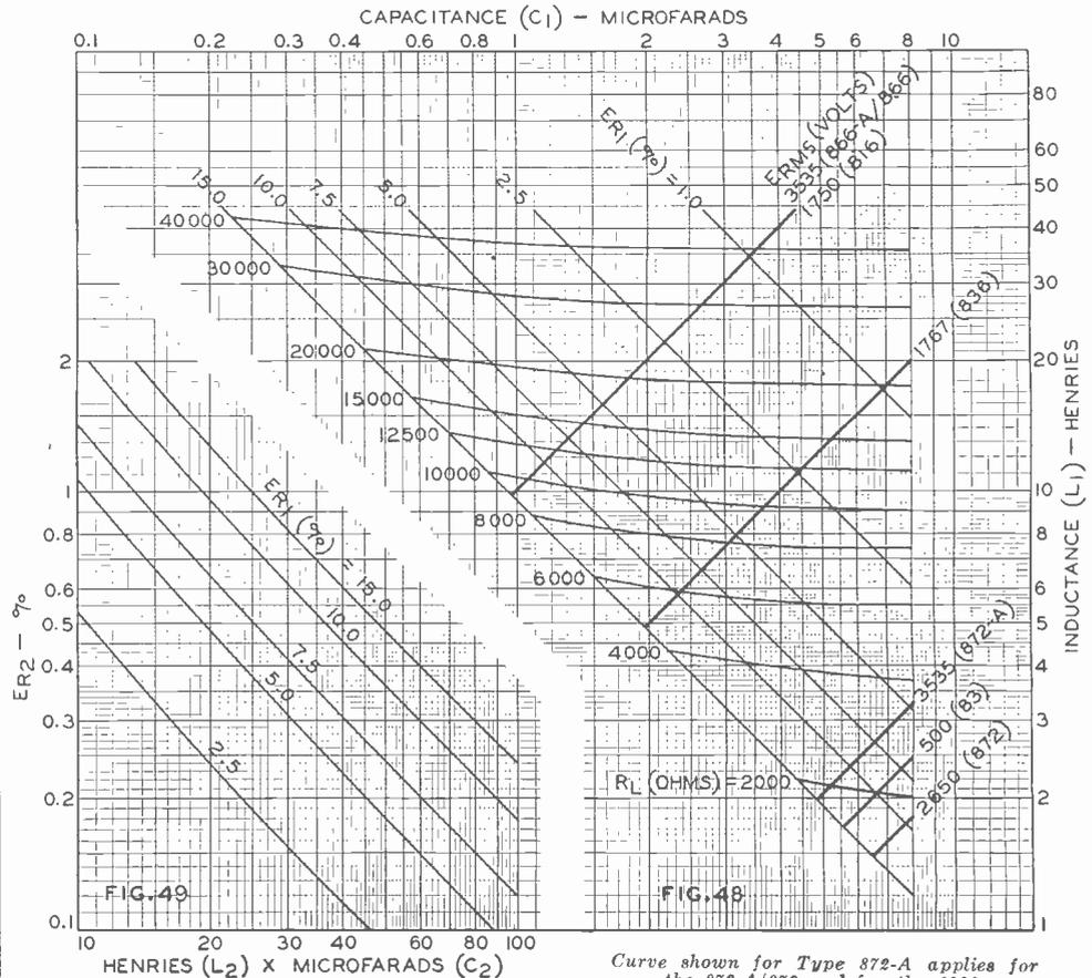
ing two type 866-A/866's, design a double-section filter which will limit the output ripple voltage to 0.5% at a load current equal to the combined maximum d-c load-current rating of the tubes (500 ma.) and still prevent the peak plate current of either tube from rising higher than its maximum peak plate-current rating. The input choke is to be of the swinging type and the voltage regulation is to be good from no-load to full load.
