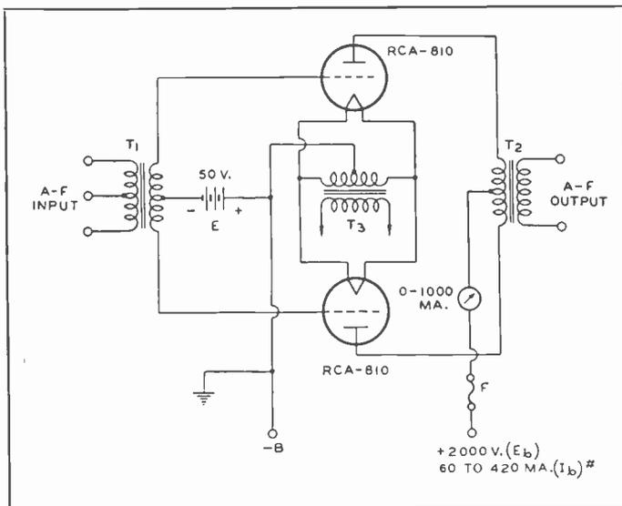
$T_1$ =Input transformer; plate-to-plate impedance, 1500 ohms (Note 2)  $T_3$ =c.t. filament transformer
