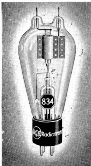
RCA-834 is a transmitting triode designed particularly for use as an r-f amplifier and oscillator at the ultra-high frequencies. It has a maximum plate-dissipation rating of 50 watts (CCS) and can be used with maximum ratings at frequencies up to 100 Mc! It may be operated at reduced input up to 350 Mc! RCA-834 is conservatively rated at 125 watts input for class C telegraph service and 100 watts for plate-modulated service.
