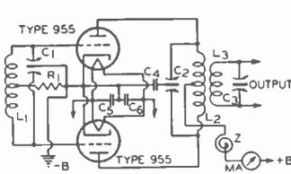
L<sub>1</sub> C<sub>1</sub>, L<sub>2</sub> C<sub>2</sub>—Depend on frequency range desired
