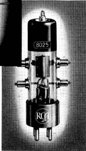
RCA-8012 and RCA-8025 are uhf triodes designed for use as oscillators, r-f power amplifiers, and frequency multipliers. The 8025 is similar to the 8012 but the grid and plate terminals are equipped with miniature caps and the filament connections are made to a small 4-pin Micanol base. The 8012 supersedes the 1628.
