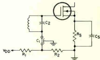
Fig. 6. Circuit used to eliminate input-circuit loading.
