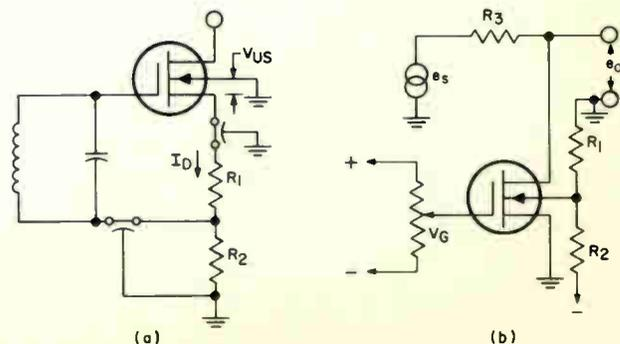
Fig. 7. Substrate biasing circuits.
