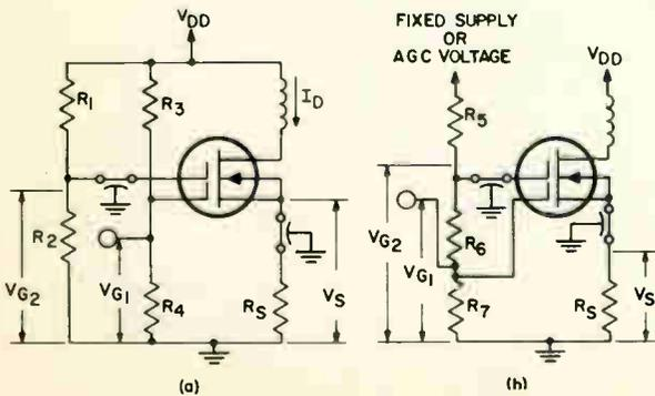
Fig. 12. Typical biasing circuits for the 3N140.
