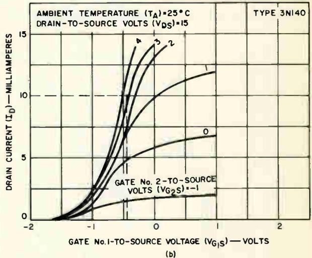
Fig. 11. Characteristics curves for the 3N140.
