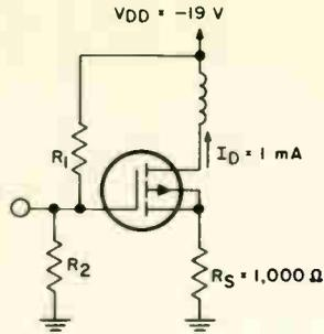
Fig. 8. Biasing circuit for an enhancement-type MOS transistor.
