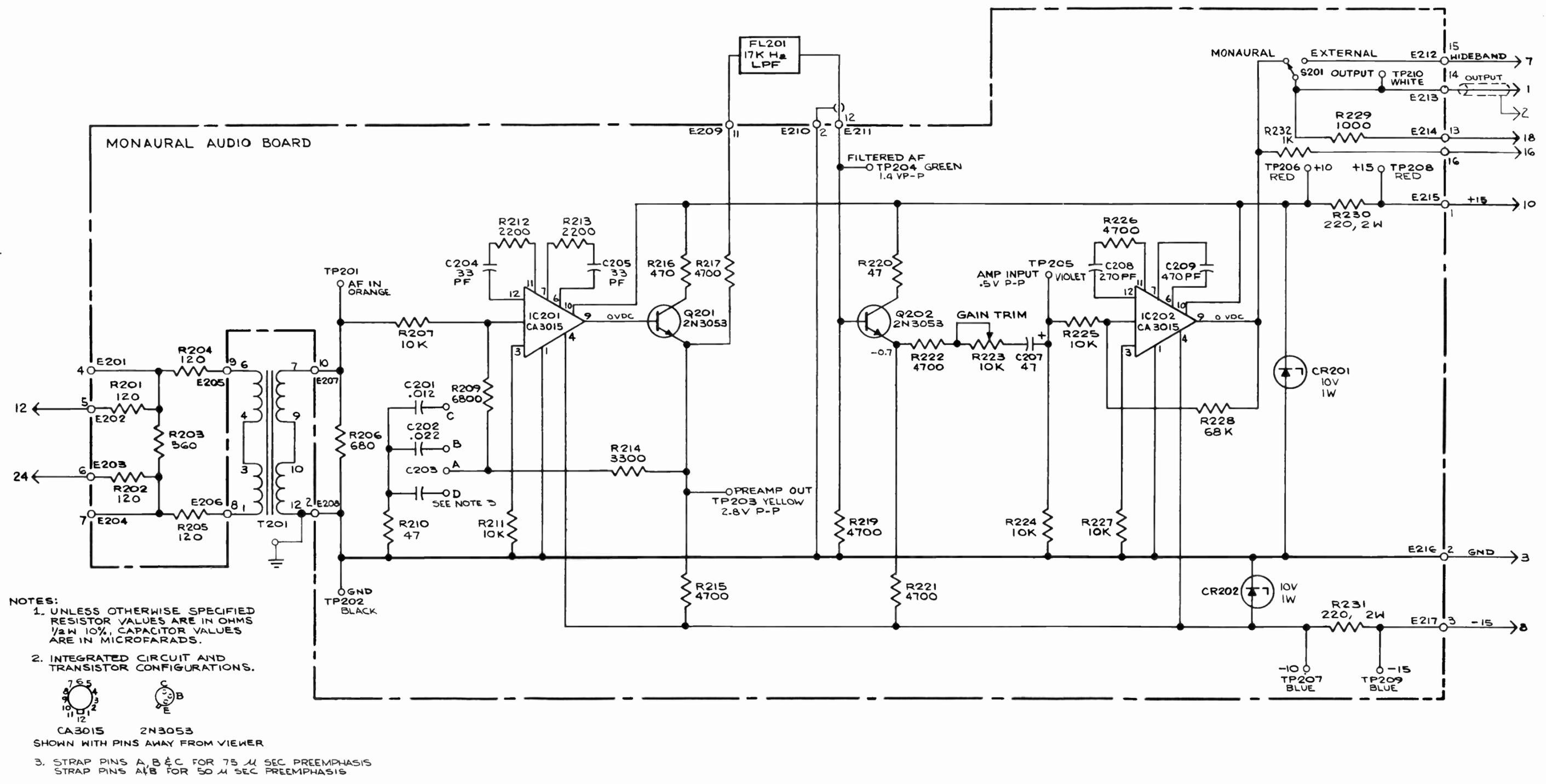
Figure 53. Monaural Audio Module, Schematic Diagram
