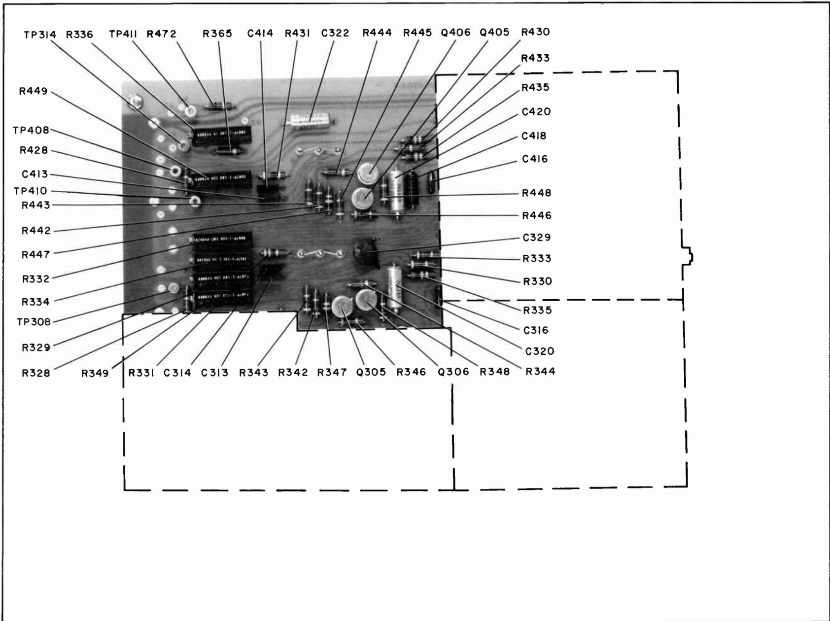
Figure 32. Stereo Generator Board, Parts Location
