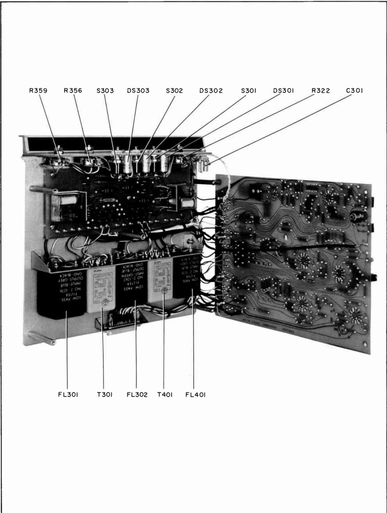
Figure 29. Stereo Generator Board, Parts Location
