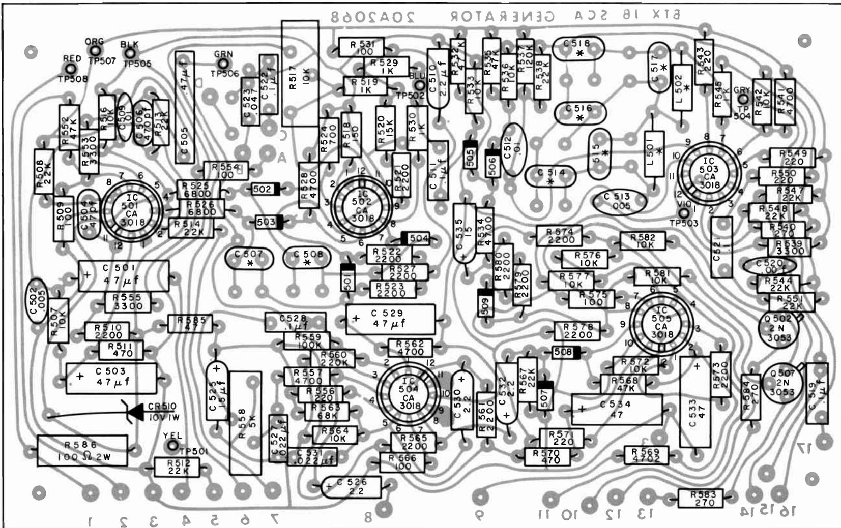
Figure 44. SCA Generator Board, Parts Overlay, Top
