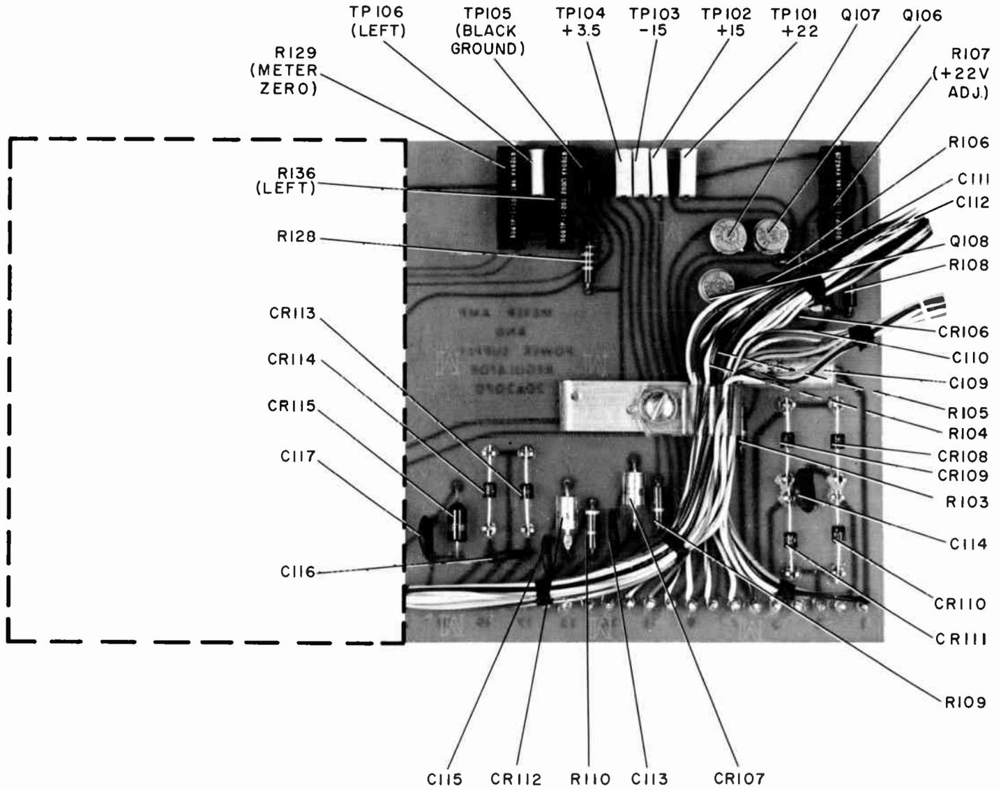
Figure 15. Main Frame Metering Amplifier Board, Parts Location
