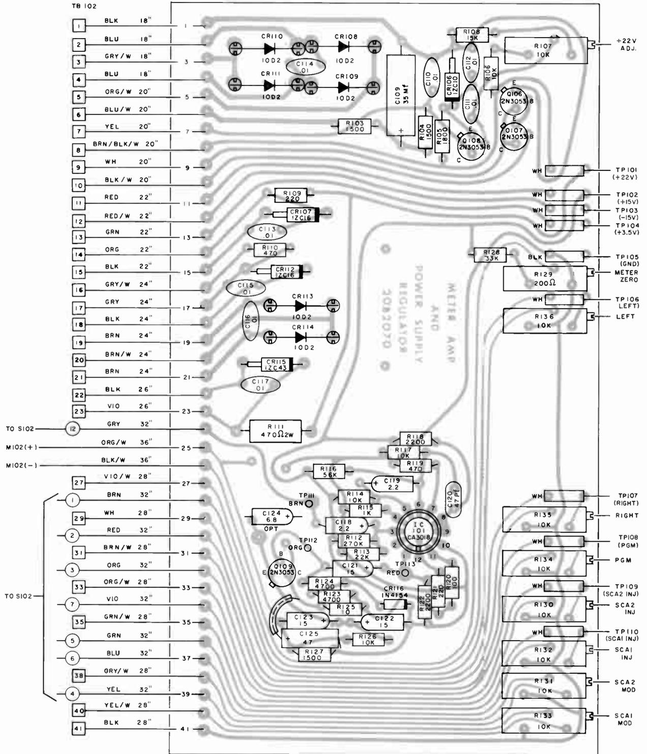
Figure 17. Main Frame Metering Amplifier Board, Parts Overlay, Bottom
