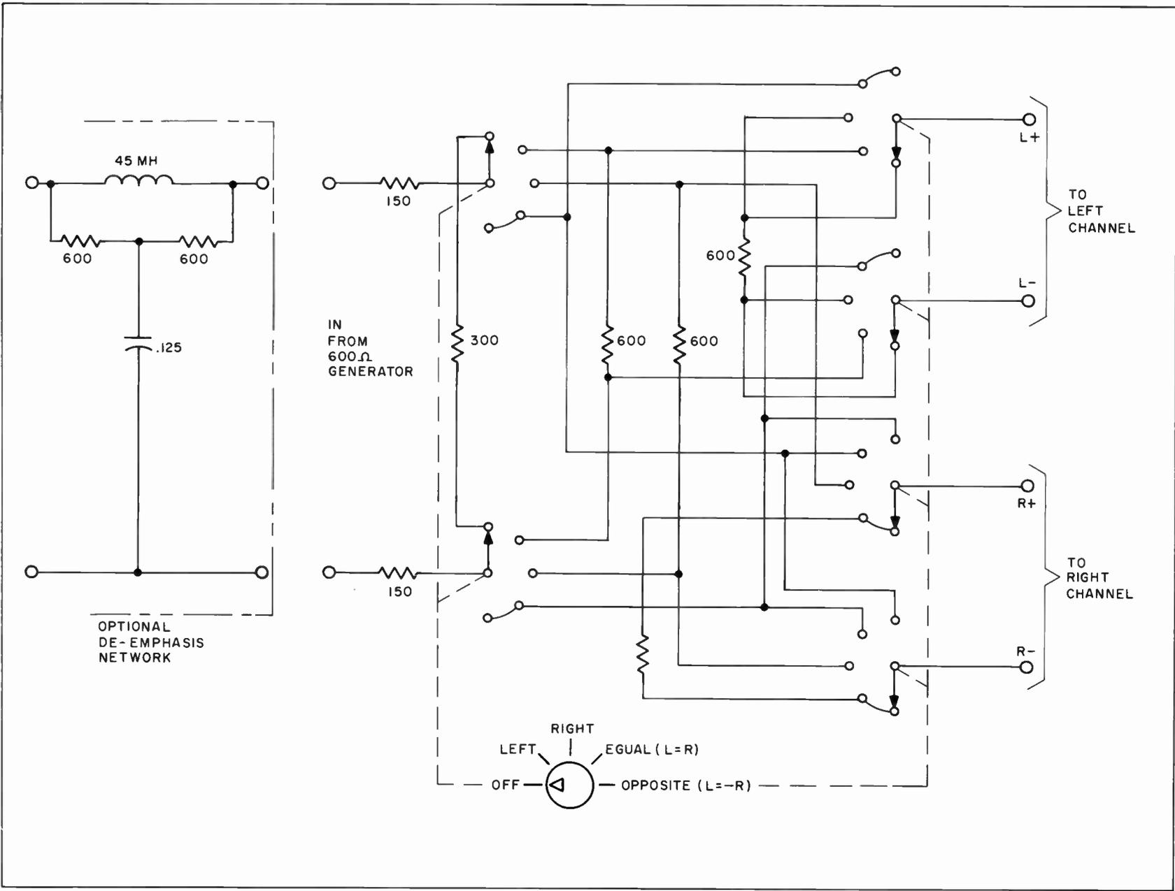
Figure 57. BTX-1B Low-Pass Filter Installation
