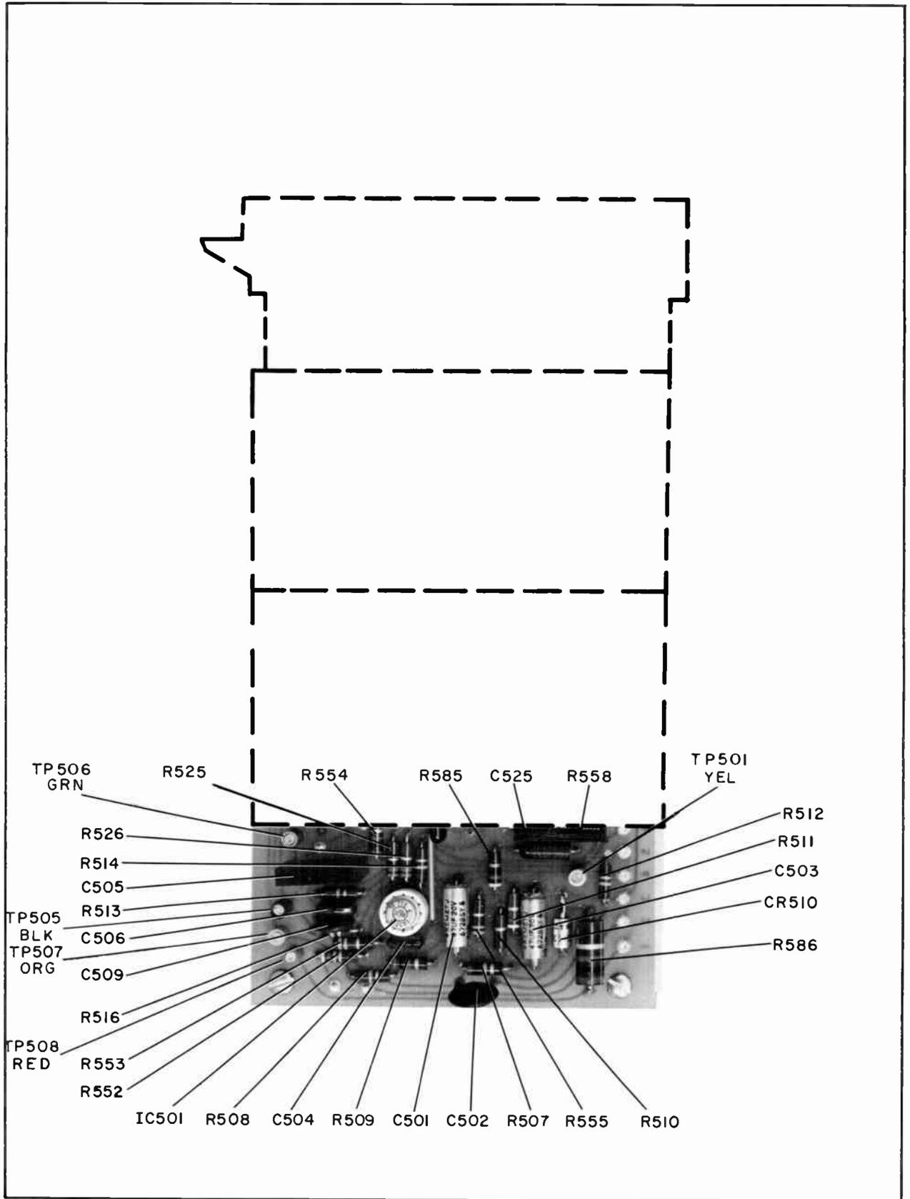
Figure 43. SCA Generator Board, Parts Location
