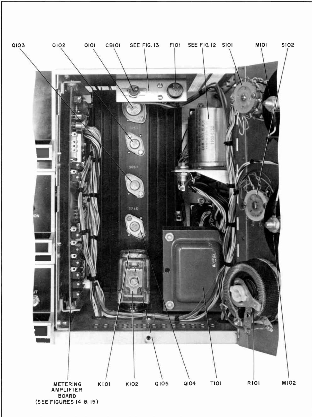
Figure 11. Main Frame, Parts Location
