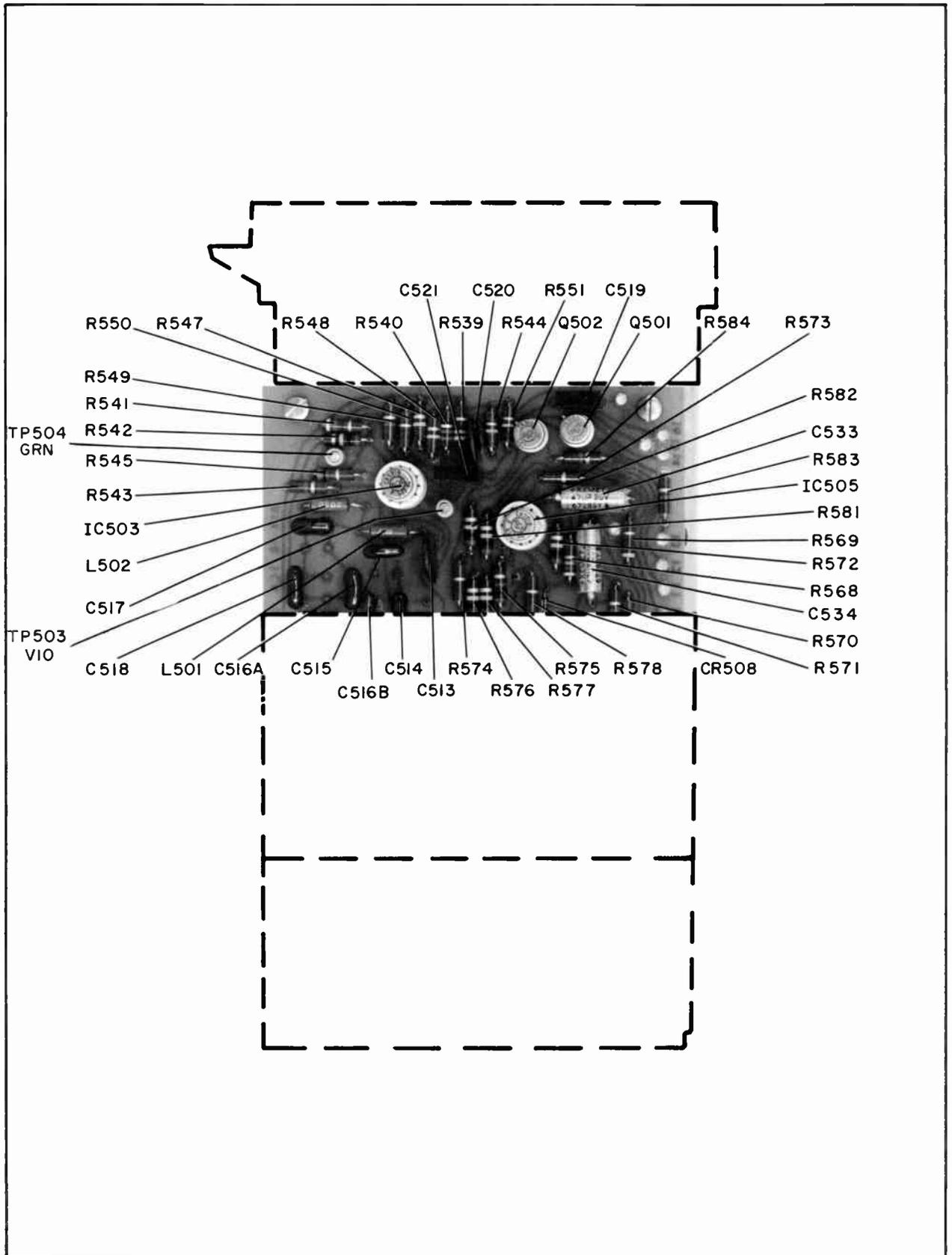
Figure 41. SCA Generator Board, Parts Location
