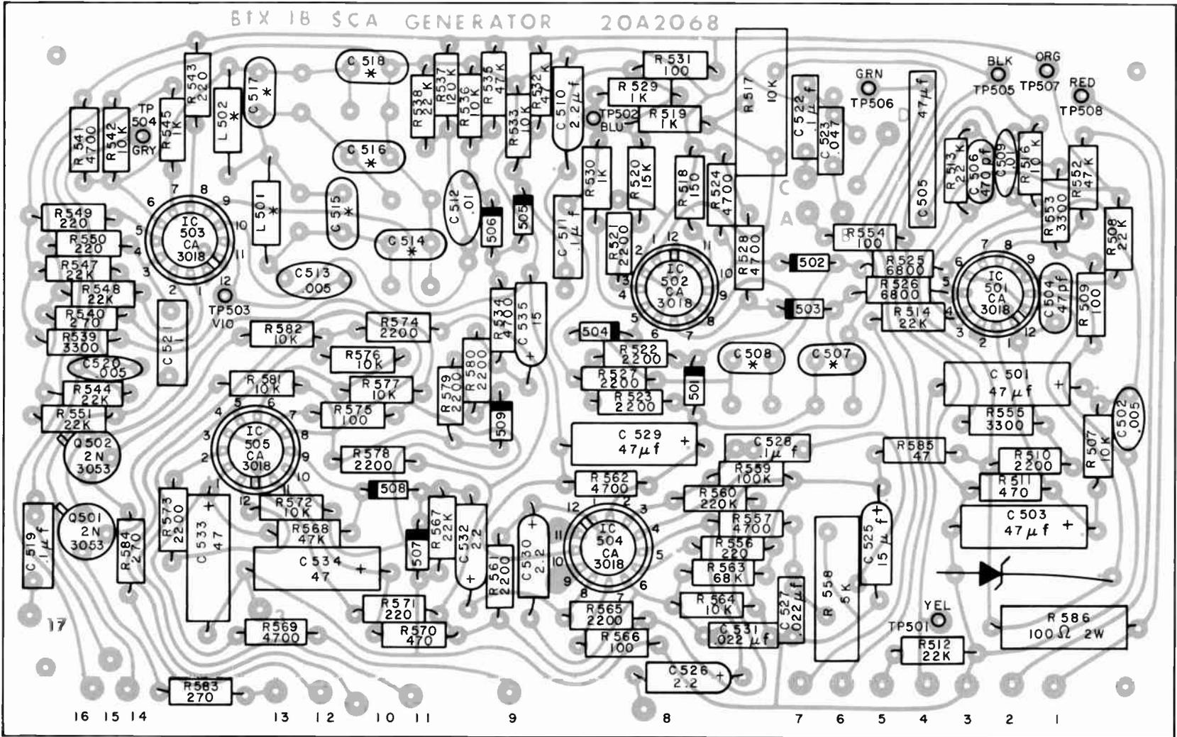
Figure 45. SCA Generator Board, Parts Overlay
