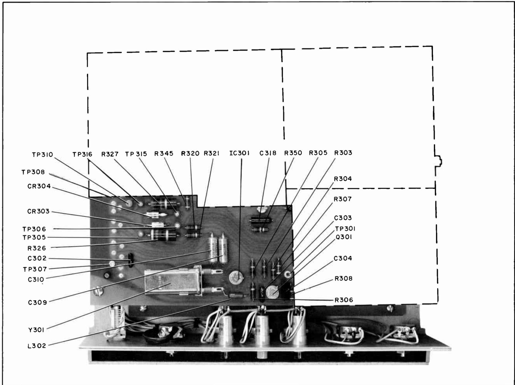
Figure 30. Stereo Generator Board, Parts Location
