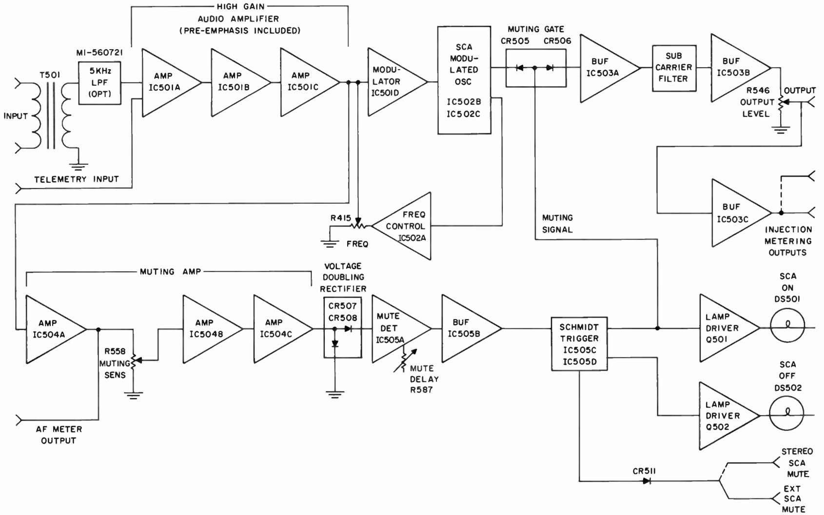
Figure 5. BTX-1B SCA Generator, Simplified Block Diagram
