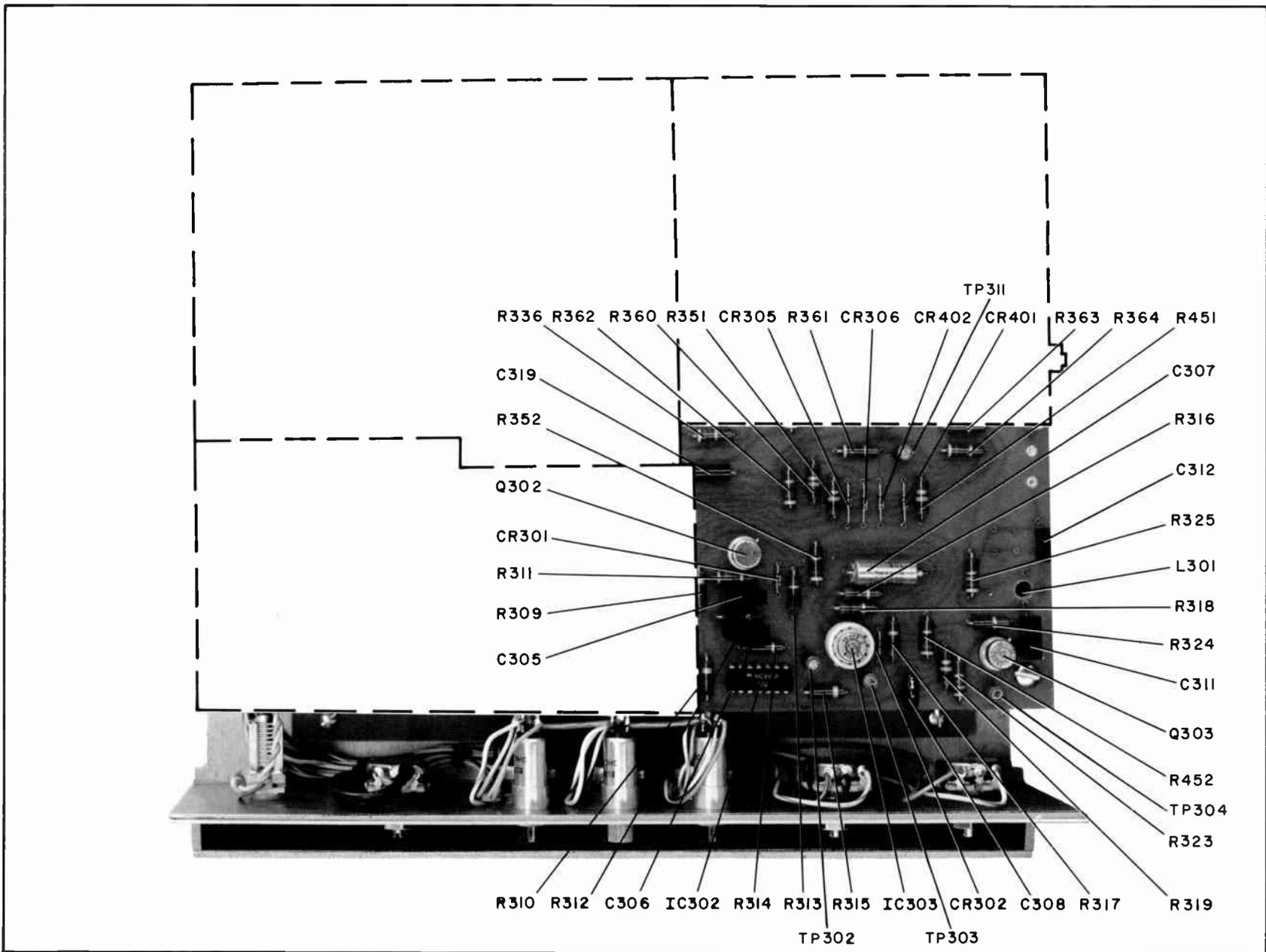
Figure 33. Stereo Generator Sub-Board, Parts Location
