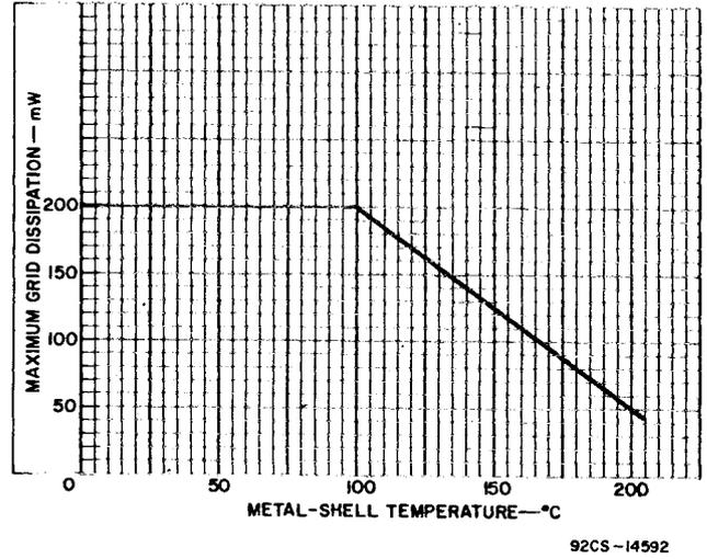
Fig. 22 - Grid-dissipation rating chart, dev. type A15526.
