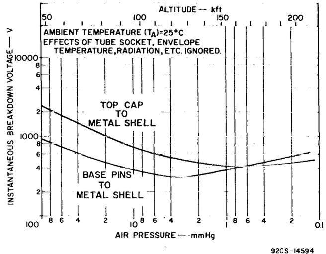
Fig. 6 - Breakdown-voltage characteristics, type 8627 and dev. type A15526.
