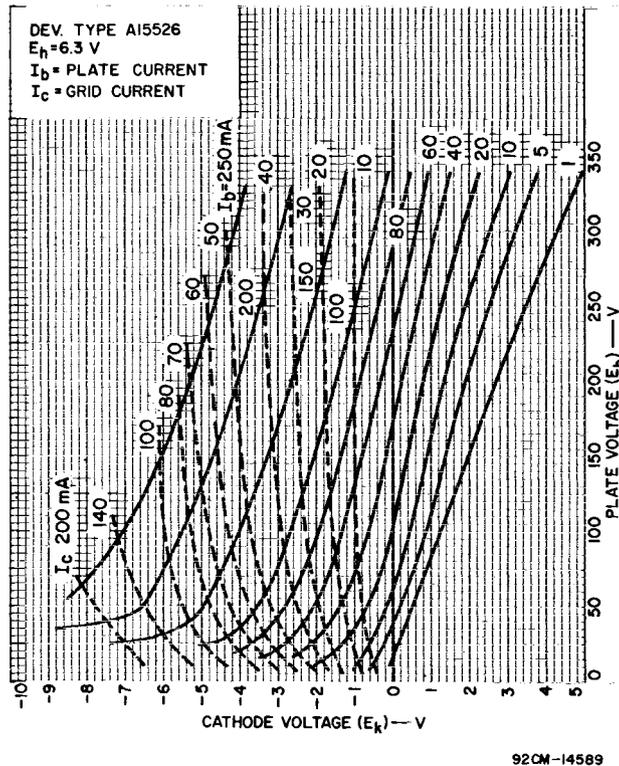
Fig.20 - Typical grounded-grid constant-current characteristics, dev. type A15526.
