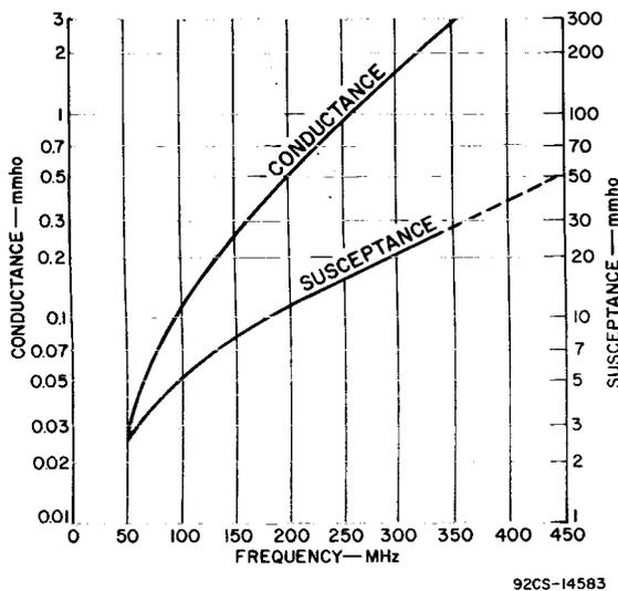
Fig.33 - Typical values of conductance and susceptance as functions of frequency, types 7586, 7895, and 8056.
