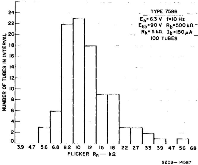
Fig. 27 - Equivalent flicker noise resistance at 10 Hz, type 7586.
