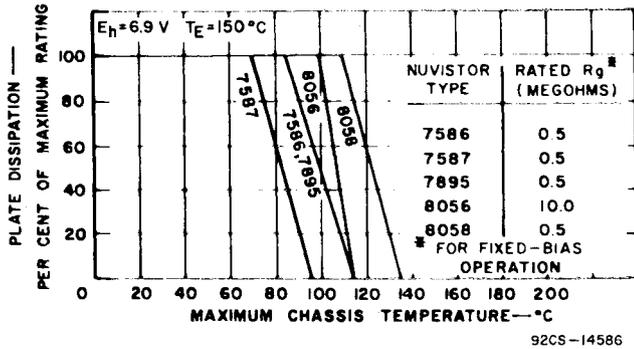
Fig. 4 - Combinations of plate dissipation and chassis temperature for metal-shell temperature of  $150^{\circ}\text{C}$ .
