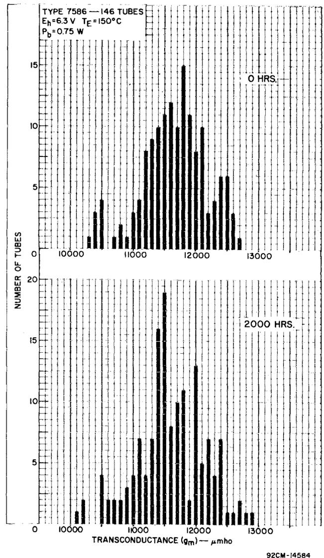
**Fig. 2 - Transconductance at 0 and 2000 hours, type 7586.**
