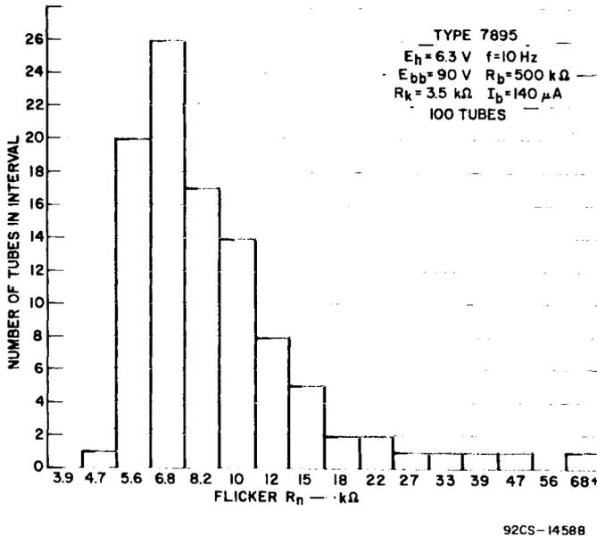
Fig. 28 - Equivalent flicker noise resistance at 10 Hz, type 7895.
