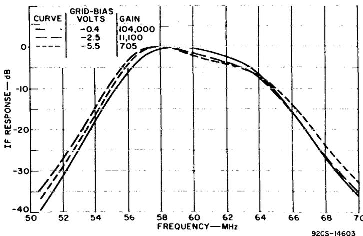
Fig. 14 - Gain-bandpass characteristics of a 5-stage, 60-MHz if amplifier utilizing type 7587.
