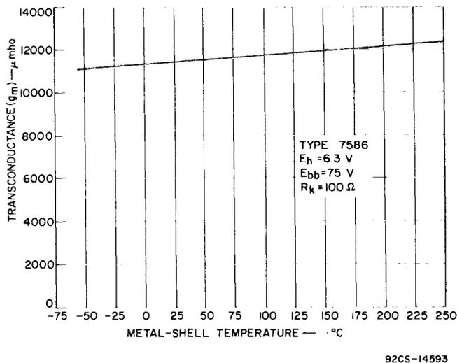
Fig. 5 - The effect of shell temperature on transconductance, type 7586.
