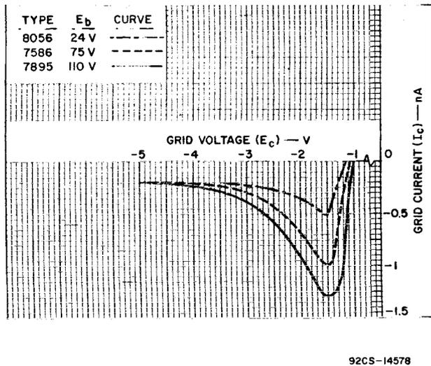
Fig.32 - Typical values of grid current as functions of grid voltage, types 7586, 7895, 8056.
