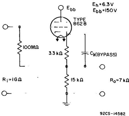
Fig.12 - High-input-impedance cathode-follower circuit, type 8628.
