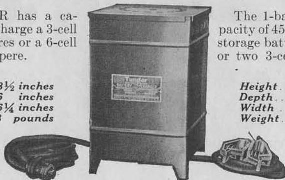
The 1-battery **TUNGAR** has a capacity of 45 watts and will charge a 3-cell storage battery at 5 amperes or a 6-cell, or two 3-cell, batteries at 3 amperes.
