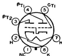
resistance, 4000 ohms; output watts, 3.8. This is a DISCONTINUED type listed for reference only.
