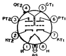
Glass lock-in type used as voltage amplifier or phase inverter in radio equipment. Outline 20, OUTLINES SECTION. Tube requires lock-in socket. Heater volts (ac/dc), 6.3; amperes, 0.6. For maximum ratings and typical operation of each triode unit, refer to metal type 6J5. The application of this type is similar to that of glass-octal type 6SN7-GT. Type 7N7 is used principally for renewal purposes.
