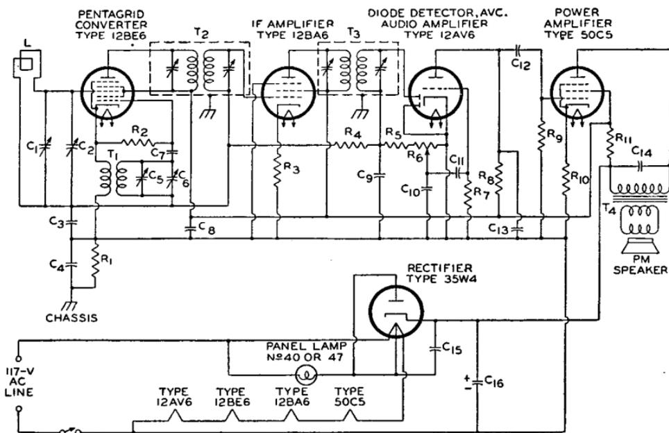
$C_1$   $C_5$  = Ganged tuning capacitors;  $C_1$ , 10-365  $\mu\text{f}$ ;  $C_5$ , 7-115  $\mu\text{f}$
