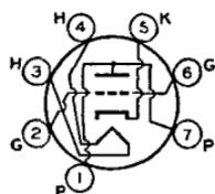
SECTION. Tubes require miniature seven-contact socket and may be mounted in any position. Type 6AF4 is a DISCONTINUED type listed for reference only.
