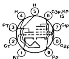
agc amplifier, or reactance tube. The triode unit is used in low-frequency oscillator, sync-separator, sync-clipper, and phase-splitter circuits. Outline 14, OUTLINES SECTION. Heater volts (ac/dc), 8.4; amperes, 0.45; warm-up time (average), 11 seconds. For definition of heater warm-up time and method for determining it, see type 6CG7. Except for heater rating, type 8AW8-A is identical with miniature type 6AW8-A.
