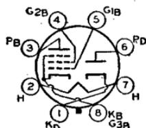
90; grid-No.1 volts, -7; plate ma., 27; grid-No.2 ma., 2; plate resistance, 17000 ohms; transconductance, 4800  $\mu$ mhos; load resistance, 2600 ohms; maximum-signal output watts, 1.0. This is a **DISCONTINUED** type listed for reference only.
