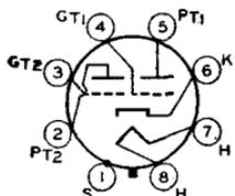
Metal type used as phase inverter or voltage amplifier in ac/dc radio equipment. Outline 3, OUTLINES SECTION. Heater volts (ac/dc), 12.6; amperes, 0.15. Except for heater rating, this type is identical with metal type 6SC7.
