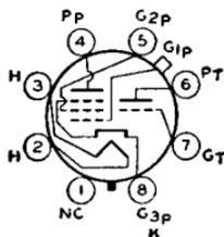
Glass octal type used as an amplifier. Outline 38, OUTLINES SECTION. Heater volts (ac/dc), 6.3; amperes, 0.3. Except for inter-electrode capacitances, this type is identical electrically with type 6F7. Type 6P7-G is a DISCONTINUED type listed for reference only.
