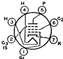
6SG7. The low value of grid-No.1-to-plate capacitance minimizes regenerative effects, while the high transconductance makes possible high signal-to-noise ratio.
