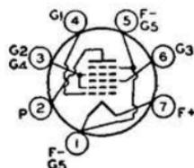
Miniature type used in lightweight, portable, compact, battery-operated receivers. Outline 11, OUTLINES SECTION. Tube requires miniature seven-contact socket and may be mounted in
