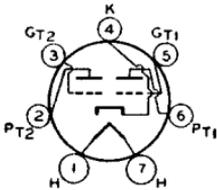
Glass type used as class A<sub>1</sub> amplifier in either push-pull or parallel circuits. Outline 42, OUTLINES SECTION. Heater volts (ac/dc), 6.3; amperes, 0.6. With plate volts of 250 and grid volts of -27.5, characteristics for each unit are: plate ma., 18; plate resistance, 3500 ohms; transconductance, 1700 μmhos; amplification factor, 6. With plate-to-plate load resistance
