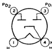
Glass type used in power supply of radio equipment having high dc requirements. Outline 42, OUTLINES SECTION. Tube requires four-contact socket. Heater volts (ac), 5.0; amperes, 2. This type is identical electrically with glass-octal type 5V4-G. Type 83-v is used principally for renewal purposes.
