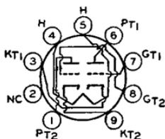
Heater volts (ac/dc), 8.4; amperes, 0.45; warm-up time (average), 11 seconds. For definition of heater warm-up time and method for determining it, see type 6CG7. Except for heater rating, type 8CM7 is identical with miniature type 6CM7.
