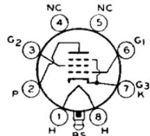
grid-No.2 ma., 5.5; plate resistance, 70000 ohms; transconductance, 3000  $\mu$ mhos; load resistance, 7500 ohms; output watts, 2.8. This is a DISCONTINUED type listed for reference only.
