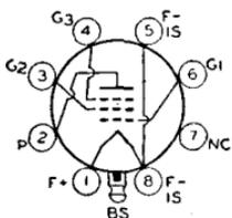
Glass lock-in type used as rf or if amplifier in battery-operated receivers. Outline 15, OUTLINES SECTION. Tube requires lock-in socket. Filament volts (dc), 1.4; amperes, 0.05. Typical operation as class A<sub>1</sub> amplifier: plate volts, 90 (110 max); grid-No.2 (screen-grid) volts, 45 max; grid-No.1 volts, 0; plate resistance (approx.), greater than 1 megohm; transconductance, 775  $\mu$ hos; plate ma., 1.15; grid-No.2 ma., 0.3. This type is used principally for renewal purposes.
