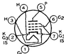
0.6; warm-up time (average), 11 seconds. For definition of heater warm-up time and method for determining it, see type 6CG7. Peak heater-cathode volts, 200 *max.* When the heater is positive with respect to the cathode, the dc component of the heater-cathode voltage must not exceed 100 volts. Except for heater and heater-cathode rating, type 3BC5 is identical with miniature type 6BC5.
