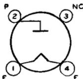
Glass type used in power supply of radio receivers. Maximum over-all length, 6-1/4 inches; maximum diameter, 2-7/16 inches. Tube requires four-contact socket and should be mounted preferably in a vertical position. Horizontal mounting is permissible if pins 1 and 4 are in a vertical plane. Filament volts (ac), 7.5; amperes,
