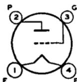
Glass type used in output stage of audio-frequency amplifiers. Outline 42, OUTLINES SECTION. Tube requires four-contact socket. Filament volts (ac/dc), 5.0; amperes, 0.25. Characteristics as class A<sub>1</sub> amplifier: plate volts, 180 max; grid volts, -40.5; cathode resistor, 2150 ohms; plate ma., 20; plate resistance, 1750 ohms; amplification factor, 3; transconductance,
