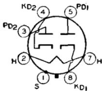
Metal type used as detector, low-voltage rectifier, or avc tube in ac/dc radio receivers. Outline 1, OUTLINES SECTION. Heater volts (ac/dc), 12.6; amperes, 0.15. Except for heater rating, this type is identical with metal type 6H6.
