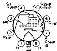
525  $\mu$ hos; plate ma., 1.8; grids-No.2-and-No.4 ma., 3.0. Typical operation of triode unit: plate supply volts, 250 (300 *max*) applied through a 20000-ohm dropping resistor bypassed by a 0.1- $\mu$ f capacitor; grid resistor, 50000 ohms; plate ma., 5.0; total cathode ma. (both units), 10.2. This is a **DISCONTINUED** type listed for reference only.
