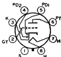
operation of triode unit as class A<sub>1</sub> amplifier: plate volts, 250 *max*; grid volts, -9; amplification factor, 16; plate resistance, 8500 ohms; transconductance, 1900  $\mu$ mhos; plate ma., 9.5; plate dissipation, 2.5 *max* watts; load resistance, 10000 ohms; power output, 300 milliwatts; peak heater-cathode volts, 90 *max*. For diode-operation curves, refer to type 6AV6. For heater and cathode considerations, refer to type 6AV6. Type 6SR7 is used principally for renewal purposes.
