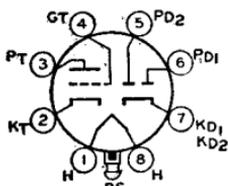
Glass lock-in type used as FM detector and audio amplifier in circuits which require diode and triode units with separate cathodes. Outline 15, OUTLINES SECTION. Tube requires lock-in socket. Heater volts (ac/dc), 6.3; amperes, 0.3. For ratings and typical operation, refer to glass-octal type 6AQ7-GT. Type 7K7 is used principally for renewal purposes.
