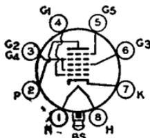
Glass lock-in type used as converter in superheterodyne circuits. Outline 15, OUTLINES SECTION. Tube requires lock-in socket. Heater volts (ac/dc), 6.3; amperes, 0.3. For maximum ratings, typical operation in converter service, and curves, refer to metal type 6SA7. Type 7Q7 is used principally for renewal purposes.
