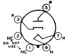
This type may be supplied with pin No.1 omitted. Tube requires octal socket and may be mounted in any position. It is especially important that this tube, like other power-handling tubes, be adequately ventilated. For curve of average plate characteristics, see page 64.
