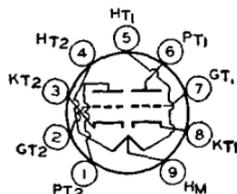
ing it, see type 6CG7. Peak heater-cathode volts, 200 max. When the heater is positive with respect to the cathode, the dc component of the heater-cathode voltage must not exceed 100 volts. Except for heater and heater-cathode ratings, type 6AU7 is identical with miniature type 12AU7. The 6AU7 is a DISCONTINUED type listed for reference only.
