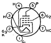
peak heater-cathode volts, 90 max. For heater and cathode considerations, refer to miniature type 6AQ5. Within its maximum ratings, type 6AR5 is equivalent in performance to glass-octal type 6K6-GT. Refer to type 6K6-GT for characteristic curves. Type 6AR5 is used principally for renewal purposes.
