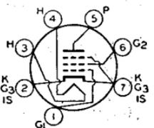
seven-contact socket and may be mounted in any position. Except for a slightly higher transconductance, this type is similar electrically to type 6AG5. Heater volts (ac/dc), 6.3; amperes, 0.3. For heater and cathode considerations, refer to type 6AV6.
