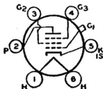
Glass type used in output stage of radio receivers. Outline 35, OUTLINES SECTION. Tube requires six-contact socket. Heater volts (ac/dc), 6.3; amperes, 0.4. Maximum ratings as class B amplifier (triode connection): plate volts, 250 *max*; peak plate ma. per tube, 90 *max*; average grid input of grids No.1 and No.2 tied together, 0.35 *max* watt. This is a DISCONTINUED type listed for reference only.
