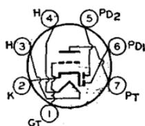
Miniature type used as combined detector, amplifier, and avc tube primarily in automobile radio receivers operating from a 12-volt storage battery. The triode unit is particularly
