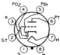
unit as class A<sub>1</sub> amplifier: plate volts, 250 *max*; plate dissipation, 2.5 *max* watts. For diode operation curves, refer to type 6AV6. Type 6ST7 is a DISCONTINUED type listed for reference only.
