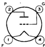
Glass type used as rf voltage amplifier in ac-operated receivers. Outline 42, OUTLINES SECTION. Tube requires four-contact socket. Filament volts (ac/dc), 1.5; amperes, 1.05. Typical operation as class A<sub>1</sub> amplifier: plate volts, 180 max; grid volts, -14.5, plate ma., 6.2; plate resistance, 7300 ohms; transconductance, 1150  $\mu$ mhos; amplification factor, 8.3. This is a DISCONTINUED type listed for reference only.
