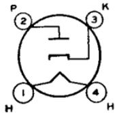
possible. Heater volts (ac/dc), 12.6; amperes, 0.3. Maximum ratings as half-wave rectifier: peak inverse plate volts, 700 *max*; peak plate ma., 330 *max*; dc output ma., 55 *max*; peak heater-cathode volts, 350 *max*. With typical operating ac plate voltages of 117, 150, and 235 volts rms, the minimum total effective plate-supply impedance required is 0, 30, and 75 ohms, respectively. This is a DISCONTINUED type listed for reference only.
