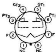
Glass octal types used in output stage of battery-operated receivers. Type 1J6-G, Outline 36; type 1J6-GT, Outline 27, OUTLINES SECTION. Tubes require octal socket. Filament volts (dc), 2.0; amperes, 0.24. Typical operation as class B power amplifier: plate volts, 135 max; peak plate ma. per plate, 50 max; grid volts, 0; zero-signal plate ma. per plate, 5; effective plate-to-plate load resistance, 10000
