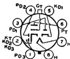
Glass octal type used as audio amplifier, AM detector, and FM detector in AM/FM receivers. Diode unit No.2 is used for AM detection, and diode units No.1 and No.3 are used for FM detection. The grid of the high-mu triode is brought out to a top cap. Outline 28, OUTLINES SECTION. Tube requires octal socket and may be mounted in any position. For
