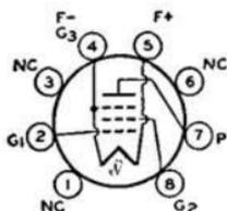
Subminiature type used in output stage of small, compact, battery-operated receivers for the standard AM broadcast band. Outline 8, OUTLINES SECTION. Tube requires subminiature eight-contact socket and may be mounted in any position. Base pins should not be soldered to circuit elements because heat of soldering operation may crack the glass seal. Filament volts (dc), 1.25; amperes, 0.04. The
