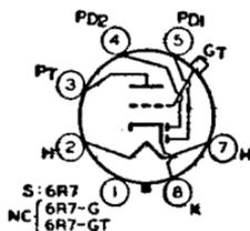
Metal type 6R7 and glass-octal types 6R7-G and 6R7-GT used as combined-detector, amplifier, and avc tubes. Outlines 4, 38, and 21, respectively, OUTLINES SECTION. Type 6R7-GT may be supplied with pin No.1 omitted. Tubes require octal sockets. Within their maximum ratings, these types are identical electrically with type 6BF6 except for capacitances. Maximum ratings of triode unit as class
