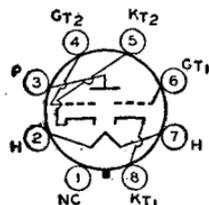
Glass octal type used as a voltage amplifier or as a driver for two type 6AC5-GT tubes in dynamic-coupled, push-pull amplifiers. In the latter service, type 6AE7-GT replaces two tubes ordinarily required as drivers. Outline 23, OUTLINES SECTION. Heater volts (ac/dc), 6.3; amperes, 0.5. This is a DISCONTINUED type listed for reference only.
