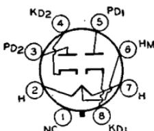
For maximum ratings and typical operation as half-wave rectifier or voltage doubler without panel lamp, refer to glass octal type 25Z6-GT. When operated with a panel lamp and 250-ohm panel-lamp shunting resistor, ratings and typical operation are the same as for type 25Z6-GT, except that dc output current per plate is 65 ma. Type 50Y7-GT is used principally for renewal purposes.
