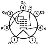
Glass type used in rf and if stages of radio receiver employing avc. Outline 44, OUTLINES SECTION. Except for interelectrode capacitances, this type is identical electrically with type 6U7-G. Heater volts (ac/dc), 6.3; amperes, 0.3. This is a DISCONTINUED type listed for reference only.
