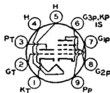
ifier, or an agc amplifier. The triode unit is used in sync-amplifier, sync-separator, sync-clipper, and phase-inverter circuits. Outline 14, OUTLINES SECTION. Tube requires miniature nine-contact socket and may be mounted in any position.
