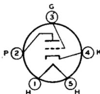
Glass type used as detector or class A<sub>1</sub> amplifier in radio receivers. Outline 35, OUTLINES SECTION. Heater volts (ac/dc), 3; amperes, 1.25. Characteristics: plate volts, 180; grid volts, -9; amplification factor, 12.5; plate resistance, 8900 ohms; transconductance, 1400  $\mu$ mhos; plate ma., 5.8. This is a DISCONTINUED type listed for reference only.
