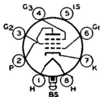
max watt; grid No.1 volts, -3; grid No.3 connected to cathode at socket; plate resistance, greater than 1 megohm; transconductance, 1575  $\mu$ mhos; plate ma., 2.2; grid-No.2 ma., 0.7. Within the limits of its maximum ratings, this type is similar in performance to metal types 6SJ7 and 12SJ7. Type 14C7 is used principally for renewal purposes.
