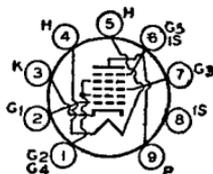
and may be mounted in any position. Its characteristics are similar to those of metal type 6SB7-Y. For heater and cathode considerations, refer to type 6AV6.
