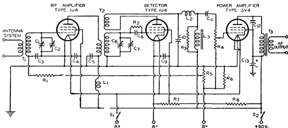
**C<sub>1</sub> C<sub>6</sub>**=Ganged band-setting capacitors, 140  $\mu\mu\text{f}$ , maximum per section
