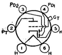
Glass type used as a combined detector, amplifier, and avc tube. Outline 39, OUTLINES SECTION. Tube requires six-contact socket. Heater volts (ac/dc), 6.3; amperes, 0.3. Characteristics of triode unit as class A<sub>1</sub> amplifier: plate volts, 250 *max*; grid volts, -20; amplification factor, 8.3; transconductance, 1100  $\mu$ mhos; pplate ma., 8.0; plate resistance, 7500 ohms; load
