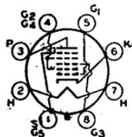
Metal type 6SA7 and glass-octal type 6SA7-GT used as converters in superheterodyne circuits. They are similar in performance to type 6BE6. For general discussion of pentagrid types, see *Frequency Conversion in ELECTRON TUBE APPLICATIONS SECTION*. Both tubes have excellent frequency stability. Type 6SA7-GT is used principally for renewal purposes.
