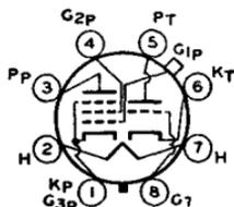
ductance, 2000  $\mu$ mhos, grid-No.1 volts for transconductance of 2  $\mu$ mhos, -41. Triode unit: plate volts, 100; grid volts, -1; plate ma., 0.6; amplification factor, 112; plate resistance, 75000; transconductance, 1500  $\mu$ mhos. This is a DISCONTINUED type listed for reference only.
