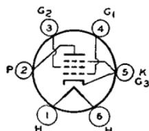
Glass type used in audio output stage of ac receivers. Outline 42, OUTLINES SECTION. Tube requires six-contact socket. Heater volts (ac/dc), 6.3; amperes, 0.7. This type is electrically identical with type 6F6. Type 42 is used principally for renewal purposes.
