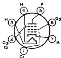
125 *max*; plate dissipation, 3 *max* watts; grid-No.2 input, 0.65 *max* watt; total cathode ma., 14 *max*; peak heater-cathode volts, 90 *max*. Type 6BD6 is used principally for renewal purposes.
