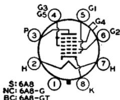
Metal type 6A8 and glass octal types 6A8-G and 6A8-GT used in superheterodyne circuits. 6A8 Outline 4, 6A8-G Outline 38, 6A8-GT Outline 24, OUTLINES SECTION. Tubes require octal socket. Heater volts (ac/dc), 6.3; amperes, 0.3. For heater and cathode considerations, refer to type 6AV6. Maximum ratings: plate, grids-No.3-and-No.5-supply, and grid-No.2-supply volts, 300 *max*; grids-No.3-and-
