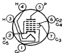
Miniature type used as a gated amplifier in color television receivers. In such service, it may be used as a combined sync separator and sync clipper. Outline 11, OUTLINES SEC-
