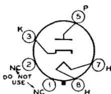
strings. Outline 22, OUTLINES SECTION. Tubes require octal socket and may be mounted in any position. These types may be supplied with pin No.1 omitted. Heater volts (ac/dc), 12.6; amperes, 0.6; warm-up time (average) for 12AX4-GTA, 11 seconds. For definition of heater warm-up time and method for determining it, see type 6CG7. Except for heater rating, these types are identical with glass octal type 6AX4-GT. Type 12AX4-GT is a DISCONTINUED type listed for reference only.
