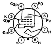
Metal type used as combined rf or if amplifier and detector or avc tube in radio receivers. Also used as resistance-coupled af amplifier. Outline 3, OUTLINES SECTION. Tube requires octal socket and may be mounted in any position. Heater volts (ac/dc), 6.3; amperes, 0.3. For heater and cathode considerations, refer to type 6AV6. For typical operation as a re-
