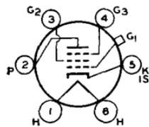
Glass type used in rf and if stages of radio receivers employing avc and as a mixer in superheterodyne circuits. Outline 44, OUTLINES SECTION. Tube requires six-contact socket. Heater volts (ac/dc), 2.5; amperes, 1.0. Except for heater ratings, this type is electrically identical with glass-octal type 6U7-G. Type 58 is a DISCONTINUED type listed for reference only.
