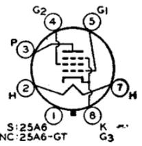
volts, 160; grid-No.2 volts, 135; plate dissipation, 5.3 watts; grid-No.2 input, 1.9 watts. These are DISCONTINUED types listed for reference only.
