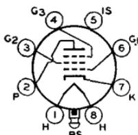
Glass lock-in type used as rf amplifier in high-frequency and wide-band applications. Outline 15, OUTLINES SECTION. Tube requires lock-in socket. Heater volts (ac/dc), 6.3; amperes, 0.15. Maximum ratings and characteristics as class A<sub>1</sub> amplifier: plate and grid-No.2 volts, 250 (300 *max*); plate dissipation, 2 *max* watts; grid-No.2 input, 0.7 *max* watt; cathode resistor, 250 ohms; grid No.3 and internal shield
