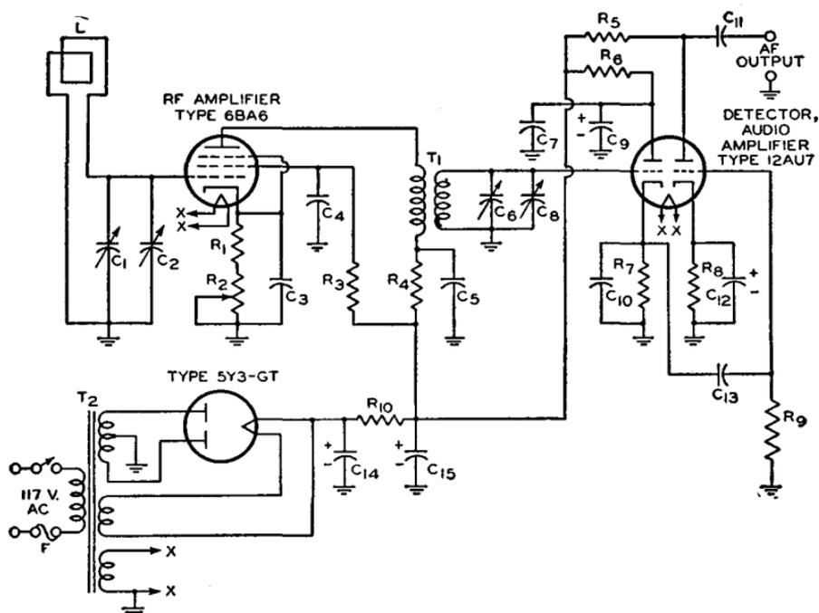
C<sub>1</sub> C<sub>6</sub>=Ganged tuning capacitors, 10-365  $\mu$ f
