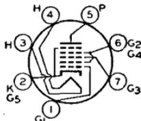
this type should be designed so that 90 per cent of the maximum values of plate voltage, grid-No.2 voltage, plate dissipation, and grid-No.2 input is never exceeded for a battery potential of 13.2 volts. Tube requires miniature seven-contact socket and may be mounted in any position.
