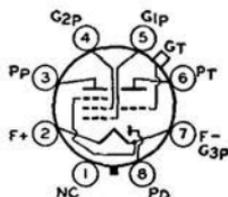
transconductance, 925  $\mu$ hos; load resistance, 12000 ohms; total harmonic distortion, 10 per cent; power output, 200 milliwatts. Characteristics of triode unit as class A<sub>1</sub> amplifier: plate volts, 90 (110 max); grid volts, 0; amplification factor, 25; plate resistance (approx.), 43500 ohms; transconductance, 575  $\mu$ hos; plate ma., 1.1. This is a DISCONTINUED type listed for reference only.
