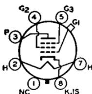
(300 *max*); grid-No.2 supply volts, 300 *max*; grid-No.2 volts, 100; grid No.3 connected to cathode at socket; grid-No.1 volts, -3; plate resistance (approx.), 0.8 megohm; transconductance, 1600  $\mu$ mhos; plate ma., 8.2; grid-No.2 ma., 2; plate dissipation, 2.25 *max* watts; grid-No.2 input, 0.25 *max* watt. This is a DISCONTINUED type listed for reference only.
