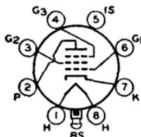
Glass lock-in type used as rf amplifier in ac/dc receivers or in mobile equipment where low heater-current drain is important. Outline 15, OUTLINES SECTION. Tube requires lock-in socket. Heater volts (ac/dc), 6.3; amperes, 0.15. Maximum ratings and characteristics as class A<sub>1</sub> amplifier: plate and grid-No.2 volts, 250 (300 *max*); plate dissipation, 2 *max* watts; grid-No.2 input, 0.75 *max* watt; grid
