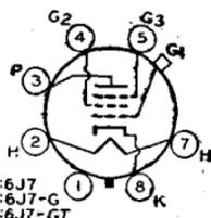
**SECTION.** Type 6J7-GT is used principally for renewal purposes. Type 6J7-G is a **DISCONTINUED** type listed for reference only. All types require octal socket and may be mounted in any position. For typical operation as resistance-coupled amplifiers, refer to Charts 11 and 14, **RESISTANCE-COUPLED AMPLIFIER SECTION.** For heater and cathode considerations, refer to type 6AV6.
