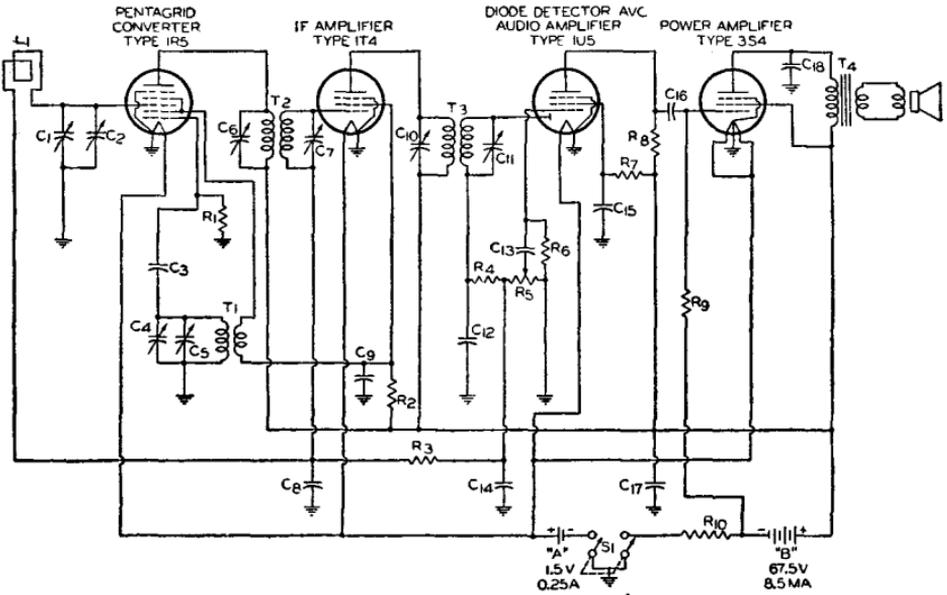
$C_1 C_4$  = Ganged tuning capacitors:  $C_1$ , 10-274  $\mu\text{mf}$ ;  $C_4$ , 7.5-122.5  $\mu\text{mf}$
