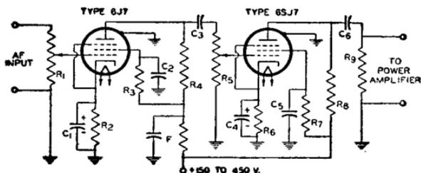
$C_1$   $C_4$  = 8  $\mu$ f, electrolytic, 25 v.
