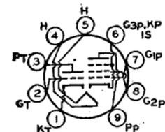
Miniature type used in a wide variety of applications in television receivers employing series-connected heater strings. The pentode unit is used as an if amplifier, a video amplifier, or an agc amplifier. The triode unit is used in low-frequency oscillator circuits. Outline 14, OUTLINES SECTION. Tube requires miniature nine-contact socket and may be mounted in any position.
