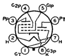
dissipation, 8.5 *max* watts; grid-No.2 input, 2.7 *max* watts. Maximum ratings of triode unit as class A<sub>1</sub> amplifier: plate volts, 285 *max*; plate dissipation, 1.0 *max* watt. This type is used principally for renewal purposes.
