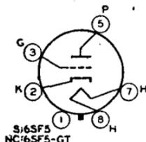
Metal type 6SF5 and glass-octal type 6SF5-GT are used in resistance-coupled amplifier circuits. Outlines 3 and 23, respectively, OUTLINES SECTION. Type 6SF5-GT may be supplied with pin No.1 omitted. Tubes require octal socket and may be mounted in any position. Characteristics, application, and references under type 6F5 apply to types 6SF5 and 6SF5-GT. Heater volts (ac/dc), 6.3; amperes, 0.3. Type 6SF5-GT is used principally for renewal purposes.
