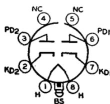
Lock-in type used as half-wave rectifier or voltage doubler in ac/dc receivers. Outline 20, OUTLINES SECTION. Tube requires lock-in socket. Heater volts (ac/dc), 50; amperes, 0.15. This type is electrically identical with glass-octal type 50Y6-GT and, except for heater rating, with glass-octal type 25Z6-GT. Refer to type 25Z6-GT for maximum ratings, typical operation, and curves. Type 50X6 is used principally for renewal purposes.
