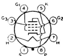
grid-No.2 volts, 100; grid-No.1 volts, -3; grid No.3 connected to cathode at socket; plate resistance (approx.), 1 megohm; transconductance, 1850  $\mu$ mhos; plate ma., 9; grid-No.2 ma., 2; plate dissipation, 2.25 *max* watts; grid-No.2 input, 0.35 *max* watts. Type 6SS7 is used principally for renewal purposes.
