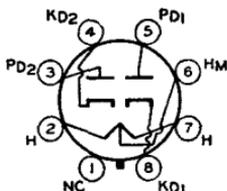
between pins 2 and 7), 2. Maximum ratings as rectifier or doubler: peak inverse plate volts, 700 max; peak plate ma. per plate, 400 max; dc output ma. per plate with panel lamp, 65 max; peak heater-cathode volts, 350 max; panel lamp section volts (pins 6 and 7), 2.5 max. This is a DISCONTINUED type listed for reference only.
