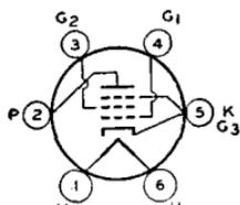
Glass type used in output stage of radio receivers. Outline 34 or 35, OUTLINES SECTION. Tube requires six-contact socket. Heater volts (ac/dc), 6.3; amperes, 0.4. This type is electrically identical with type 6K6-GT. Type 41 is used principally for renewal purposes.
