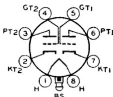
Glass lock-in type used as voltage amplifier or phase inverter in radio equipment. Outline 15, OUTLINES SECTION. Tube requires lock-in socket. Heater volts (ac/dc), 6.3; amperes, 0.3. Ratings and characteristics as class A<sub>1</sub> amplifier (each section): plate volts, 250 (300 *max*); cathode-bias resistor, 1100 ohms; plate ma., 9; transconductance, 2100  $\mu$ hos; amplification factor, 16; plate resistance, 7600 ohms. This type is used principally for renewal purposes.
