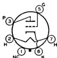
Glass octal type used as class A<sub>1</sub> amplifier in ac/dc radio receivers. Outline 23, OUTLINES SECTION. Heater volts (ac/dc), 6.3; amperes, 0.3. Maximum ratings as class A<sub>1</sub> amplifier: plate volts, 300 *max*; plate dissipation, 2.5 *max* watts. This is a DISCONTINUED type listed for reference only.
