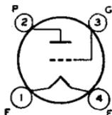
Glass type used as resistance-coupled or impedance-coupled amplifier in battery-operated receivers. Outline 42, OUTLINES SECTION. Filament volts (dc), 5; amperes, 0.25. Characteristics as class A<sub>1</sub> amplifier: plate-supply volts, 180; load resistance, 250000 ohms; grid volts, -3; plate ma., 0.2; plate resistance, 150000 ohms; amplification factor, 30; transconductance, 200  $\mu$ hos. This is a DISCONTINUED type listed for reference only.
