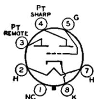
Glass octal type used as a control tube for twin-indicator type electron-ray tubes. Outline 36, OUTLINES SECTION. Contains two triodes with different cutoff characteristics. If avc voltage is applied to the common control grid in suitable circuit, one triode section operates on weak signals while the other operates on strong signals. Heater voltage (ac/dc), 6.3; amperes, 0.15. This is a DISCONTINUED type listed for reference only.
