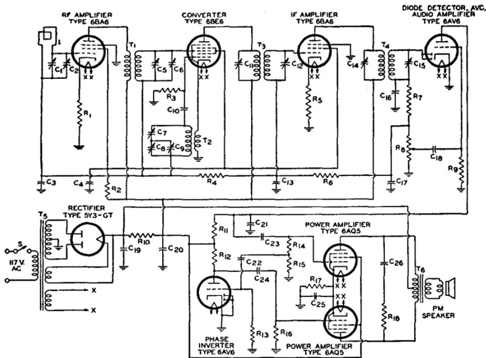
C<sub>1</sub> C<sub>5</sub> C<sub>8</sub>=Ganged tuning capacitors, 10-365  $\mu$ f
