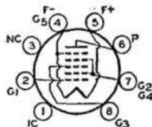
nected directly across a dry-cell battery rated at a terminal potential of 1.5 volts. Filament voltage should never exceed 1.6 volts. Maximum ratings: plate volts, 67.5 *max*; grids-No.2-and-No.4 (screen-grid) volts, 45 *max*; grids-No.2-and-No.4 supply volts, 67.5 *max*; total cathode ma., 4 *max*. This type is used principally for renewal purposes.
