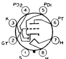
grid to plate, 1.1  $\mu$ f; input, 2.4  $\mu$ f; output, 2.8  $\mu$ f. For diode operation curves, refer to type 6AV6. Type 6SZ7 is used principally for renewal purposes.
