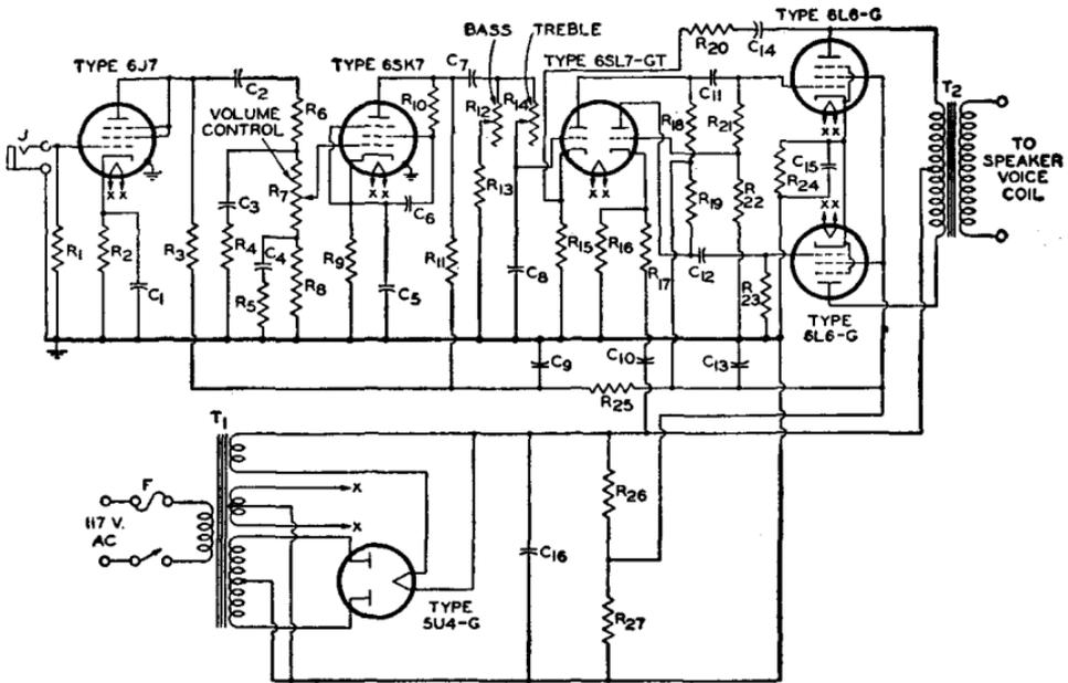
$C_1$   $C_3$   $C_{15}$  = 20  $\mu$ f, electrolytic, 25 v.
