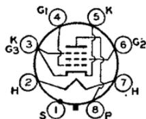
Metal type used as rf amplifier in high-frequency and wide-band applications. Features high transconductance with low grid-No.1-to-plate capacitance. Suitable for frequencies
