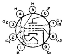
TION. Tube requires miniature nine-contact socket. Vertical tube mounting is preferred but horizontal mounting is permissible if pins No.3 and No.8 are in vertical plane.
