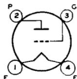
Glass type used in output stage of radio receivers. Outline 42, OUTLINES SECTION. Tube requires four-contact socket and should preferably be mounted in vertical position. Horizontal operation is permissible if pins 1 and 4 are in vertical plane. Filament volts (ac/dc), 2.5; amperes, 1.5. This type is used principally for renewal purposes.
