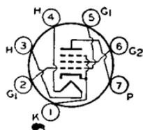
Miniature type used in the audio output stages of television receivers employing series-connected heater strings. Outline 13, OUTLINES SECTION. Tube requires miniature seven-contact socket and may be mounted in any position.
