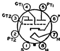
Tube requires octal socket and may be mounted in any position. For heater and cathode considerations, refer to type 6AV6. For typical operation as a resistance-coupled amplifier, refer to Chart 16, RESISTANCE-COUPLED AMPLIFIER SECTION.
