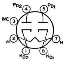
Octal type having high perveance used as a damper tube in horizontal deflection circuits of television receivers or as a rectifier in conventional power-supply applications. Outline 31, OUTLINES SECTION. Tube requires octal socket and may be mounted in any position. It is especially important that this tube, like other power-handling tubes, be adequately ventilated. Heater volts (ac/dc), 6.3; amperes, 1.6. Maxi-
