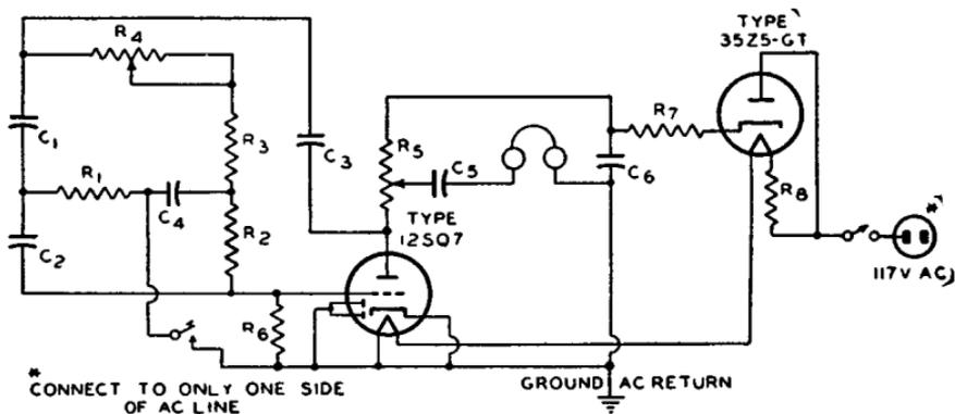
$C_1$   $C_2$  = 0.001  $\mu$ f, mica, 300 v.
