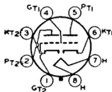
any position. Except for the common heater, each triode unit is independent of the other. For typical operation as phase inverter or resistance-coupled amplifier, refer to Chart 7, RESISTANCE-COUPLED AMPLIFIER SECTION. For heater and cathode considerations, refer to type 6AV6.
