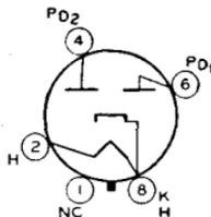
position. The heater is designed to operate from the ac line through a step-down transformer. The voltage at the heater terminals should be 5.0 volts under operating conditions at an average line voltage of 117 volts. It is especially important that this tube, like other power-handling tubes, be adequately ventilated.
