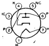
Miniature type used in power supply of small, portable, ac/dc/battery receivers where small size and low heat dissipation are important. Outline 11, OUTLINES SECTION. Tube requires miniature seven-contact socket and may be mounted in any position. Heater volts (ac/dc) 45; amperes, 0.075. Maximum ratings: peak inverse plate volts, 350 max; peak plate
