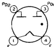
Glass type used to supply dc power of uniform voltage to receivers in which the rectified current requirements are subject to considerable variation. Outline 42, OUTLINES SECTION. Tube requires four-contact socket and should be mounted in vertical position with base down. Filament volts (ac), 2.5; amperes, 3. Maximum ratings for full-wave rectifier service: peak in-
