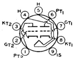
internal shield minimizes coupling between the two triode units so that either unit will give stable performance in vhf applications. Outline 12, OUTLINES SECTION. Tube requires miniature nine-contact socket and may be mounted in any position.
