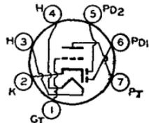
seven-contact socket and may be mounted in any position. For typical operation as resistance-coupled amplifier, refer to Chart 7, **RESISTANCE-COUPLED AMPLIFIER SECTION**. For heater considerations, refer to type 6AV6.
