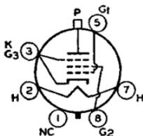
amperes, 0.6; warm-up time (average), 11 seconds. For definition of heater warm-up time and method for determining it, see type 6CG7. Peak heater-cathode volts, 200 max. When the heater is positive with respect to the cathode, the dc component of the heater-cathode voltage must not exceed 100 volts. Except for heater and heater-cathode ratings, type 25CD6-GA is identical with glass octal type 6CD6-G and type 25CD6-GB is identical with glass octal type 6CD6-GA.
