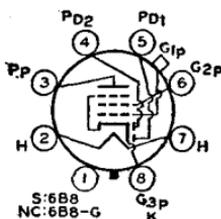
Heater volts (ac/dc), 6.3; amperes, 0.3. Maximum ratings of pentode unit as class A<sub>1</sub> amplifier: plate volts, 300 *max*; grid-No.2 (screen-grid) volts, 125 *max*; grid-No.2 supply volts, 300 *max*; grid-No.1 volts, 0 *min*; plate dissipation, 3.0 *max* watts (6B8), 2.25 *max* watts (6B8-G); grid-No.2 input, 0.3 *max* watt. For typical operation as a resistance-coupled amplifier, refer to Chart 5, RESISTANCE-COUPLED AMPLIFIER SECTION.
