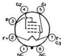
Glass octal type used in output stage of battery-operated receivers. Outline 41, OUTLINES SECTION. Tube requires octal socket. Filament volts (dc), 2.0; amperes, 0.12. Typical operation as class A<sub>1</sub> amplifier: plate and grid-No.2 (screen-grid) volts, 135 max; grid-No.1 volts, -16.5; plate ma., 7.0; grid-No.2 ma., 2.0; plate resistance, 105000 ohms; load resistance, 13500 ohms; output watts, 0.45. This is a DISCONTINUED type listed for reference only.
