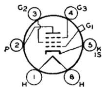
Glass type used as biased detector in ac-operated receivers. Outline 44, OUTLINES SECTION. Tube requires six-contact socket. Heater volts (ac/dc), 2.5; amperes, 1.0. Except for heater rating and capacitances, this type is electrically identical with metal type 6J7. Type 57 is a DISCONTINUED type listed for reference only.
