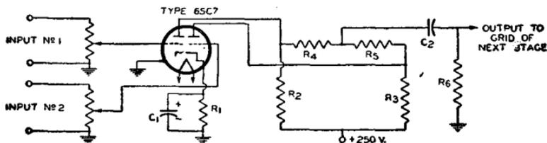
$C_1 = 10 \mu\text{f}$ , electrolytic, 25 v.
