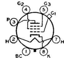
Glass octal type used as biased detector or high-gain audio amplifier in ac/dc radio receivers. Outline 24, OUTLINES SECTION. Heater volts (ac/dc), 12.6; amperes, 0.15. Except for heater rating, this type is identical with glass-octal type 6J7-GT. Type 12J7-GT is used principally for renewal purposes.
