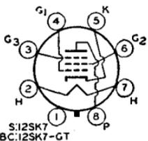
(ac/dc), 12.6; amperes, 0.15. Except for heater rating, type 12SK7 is identical with metal type 6SK7, and type 12SK7-GT is identical with glass-octal type 6SK7-GT. Type 12SK7-GT is used principally for renewal purposes.
