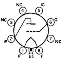
Glass lock-in type used as detector or voltage amplifier in battery-operated receivers. Outline 15, OUTLINES SECTION. Tube requires lock-in socket. Filament volts (dc), 1.4; amperes, 0.05. Typical operation as class A<sub>1</sub> amplifier: plate volts, 90 (110 max); grid volts, -3; plate ma., 1.4; plate resistance, 1900 ohms; transconductance, 760  $\mu$ hos; amplification factor, 14.5. This type is used principally for renewal purposes.
