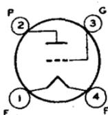
Glass type used as voltage amplifier or detector in battery-operated receivers. Outline 34 or 35, OUTLINES SECTION. Tube requires four-contact socket. Filament volts (dc), 2.0; amperes, 0.06. Except for interelectrode capacitances, this type is electrically identical with glass-octal type 1H4-G. Type 30 is a DISCONTINUED type listed for reference only.
