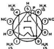
nine-contact socket and may be mounted in any position. For curve of average plate characteristics, see page 64. For high-voltage considerations, see type 1B3-GT.
