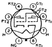
amperes, 0.3. Maximum ratings for each triode unit as class A<sub>1</sub> amplifier: plate volts, 250 max; grid volts, 0 min; plate dissipation, 1.0 max watt. Typical operation: plate volts, 250; grid volts, -4.5; plate ma., 3.2; plate resistance, 22500 ohms; amplification factor, 36; transconductance, 1600 μmhos. For typical operation as a resistance-coupled amplifier, refer to Chart 12, RESISTANCE-COUPLED AMPLIFIER SECTION. This type is used principally for renewal purposes.
