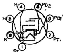
output stages in automobile receivers. It is equivalent in performance to metal type 6SR7. Outline 11, OUTLINES SECTION. Tube requires miniature seven-contact socket and may be mounted in any position. For typical operation as a resistance-coupled amplifier, refer to Chart 9, RESISTANCE-COUPLED AMPLIFIER SECTION. For heater and cathode considerations, refer to type 6AV6.
