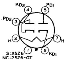
either the ac/dc type or the voltage-doubler type. Outlines 6 and 23, respectively, OUTLINES SECTION. Type 25Z6-GT may be supplied with pin No.1 omitted. Tubes require octal socket and may be mounted in any position. Type 25Z6 is a DISCONTINUED type listed for reference only.
