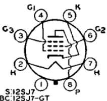
Heater volts (ac/dc), 12.6; amperes, 0.15. Except for heater rating, type 12SJ7 is identical with metal type 6SJ7, and type 12SJ7-GT is identical with glass-octal type 6SJ7-GT. Type 12SJ7-GT is a DISCONTINUED type listed for reference only.
