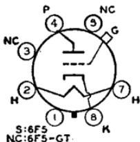
Metal type 6F5 and glass-octal type 6F5-GT used in resistance-coupled amplifier circuits. Outlines 4 and 21, respectively, OUTLINES SECTION. Tubes require octal socket and may be mounted in any position. Type 6F5-GT may be supplied with pin No.1 omitted. For typical operation as a resistance-coupled amplifier, refer to Chart 17, RESISTANCE-COUPLED AMPLIFIER SECTION. For
