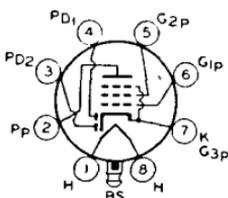
volts, -1 (*0 min*); plate resistance (approx.), 1.0 megohm; transconductance, 3200  $\mu$ hos; plate ma., 5.7; grid-No.2 ma., 2.1, grid-No.1 volts for transconductance of 10  $\mu$ hos, -30. Refer to type 6AV6 for diode operation curves. Type 7R7 is used principally for renewal purposes.
