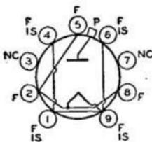
Miniature type used as rectifier of high-voltage pulses produced in the scanning systems of television receivers. Outline 17, OUTLINES SECTION. Tube requires miniature nine-contact socket and may be mounted in any position. Plate connection is cap at top of bulb. Pin No.3 may be connected to the filament, or used as a tie point for the filament-dropping resistor; otherwise it should not be used. For filament
