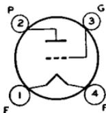
Glass type used in output stage of radio receivers. Outline 42, OUTLINES SECTION. Filament volts (ac/dc), 5.0; amperes, 1.25. Characteristics: plate volts, 250; grid volts, -60; plate ma., 30; amplification factor, 3; plate resistance, 1750 ohms; transconductance, 1700  $\mu$ mhos; load resistance, 5000 ohms; output watts, 1.8. This is a DISCONTINUED type listed for reference only.
