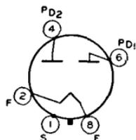
Metal type used in power supply of radio equipment having large dc requirements. Outline 7, OUTLINES SECTION. Tube requires octal socket. Vertical tube mounting is preferred but horizontal mounting is permissible if pins 2 and 8 are in vertical plane. Filament volts (ac), 5.0; amperes, 2.0. Maximum ratings as full-wave rectifier: peak inverse plate volts, 1550 max; peak plate ma., 675 max; dc output ma., 225 max. This type is used principally for renewal purposes.
