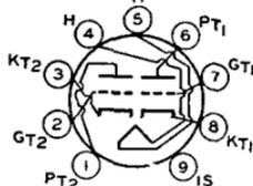
warm-up time (average), 11 seconds. For definition of heater warm-up time and method for determining it, see type 6CG7. Except for heater rating, type 5BQ7-A is identical with miniature type 6BQ7-A.
