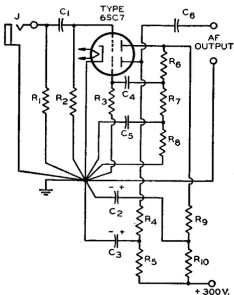
C<sub>1</sub> C<sub>4</sub> C<sub>6</sub>=0.05  $\mu$ f, paper, 600 v.
