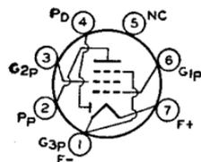
Miniature type used in light-weight, compact, portable, battery-operated receivers as combined detector and af voltage amplifier. The 1U5 is similar to the 1S5 but utilizes an improved structure which greatly reduces any tendency toward microphonic effects.
