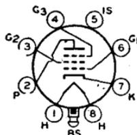
0.8 *max* watt; grid No.3 connected to cathode at socket; cathode-bias resistor, 160 *min* ohms; plate resistance, 0.3 megohm; transconductance, 5800  $\mu$ hos; plate ma., 10; grid-No.2 ma., 3.9; grid-No.1 volts for plate current of 10  $\mu$ a., -16. The application of this type is similar to that of miniature type 6AU6. Type 7V7 is used principally for renewal purposes.
