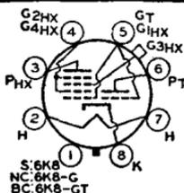
**OUTLINES SECTION.** Types 6K8-G and 6K8-GT are **DISCONTINUED** types listed for reference only. Tubes require octal socket and may be mounted in any position. For heater and cathode considerations, refer to type 6AV6. For application, refer to *Frequency Conversion* in **ELECTRON TUBE APPLICATIONS SECTION.**
