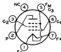
filament mid-tap so that tubes may be used either with a 1.4-volt battery supply or in series with other miniature tubes having 0.050-ampere filaments.
