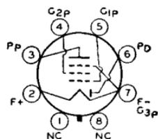
0.3 megohm; transconductance, 800 μmhos; load resistance, 25000 ohms; output watts, 0.1. This is a DISCONTINUED type listed for reference only.
