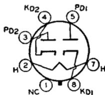
SECTION. This type may be supplied with pin No.1 omitted. Tube requires octal socket. Heater volts (ac/dc), 50; amperes, 0.15. Except for heater rating, this type is electrically identical with type 25Z6-GT.
