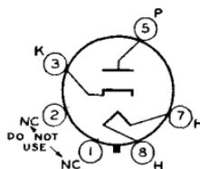
volts and a peak heater-cathode voltage rating of 450 max volts with heater negative with respect to cathode, this type is identical with glass octal type 6W4-GT. Type 25W4-GT is used principally for renewal purposes.
