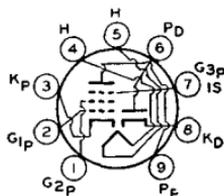
The high-perveance diode is used as an audio detector, video detector, or dc restorer. Outline 12, OUTLINES SECTION. Heater volts (ac/dc), 4.7; amperes, 0.6; warm-up time (average), 11 seconds. For definition of heater warm-up time and method for determining it, see type 6CG7. Except for heater rating, type 5AS8 is identical with miniature type 6AS8.
