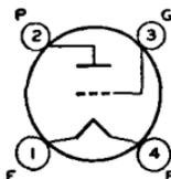
5000 ohms; transconductance, 1600 μmhos; load resistance, 10200 ohms; undistorted output watts, 1.6. This is a DISCONTINUED type listed for reference only.
