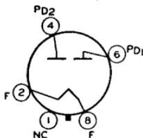
octal socket. Vertical tube mounting is preferred, but horizontal operation is permissible if pins 2 and 8 are in horizontal plane. It is especially important that these tubes, like other power-handling tubes, be adequately ventilated. Type 5Y3-G is a DISCONTINUED type listed for reference only. For discussion of Rating Chart and Operation Characteristics, refer to type 6AX5-GT.
