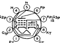
Heater volts (ac/dc), 4.7; amperes, 0.6; warm-up time (average), 11 seconds. For definition of heater warm-up time and method for determining it, see type 6CG7. Peak heater-cathode volts, 200 *max*. When the heater is positive with respect to the cathode, the dc component of the heater-cathode voltage must not exceed 100 volts. Except for heater and heater-cathode rating, type 5U8 is identical with miniature type 6U8.
