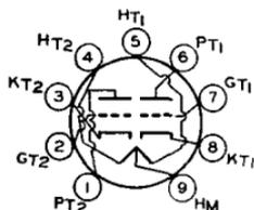
Miniature type used as frequency converter in vhf tuners of television receivers. Also used as rf amplifier, oscillator, or mixer. Outline 12, OUTLINES SECTION. Tube requires miniature nine-contact socket and may be mounted in any position. Each triode unit is independent of the other except for the common heater.
