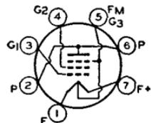
3V4 are identical. Refer to type 3V4 for ratings, typical operation, curves, and installation considerations.
