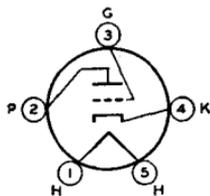
Glass type used as detector, amplifier, or oscillator in ac-operated receivers. Outline 34 or 35, OUTLINES SECTION. Tube requires five-contact socket. Heater volts (ac/dc), 2.5; amperes, 1.0. Except for heater rating, this type is electrically identical with glass type 76. Type 56 is a DISCONTINUED type listed for reference only.
