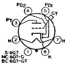
Metal type 6Q7 and glass-octal types 6Q7-G and 6Q7-GT used as combined detector, amplifier, and avc tubes in radio receivers. Outlines 4, 38, and 24, respectively, OUTLINES SECTION. Types 6Q7 and 6Q7-GT are used principally for renewal purposes. Type 6Q7-G is a DISCONTINUED type listed for reference only. Tubes require octal socket and may be mounted in any position. Heater volts (ac/dc),
