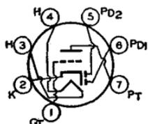
ment using this type should be designed so that 90 per cent of the maximum value of plate voltage is never exceeded for a battery potential of 13.2 volts. Tube requires miniature seven-contact socket and may be mounted in any position.
