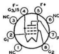
Subminiature type used as rf or if amplifier in stages not controlled by AVC in small, compact, battery-operated receivers for the standard AM broadcast band. Outline 8, OUTLINES SECTION. Tube requires subminiature eight-contact socket and may be mounted in any position. Base pins should not be soldered to circuit elements because the heat of the soldering operation may crack the glass seal. Filament volts
