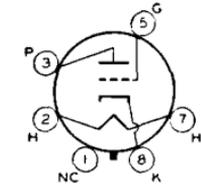
Glass octal type used as detector, amplifier, or oscillator in ac/dc radio equipment. Outline 25, OUTLINES SECTION. This type may be supplied with pin No.1 omitted. Heater volts (ac/dc), 12.6; amperes, 0.15. Except for heater rating, this type is identical with glass-octal type 6J5-GT. Type 12J5-GT is used principally for renewal purposes.
