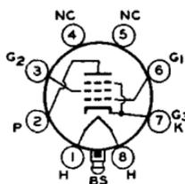
Glass lock-in type used in output stage of ac/dc receivers. Outline 20, OUTLINES SECTION. Tube requires lock-in socket. Heater volts (ac/dc), 35; amperes, 0.15. For ratings, and curves, refer to glass-octal type 35L6-GT. Type 35A5 is used principally for renewal purposes.
