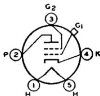
conductance, 1050 μmhos; plate ma., 4; grid-No.2 ma., 1.7 max. This type is used principally for renewal purposes.
