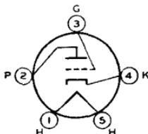
Glass type used as voltage amplifier or detector in ac-operated receivers. Outline 34 or 35, OUTLINES SECTION. Tube requires five-contact socket. Heater volts (ac/dc), 2.5; amperes, 1.75. Maximum ratings and characteristics as class A<sub>1</sub> amplifier: plate volts, 250 max; grid volts, -21; amplification factor, 9; plate resistance, 9250 ohms; transconductance, 975  $\mu$ mhos; plate ma., 5.2. This type is used principally for renewal purposes.
