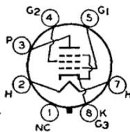
plate volts, 135 (200 max); grid-No.2 (screen-grid) volts, 135 max; plate dissipation, 12.5 max watts; grid-No.2 input, 1.75 max watts; grid-No.1 (control-grid) volts, -13.5; plate ma., 58; grid-No.2
