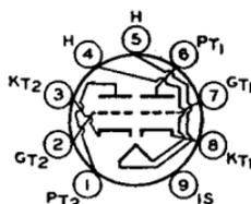
rf stage of television receivers utilizing a cathode-drive amplifier of the direct-coupled type or in push-pull cathode-drive rf amplifiers. Outline 12, OUTLINES SECTION. Tube requires miniature nine-contact socket and may be mounted in any position.
