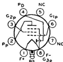
Glass lock-in type used as combined detector and af voltage amplifier in battery-operated receivers. Outline 15, OUTLINES SECTION. Tube requires lock-in socket. Filament volts (dc), 1.4; amperes, 0.05. Characteristics of pentode unit: plate volts, 90 (110 max); grid-No.2 volts, 45; grid-No.1 volts, 0; plate ma., 0.6; grid-No.2 ma., 0.1; plate resistance, 0.75 megohm; transconductance, 575  $\mu$ hos. This type is used principally for renewal purposes.
