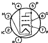
a power output of 5.5 watts at moderate frequencies, and 2.5 watts at 150 megacycles per second. Outline 11, OUTLINES SECTION. Tube requires miniature seven-contact socket and may be mounted in any position. For typical operation as a resistance-coupled amplifier, refer to Chart 10, RESISTANCE-COUPLED AMPLIFIER SECTION. For heater and cathode considerations, refer to type 6AV6. For additional curve of plate characteristics, refer to type 12AU7.
