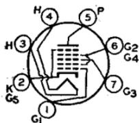
Miniature type used as converter in ac/dc receivers for both standard broadcast and FM bands. Outline 11, OUTLINES SECTION. Heater volts (ac/dc), 12.6; amperes, 0.15. Except for heater rating, this type is identical with miniature type 6BE6.
