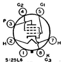
Metal type 25L6 and glass-octal type 25L6-GT are used in output stage of ac/dc receivers. Outlines 6 and 23, respectively, OUTLINES SECTION. These tubes require octal sockets and may be mounted in any position. Type 25L6-GT may be supplied with pin No.1 omitted. Heater volts (ac/dc), 25; amperes, 0.3. For maximum ratings and typical
