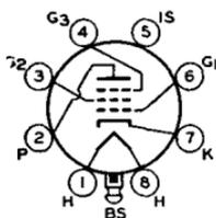
Lock-in type used in output stage of video amplifier of television receivers. Outline 20, OUTLINES SECTION. Tube requires lock-in socket. Heater volts (ac/dc), 6.3; amperes, 0.6. Typical operation and ratings as class A<sub>1</sub> video amplifier: plate volts, 300 *max*; grid-No.2 volts, 150 *max*; plate dissipation, 10 *max* watts; grid-No.2 input, 1.2 *max* watts; cathode resistor, 68
