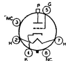
*max*, 6BD4-A 55000 *max*; dc grid volts, -125 *max*; peak grid volts, -550 *max*; dc plate ma., 1.5 *max*; plate dissipation, 6BD4 20 *max* watts, 6BD4-A 25 *max* watts; peak heater-cathode volts, 180 *max*. When operated at plate voltages above 16000 volts, these tubes will produce X-rays which can constitute a health hazard unless the tubes are adequately shielded. Type 6BD4 is a DISCONTINUED type listed for reference only. Type 6BD4-A is used principally for renewal purposes.
