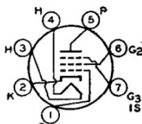
in vhf television tuners. This tube features very high transconductance combined with low interelectrode capacitance values, and is provided with separate base pins for grid No.3 and cathode to permit the use of an unbypassed cathode resistor to minimize the effects of regeneration. Outline 11, OUTLINES SECTION. Tube requires miniature seven-contact socket and may be mounted in any position.
