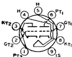
Heater volts (ac/dc), 8.4; amperes, 0.45; warm-up time (average), 11 seconds. For definition of heater warm-up time and method for determining it, see type 6CG7. Except for heater rating, type 8CG7 is identical with miniature type 6CG7.
