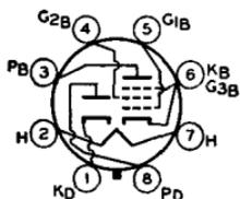
Glass octal type used as combined half-wave rectifier and output amplifier in ac/dc receivers. Outline 27, OUTLINES SECTION. Tube requires octal socket. Heater volts (ac/dc), 70; amperes, 0.15. Maximum ratings of rectifier unit: peak inverse plate volts, 350; peak plate ma., 420; dc output ma., 70; peak heater-cathode volts, 175; minimum total effective
