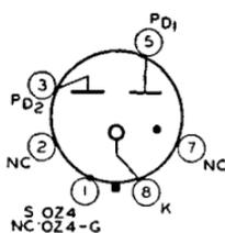
Maximum ratings for full-wave rectifier service: peak starting supply volts (per plate), 300 *max*; peak plate-to-plate volts, 1000 *max*; peak plate ma. (per plate), 200 *max*; dc output ma., 75 *max*, 30 *min*; dc output volts, 300 *max*; average dynamic tube voltage drop, 24 volts. These types are used principally for renewal purposes.
