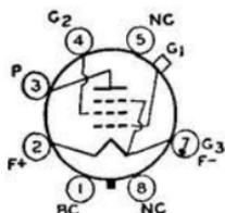
Glass octal type used as rf or if amplifier in battery-operated receivers. Outline 24, OUTLINES SECTION. Tube requires octal socket. Filament volts (dc), 1.4; amperes, 0.05. Typical operation as class A<sub>1</sub> amplifier: plate volts, 90 (110 max); grid-No.2 (screen-grid) volts, 90 (110 max); grid-No.1 volts, 0; plate resistance (approx.), 0.8 megohm; transconductance, 750  $\mu$ mhos; transconductance (approx.) with -12
