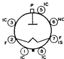
scanning systems. When used as an rf rectifier, one 1B3-GT in a half-wave circuit is capable of delivering a maximum dc output voltage of about 15000 volts. In a voltage-doubler circuit, two tubes will give about 30000 volts; and in a voltage-tripler circuit, three 1B3-GT's will deliver 45000 volts approximately. For curve of average plate characteristics, see page 64.
