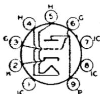
Miniature types having high permeance used as vertical deflection amplifiers in television receivers. Type 6S4-A has a controlled heater warm-up time for use in television receivers employing series-connected heater strings. Outline 14, OUTLINES SECTION. Tubes require miniature nine-contact socket and may be mounted in any position. For heater and cathode considerations, refer to type 6AQ5. Type 6S4 is used principally for renewal purposes.
