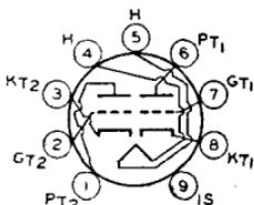
Miniature type used as vertical deflection oscillator and horizontal deflection oscillator in television receivers employing series-connected heater strings. Also used as phase inverter, sync separator and amplifier, and resistance-coupled amplifier in radio equipment. Except for the common heater, each triode unit is independent of the other. For typical operation as phase inverter or resistance-coupled amplifier, refer to Chart 13, RESISTANCE-COUPLED AMPLIFIER SECTION.
