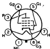
Glass octal type used as output amplifier. Outline 41, OUTLINES SECTION. Heater volts (ac/dc), 25; amperes, 0.3. Refer to type 6Y6-G for typical operation as a class A<sub>1</sub> amplifier. Type 25C6-G is a DISCONTINUED type listed for reference only.
