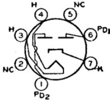
Miniature type used in power supply of automobile and ac-operated radio receivers. Equivalent in performance to larger types 6X5 and 6X5-GT. Type 6X4 requires miniature seven-contact
