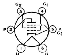
Glass type used in audio output stage of ac/dc receivers. Outline 42, OUTLINES SECTION. Tube requires six-contact socket. Heater volts (ac/dc), 25; amperes, 0.3. This type is electrically identical with type 25A6. Type 43 is used principally for renewal purposes.
