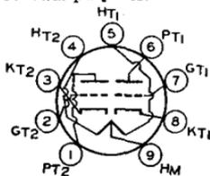
Miniature type used as a combined vertical deflection amplifier and vertical deflection oscillator, and as a horizontal deflection oscillator, in television receivers employing series-connected heater strings. Also used as audio mixer, phase inverter, multivibrator, sync separator and amplifier, and resistance-coupled amplifier in radio equipment. Outline 12, OUTLINES SECTION. Tube requires miniature nine-contact socket and may be mounted in any position. Each triode unit is independent of
