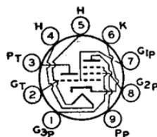
Heater volts (ac/dc), 4.7; amperes, 0.6; warm-up time (average), 11 seconds. For definition of heater warm-up time and method for determining it, see type 6CG7. Peak heater-cathode volts, 200 *max*. When the heater is positive with respect to the cathode, the dc component of the heater-cathode voltage must not exceed 100 volts. Except for heater and heater-cathode ratings, type 5X8 is identical with miniature type 6X8.
