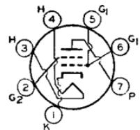
Miniature type used as power amplifier driver in automobile radio receivers operating from a 12-volt storage battery. Outline 13, OUTLINES SECTION. Equipment using this type
