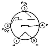
Glass type used in power supply of automobile and ac-operated radio receivers. Outline 34 or 35, OUTLINES SECTION. Tube requires five-contact socket. Heater volts (ac/dc), 6.3; amperes, 0.5. Maximum ratings: peak inverse plate volts, 1250 *max*; peak plate ma., 180 *max*; dc output ma., 60 *max*; peak heater-cathode volts, 450 *max*. Typical operation with capaci-
