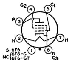
Outlines 6, 41, and 27, respectively, OUTLINES SECTION. Type 6F6-GT may be supplied with pin No.1 omitted. Tubes require octal socket and may be mounted in any position. It is especially important that these tubes, like other power-handling tubes, be adequately ventilated. Types 6F6-G and 6F6-GT are used principally for renewal purposes.
