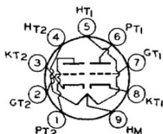
devices. Outline 12, OUTLINES SECTION. Tube requires miniature nine-contact socket and may be mounted in any position. Its characteristics are similar to glass-octal type 6SL7-GT. Each triode unit is independent of the other except for the common heater. For characteristics and curves, refer to type 6AV6. For typical operation as a resistance-coupled amplifier, refer to Chart 20, RESISTANCE-COUPLED AMPLIFIER SECTION.
