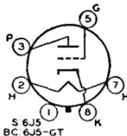
high amplification factor. Outlines 3 and 25, respectively, OUTLINES SECTION. Tubes require octal socket and may be mounted in any position. For heater and cathode considerations, refer to type 6AV6. For typical operation as resistance-coupled amplifiers, refer to Chart 13, RESISTANCE-COUPLED AMPLIFIER SECTION.
