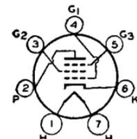
Glass type used in audio output stage of ac-operated receivers. Outline 52, OUTLINES SECTION. Tube requires medium seven-contact (0.855-inch, pin-circle diameter) socket. Heater volts (ac/dc), 2.5; amperes, 2.0. Typical operation as class A<sub>1</sub> amplifier (triode connection; grids No.2 and No.3 tied to plate); plate volts, 250 max; grid volts, -28; plate ma., 26;
