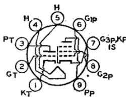
amperes, 0.6; warm-up time (average), 11 seconds. For definition of heater warm-up time and method for determining it, see type 6CG7. Except for heater rating and basing arrangement, type 5AV8 is identical with miniature type 6AN8.
