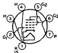
OUTLINES SECTION. Heater volts (ac/dc), 3.15; amperes, 0.6; warm-up time (average), 11 seconds. For definition of heater warm-up time and method for determining it, see type 6CG7. Peak heater-cathode volts, 200 *max.* When the heater is positive with respect to the cathode, the dc component of the heater-cathode voltage must not exceed 100 volts. Except for heater and heater-cathode ratings, type 3BN6 is identical with miniature type 6BN6.
