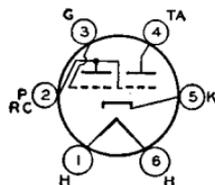
Glass type used to indicate visually by means of a fluorescent target the effects of a change in a controlling voltage. It is used as a convenient means of indicating accurate radio-receiver tuning. Outline 34, OUTLINES SECTION. Tube requires six-contact socket. For heater and cathode considerations, refer to type 6AV6. Heater volts (ac/dc) 6.3; amperes, 0.15. Ratings: plate-supply volts, 180 *max*; target volts, 180 *max*, 125 *min*. This type is used principally for renewal purposes.
