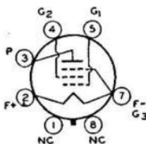
Glass octal type used in the output stage of battery-operated receivers. Outline 23, OUTLINES SECTION. This type may be supplied with pin No.1 omitted. Tube requires octal socket. Filament volts (dc), 1.4; amperes, 0.1. For electrical characteristics and ratings, refer to type 3Q5-GT with parallel filament arrangement. Type 1Q5-GT is a DISCONTINUED type for reference only.
