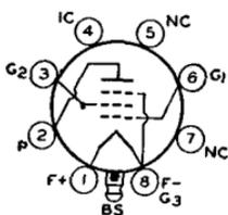
Glass lock-in type used in output stage of battery-operated receivers. Outline 15, OUTLINES SECTION. Tube requires lock-in socket. Filament volts (dc), 1.4; amperes, 0.05. For electrical characteristics, refer to pentode unit of glass-octal type 1D8-GT. Type 1LB4 is used principally for renewal purposes.
