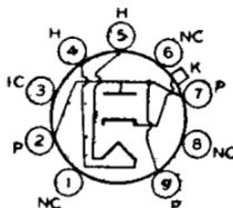
miniature nine-contact socket and may be mounted in any position. It is especially important that this tube, like other power-handling tubes, be adequately ventilated.
