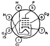
should be designed so that 90 per cent of the maximum values of plate voltage and grid-No.2 voltage is never exceeded for a battery potential of 13.2 volts. Tube requires miniature seven-contact socket and may be mounted in any position.
