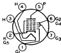
per. Outline 11, OUTLINES SECTION. Heater volts (ac/dc), 3.15; amperes, 0.6; warm-up time (average), 11 seconds. For definition of heater warm-up time and
