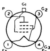
resistance, 1.0 megohm; transconductance, 620  $\mu$ mhos; transconductance at grid-No.1 voltage of -22.5 volts, 15  $\mu$ mhos. This is a **DISCONTINUED** type listed for reference only.
