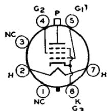
(ac/dc), 25; amperes, 0.3. Except for heater rating, type 25BQ6-GT is identical with glass octal type 6BQ6-GT, and type 25BQ6-GTB/25CU6 is identical with glass octal type 6BQ6-GTB/6CU6. Type 25BQ6-GT is used principally for renewal purposes.
