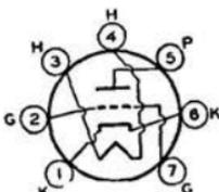
(ac/dc), 2.3; amperes, 0.6; warm-up time (average), 11 seconds. For definition of heater warm-up time and method for determining it, see type 6CG7. Except for heater rating, type 2BN4 is identical with miniature type 6BN4.
