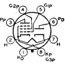
μmhos; load resistance, 4500 ohms; output watts, 0.77. Maximum ratings of rectifier unit: peak inverse plate volts, 350; peak plate ma., 450; dc output ma., 75; peak heater-cathode volts, 175. This is a DISCONTINUED type listed for reference only.
