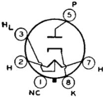
octal socket and may be mounted in any position. This type may be supplied with pin No.1 omitted. For installation and application considerations, refer to miniature type 35W4.
