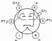
Glass type used in output stage of radio receivers as a class B power amplifier or a class A<sub>1</sub> driver. Outline 34, OUTLINES SECTION. Tube requires six-contact socket. Heater volts (ac/dc), 6.3; amperes, 0.6. Maximum ratings and typical operation as class B power amplifier: plate volts, 250 *max*; grid volts, 0; zero-signal plate ma., 10.5; effective load resistance
