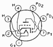
Miniature type used as a combined detector, amplifier, and avc tube in compact ac/dc radio receivers. Outline 12, OUTLINES SECTION. Heater volts (ac/dc), 12.6; amperes, 0.15. Except for the heater rating, this type is identical with miniature type 6AT6.
