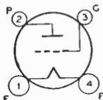
Glass type used in output stage of audio-frequency amplifiers. Outline 36, OUTLINES SECTION. Tube requires four-contact socket. Filament volts (ac/dc), 5.0; amperes, 0.25. Characteristics as class A<sub>1</sub> amplifier: plate volts, 180 *max*; grid volts, -40.5; cathode resistor, 2150 ohms; plate ma., 20; plate resistance, 1750 ohms; amplification factor, 3; transconductance,
