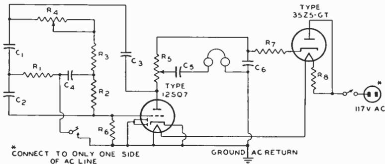
C<sub>1</sub> C<sub>2</sub> = 0.001  $\mu$ f, mica, 300 v.
