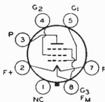
series filament arrangement, filament voltage is applied between pins 2 and 7. For parallel filament arrangement, filament voltage is applied between pin 8 and pins 2 and 7 connected together. For additional filament considerations, refer to type 3V4 and ELECTRON TUBE INSTALLATION SECTION.
