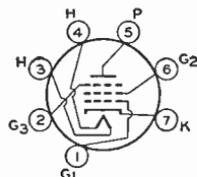
Tube requires miniature seven-contact socket and may be mounted in any position. For heater and cathode considerations, refer to type 6AQ5.
