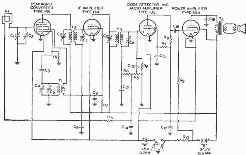
C<sub>1</sub> C<sub>4</sub> = Ganged tuning capacitors: C<sub>1</sub>, 10-274  $\mu\text{mf}$ ; C<sub>4</sub>, 7.5-122.5  $\mu\text{mf}$
