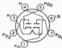
Heater volts (ac/dc), 12.6; amperes, 0.15. Except for heater rating, this type is identical with miniature type 6AL5.
