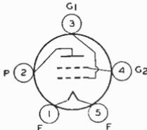
Glass type used as class A<sub>1</sub> or class B amplifier in radio equipment. Outline 41, OUTLINES SECTION. Tube requires five-contact socket. Filament volts (ac/dc), 2.5; amperes, 1.75. Typical operation as class A<sub>1</sub> amplifier (grid No.2 connected to plate at socket): plate volts, 250 *max*; grid volts, -33; plate ma., 22; plate resistance, 2380 ohms; am-
