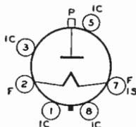
scanning systems. When used as an rf rectifier, one 1B3-GT in a half-wave circuit is capable of delivering a maximum dc output voltage of about 15000 volts. In a voltage-doubler circuit, two tubes will give about 30000 volts; and in a voltage-tripler circuit, three 1B3-GT's will deliver 45000 volts approximately.
