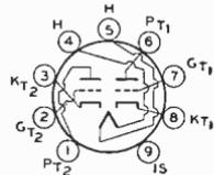
Miniature types used as first rf amplifier in tuners of vhf television receivers or as low-noise if pre-amplifier tube in uhf television receivers employing a crystal mixer. Both types are especially useful in the rf stage of television receivers utilizing a driven grounded-grid amplifier of the direct-coupled type or in push-pull grounded-grid rf amplifiers. Outline 13, OUTLINES SECTION. Tubes require noval nine-contact socket and may be mounted in any position.
