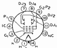
4000 *max*; anode-No.1 volts, 1500 *max*), this type is identical with type 7JP4. The 7JP4 may be used to replace the 7GP4 provided no connections are made to pins 4 and 12. The 7GP4 is a DISCONTINUED type listed for reference only.
