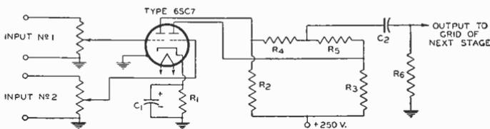
$C_1 = 8 \mu\text{f}$ , electrolytic, 25 v.
