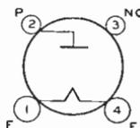
**FULL-WAVE MERCURY-VAPOR RECTIFIER**
