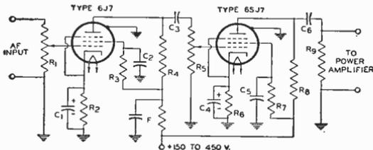
C<sub>1</sub> C<sub>4</sub> = 8  $\mu$ f, electrolytic, 25 v.
