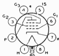
max watt; grid No.1 volts, -3; grid No.3 connected to cathode at socket; plate resistance, greater than 1 megohm; transconductance, 1575  $\mu$ mhos; plate ma., 2.2; grid-No.2 ma., 0.7. Within the limits of its maximum ratings, this type is similar in performance to metal types 6SJ7 and 12SJ7.
