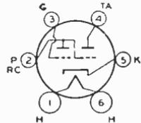
accurate radio-receiver tuning. Outline 30, OUTLINES SECTION. Tube requires six-contact socket and may be mounted in any position. For heater and cathode considerations, refer to type 6AV6. Type 6U5 has a remote plate-current cutoff characteristic. For a discussion of electron-ray tube considerations, refer to ELECTRON TUBE APPLICATION SECTION.
