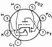
output stages in automobile receivers. It is equivalent in performance to metal type 6SR7. Outline 12, **OUTLINES SECTION**. Tube requires miniature seven-contact socket and may be mounted in any position. For typical operation as a resistance-coupled amplifier, refer to Chart 9, **RESISTANCE-COUPLED AMPLIFIER SECTION**. For heater and cathode considerations, refer to type 6AV6.
