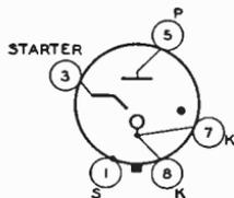
Metal type used primarily in vibrator-type B-supply units of automobile receivers. Utilizes a starter electrode and an ionically heated cathode. Starter anode permits operation of OY4 directly from 117-volt ac line. Outline 3, OUTLINES SECTION. Tube requires octal socket. Pins 7 and 8 must be tied together at socket. RF filter circuits placed close to socket terminals are required to reduce rectifier noise. Ratings as
