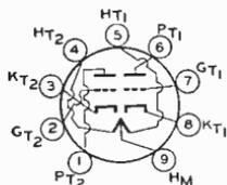
Miniature type used as grounded-grid amplifier or frequency converter in the FM and television broadcast bands. Outline 13, OUTLINES SECTION. Tube requires noval nine-contact socket and may be mounted in any position. Each triode unit is independent of the other except for the common heater.
