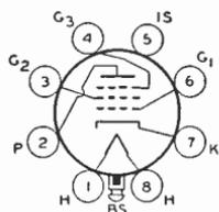
Glass lock-in type used as rf amplifier in ac/dc receivers or in mobile equipment where low heater-current drain is important. Outline 14, OUTLINES SECTION. Tube requires lock-in socket. Heater volts (ac/dc), 6.3; amperes, 0.15. Maximum ratings and characteristics as class A<sub>1</sub> amplifier: plate and grid-No.2 volts, 250 (300 *max*); plate dissipation, 2 *max* watts; grid-No.2 input, 0.75 *max* watt; grid
