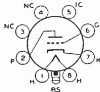
Glass lock-in type used as detector, amplifier, or oscillator in ac/dc radio receivers. Outline 14, OUTLINES SECTION. Tube requires lock-in socket. Heater volts (ac/dc), 12.6; amperes, 0.15. Except for heater rating and capacitances, this type is electrically identical with lock-in type 7A4 and metal type 6J5. The application of this type is similar to that of glass-octal type 12J5-GT.
