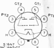
as a class B amplifier. Outlines 6 and 22, respectively, OUTLINES SECTION. Tubes require octal socket and may be mounted in any position. For typical operation as a resistance-coupled amplifier, refer to Chart 6, RESISTANCE-COUPLED AMPLIFIER SECTION. For class B amplifier considerations, refer to ELECTRON TUBE APPLICATIONS SECTION.
