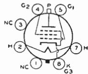
octal socket and may be mounted in any position. Heater volts (ac/dc), 25; amperes, 0.3. Except for heater rating, this type is identical with glass octal type 6BQ6-GT.
