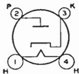
Glass type used in ac/dc or automobile receivers. Outline 32, OUTLINES SECTION. Tube requires four-contact socket. For heater considerations, refer to type 6AT6. Heater volts (ac/dc), 6.3; amperes, 0.3. Maximum ratings as half-wave rectifier: peak inverse plate volts, 1000; peak plate ma., 270; peak heater-cathode volts, 500; dc output ma., 45. This type is used principally for renewal purposes.
