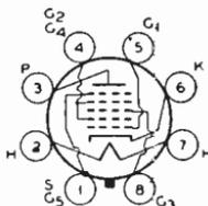
cycle region. The 6SB7-Y has a micanol base which minimizes drift in oscillator frequency during warm-up period. For general discussion of pentagrid types, see **Frequency Conversion** in ELECTRON TUBE APPLICATIONS SECTION. Outline 3, OUTLINES SECTION. Tube requires octal socket and may be mounted in any position. For heater and cathode considerations, refer to type 6AV6.
