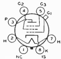
amplifier: plate volts, 300; grid-No.2 (screen) volts, 100; grid-No.2 sup; volts, 300; grid-No.1 (control-grid) volts, 0 *min*; plate dissipation, 2.25 watts; grid-No.2 input, 0.25
