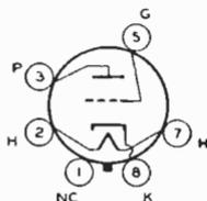
As a class A<sub>1</sub> amplifier, the 6L5-G may be operated in resistance-coupled circuits as shown in Chart 15, RESISTANCE-COUPLED AMPLIFIER SECTION. This type is used principally for renewal purposes.
