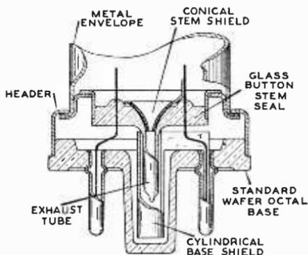
the capacitance between them is kept to a value comparable with that obtainable with top-cap construction.
