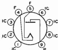
Miniature type used in high-voltage, low-current applications such as the rectifier in high-voltage, pulse-operated voltage-doubling power supplies for kinescopes. The very low power
