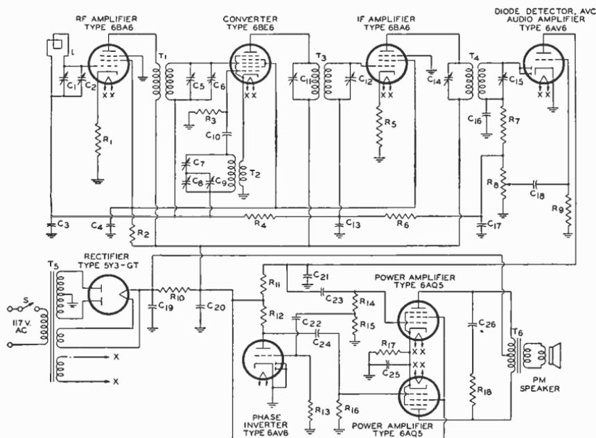
C<sub>1</sub> C<sub>5</sub> C<sub>8</sub>=Ganged tuning capacitors, 365  $\mu$ f
