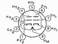
Miniature type used as a combined vertical deflection amplifier and vertical oscillator in television receivers. It is also used in other applications including phase-inverter circuits and multivibrator circuits. Outline 16, OUTLINES SECTION. Tube requires noval nine-contact socket and may be mounted in any position. Each triode unit is independent of the other except for the common heater.
