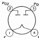
be mounted preferably in a vertical position. Horizontal mounting is permissible if pins 1 and 4 are in a horizontal plane. Filament volts (ac), 5.0; amperes, 2.0. For filament operation, refer to type 5U4-G. Type 80 is electrically identical with glass-octal type 5Y3-GT.
