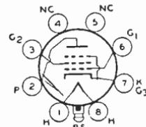
Glass lock-in type used as output amplifier in ac/dc radio receivers. Outline 14, OUTLINES SECTION. Tube requires lock-in socket. Heater volts (ac/dc), 12.6; amperes, 0.15. Typical operation and ratings as class A<sub>1</sub> amplifier: plate volts and grid-No.2 volts, 250 (300 *max*); plate dissipation, 7.5 watts; grid-No.2 input, 1.5 watts; grid-No.1 volts, -12.5; plate ma., 32;
