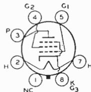
OUTLINES SECTION. Tube requires octal socket and may be mounted in any position.
