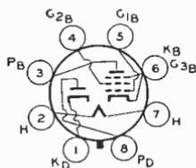
plate-supply impedance, 15 ohms. Typical operation and maximum ratings of beam power unit as class A<sub>1</sub> amplifier: plate and grid-No.2 volts, 110 (117 *max*); grid-No.1 volts, -7.5; plate ma., 40; grid-No.2 ma., 3; plate resistance, 15000 ohms; transconductance, 7500 μmhos; load resistance, 2000 ohms; output watts, 1.8; plate dissipation, 5 *max* watts; grid-No.2 input, 1 *max* watt.
