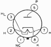
Glass octal type used in power supply of ac/dc receivers. The heater is provided with a tap for operation of a panel lamp. Outline 22, OUTLINES SECTION. Tube requires octal socket. Except for difference in heater voltage, this type has the same ratings and typical operation values as glass-octal type 35Z5-GT.
