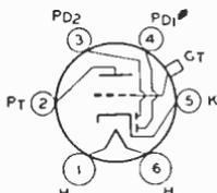
Glass type used as combined detector, amplifier, and avc tube in radio receivers. Outline 34, OUTLINES SECTION. Tube requires six-contact socket. Heater volts (ac/dc), 6.3; amperes, 0.3. Except for interelectrode capacitances and plate volts of 250 *max*, this type is identical electrically with metal type 6SQ7. Type 75 is used principally for renewal purposes.
