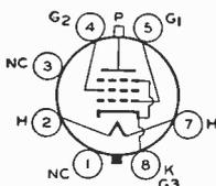
SECTION. Tube requires octal socket and may be mounted in any position.
