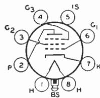
Glass lock-in type used as rf amplifier in high-frequency and wide-band applications. Outline 14, OUTLINES SECTION. Tube requires lock-in socket. Heater volts (ac/dc), 6.3; amperes, 0.15. Maximum ratings and characteristics as class A<sub>1</sub> amplifier: plate and grid-No.2 volts, 250 (300 *max*); plate dissipation, 2 *max* watts; grid-No.2 input, 0.7 *max* watt; cathode resistor, 250 ohms; grid No.3 and internal shield
