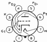
trically as type 6AT6. Outline 3, OUTLINES SECTION. Tube requires octal socket and may be mounted in any position. Heater volts (ac/dc), 6.3; amperes, 0.15. Direct interelectrode capacitances of triode unit (shell connected to cathode): grid to plate, 1.1  $\mu\text{mf}$ ; input, 2.4  $\mu\text{mf}$ ; output, 2.8  $\mu\text{mf}$ . For diode operation curves, refer to type 6SQ7.
