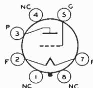
may be used and grid bias adjusted so that zero-signal plate ma. is about 0.2. This type is used principally for renewal purposes.
