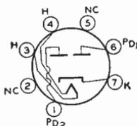
Miniature type used in power supply of automobile and ac-operated radio receivers. Equivalent in performance to larger types 6X5 and 6X5-GT.
