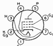
LINES SECTION. Tube requires miniature seven-contact socket and may be mounted in any position.
