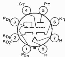
octal socket. Heater volts (ac/dc), 6.3; amperes, 0.3. Ratings and characteristics of triode unit as class A<sub>1</sub> amplifier: plate volts, 250 max; grid volts, -2; amplification factor, 70; plate resistance (approx.), 44000 ohms; transconductance, 1600 μmhos; plate ma., 2.3. For typical operation as a resistance-coupled amplifier, refer to Chart 7, RESISTANCE-COUPLED AMPLIFIER SECTION.
