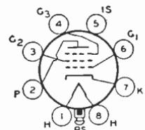
Glass lock-in type used as rf or if amplifier in radio receivers employing avc. Outline 14, OUTLINES SECTION. Tube requires lock-in socket. Heater volts (ac/dc), 6.3; amperes, 0.15. Typical operation as class A<sub>1</sub> amplifier: plate volts, 250 (300 *max*); grid-No.2 volts, 100 *max*; grid-No.1 volts, -3; grid No.3 connected to cathode at socket; plate ma., 8.5; grid-No.2
