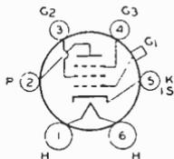
Glass type used as biased detector or high-gain amplifier in radio receivers. Outline 34, OUTLINES SECTION. Tube requires six-contact socket. Heater volts (ac/dc), 6.3; amperes, 0.3. Except for capacitances and grid-No. 2 rating of 100 *max* volts, type 77 is electrically identical with metal type 6J7. This type is used principally for renewal purposes.
