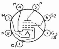
Miniature type used as rf amplifier particularly in ac/dc receivers and in mobile equipment where low heater-current drain is important. It is particularly useful in high-frequency, wide-band applications. Outline 12, OUTLINES SECTION. Tube requires miniature seven-contact socket and may be mounted in any position. For heater and cathode considerations, refer to type 6AV6.
