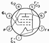
Miniature type used in output stage of lightweight, compact, portable, battery-operated equipment. Types 1S4 and 3S4 are identical except for filament arrangement. Outline 12, OUTLINES SECTION. Type 1S4 requires miniature seven-contact socket and may be mounted in any position. For ratings, typical operation, and curves, refer to type 3S4 with parallel filament arrangement. For filament con-
