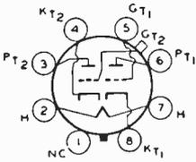
Glass octal type used as voltage amplifier or phase inverter in radio equipment. Except for common heater each triode is independent of the other. Outline 33, OUTLINES SECTION. Tube requires octal socket. Except for the heater rating of 6.3 volts (ac/dc) and 0.6 ampere and interelectrode capacitances, each triode unit is identical electrically with type 6J5. For typical operation as a resistance-coupled amplifier, refer to Chart 13, RESISTANCE-COUPLED AMPLIFIER SECTION.
