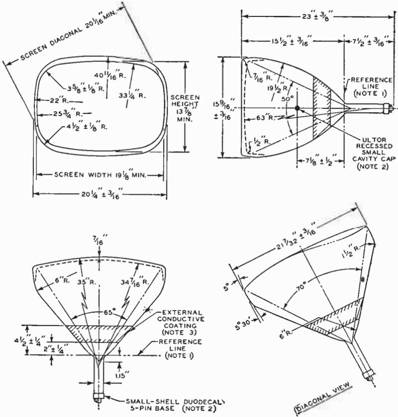
NOTE 1: With tube neck inserted through flared end of reference-line gauge (see page 291) and with tube seated in gauge, the reference line is determined by the intersection of the plane CC' of the gauge with the glass funnel.
