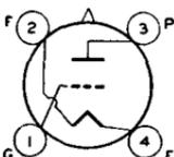
Thoriated-tungsten-filament type used as af power amplifier and modulator. Class AB<sub>1</sub> maximum CCS plate dissipation, 100 watts. Requires Jumbo four-contact socket and may be
