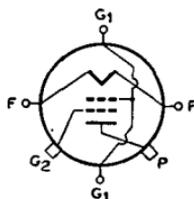
Forced-air-cooled type having thoriated-tungsten filament and integral radiator used as rf power amplifier and oscillator at frequencies up to 110 Mc. Class C Telegraphy maximum CCS plate dissipation, 800 watts.
