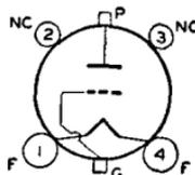
plate to filament, 2.8  $\mu\mu\text{f}$ . Maximum CCS ratings as **RF POWER AMPLIFIER AND OSCILLATOR**: dc plate volts, 1250 *max*; dc grid volts, -400 *max*; dc plate milliamperes, 80 *max*; dc grid milliamperes, 25 *max*; plate input, 100 *max* watts; plate dissipation, 35 *max* watts. Plate shows no color when tube is operated at maximum CCS ratings. The 800 is used principally for renewal purposes.
