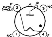
Jumbo four-contact socket and may be mounted in vertical position only, base down. OUTLINE 52, *Outlines* Section.
