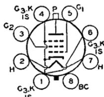
reduced input up to 175 Mc. Class C Telegraphy maximum plate dissipation, CCS 20 watts, ICAS 25 watts. Requires Octal socket and may be mounted in any position. *OUTLINE 17, Outlines Section.* Heater volts (ac/dc), 12.6 ± 10%; amperes, 0.625. Except for heater rating, the 6883 is identical with type 6146.
