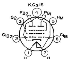
Small, sturdy, heater-cathode type used as a power amplifier and modulator, as rf power amplifier and oscillator, and as frequency tripler. May be used with full input up to 250
