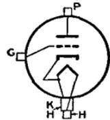
use in cathode-drive circuits of the coaxial-cylinder type. May be used with full input up to 900 Mc and with reduced input up to 2000 Mc. Class C Telegraphy maximum CCS plate dissipation, 250 watts.
