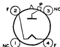
Maximum ratings: peak inverse plate volts, 7500 *max*; peak plate amperes, 0.6 *max*; average plate amperes, 0.15 *max*. The 217-C is used principally for renewal purposes.
