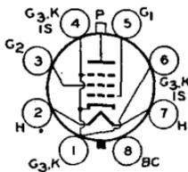
up to 175 Mc. Class C Telephony maximum plate dissipation, CCS 10 watts, ICAS 13.5 watts.
