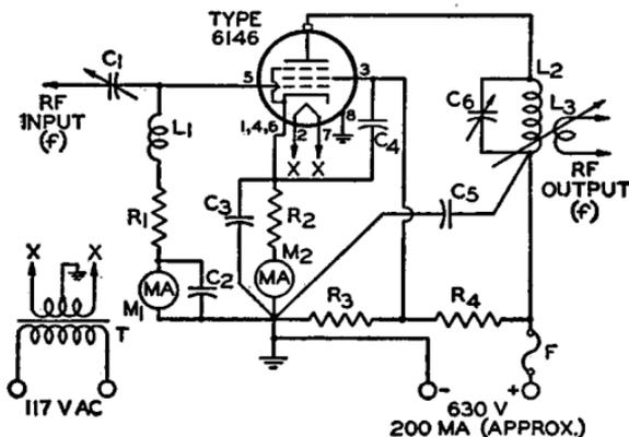
$C_1=4-50 \mu\text{f}$ , trimmer, air gap 0.015 inch
