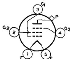
duced to 80 per cent; at 75 Mc, to 64 per cent. Class C Telegraphy maximum plate dissipation, CCS 50 watts, ICAS 65 watts. Requires Small five-contact socket and may be mounted in vertical position with base down, or in horizontal position with pins 2 and 4 in vertical plane. OUTLINE 48, *Outlines* Section. Plate shows no color when tube is operated at maximum CCS ratings, and shows a barely perceptible red color at maximum ICAS ratings.
