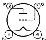
Thoriated-tungsten-filament type used as af power amplifier and modulator. Requires Small four-contact socket and may be mounted in vertical position with base down, or in horizontal position with pins 1 and 4 in vertical plane. **OUTLINE 29, Outlines Section.** Filament volts (ac/dc), 7.5; amperes, 1.25. Direct interelectrode capacitances: grid to plate, 6.4  $\mu\mu\text{f}$ ; grid to filament, 3.2  $\mu\mu\text{f}$ ; plate to filament, 2.6
