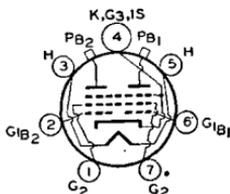
to 100 Mc and with reduced input up to 470 Mc. Class C Telegraphy maximum plate dissipation (per tube), CCS 20 watts, ICAS 25 watts. Requires Septar seven-contact socket and may be mounted in any position. *OUTLINE 14, Outlines Section.* Heater volts (ac/dc), 12.6 ± 10%; amperes, 0.625. Except for heater rating, the 6850 is identical with type 6524.
