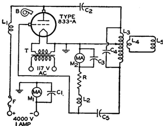
$C_1 C_3 = 0.01 \mu f$ , mica, 600 v.
