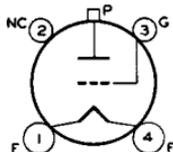
Thoriated-tungsten-filament type used as af power amplifier and modulator and as rf power amplifier and oscillator. May be used with full input up to 60 Mc and with reduced input
