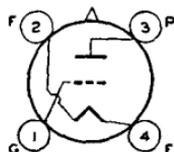
interelectrode capacitances: grid to plate, 14  $\mu\text{f}$ ; grid to filament, 5.7  $\mu\text{f}$ ; plate to filament, 4.4  $\mu\text{f}$ . **Maximum CCS ratings as RF POWER AMPLIFIER AND OSCILLATOR, CLASS C TELEGRAPHY:** dc plate volts, 1250 *max*; dc grid volts, -400 *max*; dc plate milliamperes, 175 *max*; dc grid milliamperes, 60 *max*; plate input, 220 *max* watts; plate dissipation, 100 *max* watts. Plate shows no color when
