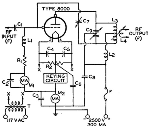
$C_1=0.0005 \mu\text{f}$ , mica, 1500 v.
