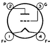
Coated-filament type used as af power amplifier and modulator and as rf power amplifier and oscillator. May be used with full input up to 6 Mc. For operation at 15 Mc, plate voltage
