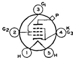
Heater-cathode type used as af power amplifier and modulator and as rf power amplifier and oscillator. May be used with full input up to 60 Mc. For operation at 80 Mc, plate voltage
