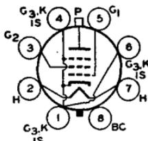
Rectangular-Wave Modulator maximum plate dissipation, 10 watts. Requires Octal socket and may be mounted in any position. **OUTLINE 17, Outlines Section.** Plate shows no color when tube is operated at maximum CCS ratings.
