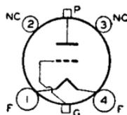
be reduced to 80 per cent of maximum ratings; at 350 Mc, to 53 per cent. Class C Telegraphy maximum CCS plate dissipation, 50 watts. Requires Small four-contact socket and may be mounted in vertical position only, base up or down. OUTLINE 44, *Outlines* Section. Plate shows an orange-red color when tube is operated at maximum CCS ratings.
