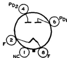
Coated-filament type used in power supply of transmitting and industrial equipment. Rated for a maximum peak inverse plate voltage of 2800 volts and maximum peak plate current of
