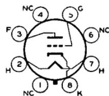
Glass-octal heater-cathode type used as rf power amplifier and oscillator. May be used with full input up to 30 Mc. For operation at 60 Mc, plate voltage and plate input should be reduced to 96 per cent of maximum ratings; at 90 Mc, to 93 per cent. Requires Octal socket and may be mounted in any position. OUTLINE 19, *Outlines* Section. Plate shows no color when tube is operated at maximum CCS ratings. The 1626 is used principally for renewal purposes.
