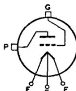
Maximum CCS ratings as RF POWER AMPLIFIER AND OSCILLATOR: dc plate volts, 3000 max; dc grid volts, -500 max; dc plate milliamperes, 500 max; dc grid milliamperes, 150 max; plate input, 1500 max watts; plate dissipation 600 max watts. The 6C24 is a DISCONTINUED type listed for reference only. As a replacement, the 5786 is a similar type although not directly interchangeable because of either electrical and/or mechanical differences.
