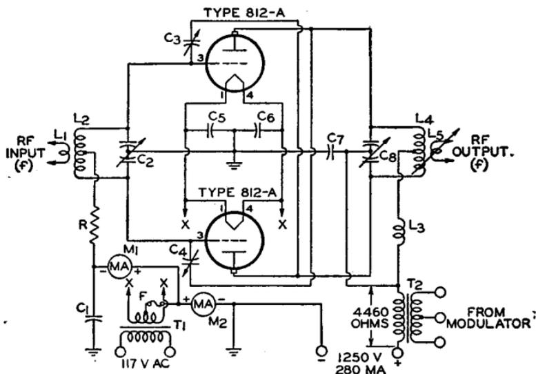
$C_1$   $C_5$   $C_6=0.005 \mu\text{f}$ , mica, 600 v.
