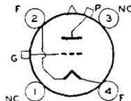
up to 100 Mc. Class C Telephony maximum plate dissipation, CCS 125 watts, ICAS 175 watts.
