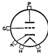
feet without pressurized chambers. May be used with full input up to 500 Mc and with reduced input up to 1700 Mc. Class C Telegraphy maximum plate dissipation, CCS 8 watts, ICAS 13 watts. May be mounted in any position. **OUTLINE 67, Outlines Section.** Cooling requirements for the 6264 are similar to those of type 6263.
