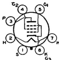
at 120 Mc, plate voltage and plate input should be reduced to 75 per cent of maximum ratings. Class C Telegraphy maximum plate dissipation, CCS 21 watts, ICAS 25 watts. Requires Octal socket and may be mounted in any position. OUTLINE 21, Outlines Section.
