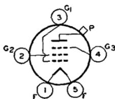
Thoriated-tungsten-filament type used as rf power amplifier and oscillator. May be used with full input up to 15 Mc and with reduced input up to 80 Mc. Requires Small five-contact socket and may be mounted in vertical position with base down, or in horizontal position with pins 2 and 4 in vertical plane. OUTLINE 48, *Outlines* Section. Plate shows no color when tube is operated at maximum CCS or ICAS ratings. The 804 is used principally for renewal purposes.
