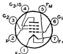
mobile and other communications equipment when compactness and low filament-power consumption are primary requirements. Designed for intermittent operation only. May be used with full input up to 100 Mc and with reduced input up to 165 Mc. Class C Telegraphy maximum ICAS plate dissipation, 5 watts.
