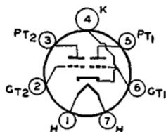
watts. Requires Septar seven-contact socket and may be mounted in vertical position with base up or down, or in horizontal position with pins 1 and 4 in vertical plane. **OUTLINE 16**, *Outlines* Section. Plates show no color when the tube is operated at maximum CCS ratings.
