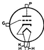
Compact liquid-and-forced-air-cooled type having heater-cathode used as af power amplifier and modulator, as rf power amplifier and oscillator, and as frequency multiplier. Coaxial
