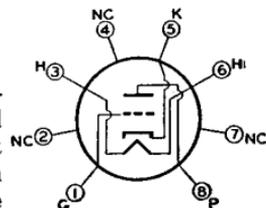
may be operated in any position. **OUTLINE 3**, *Outlines* Section. The flexible leads of the 5718 are usually soldered to the circuit elements. Soldering of the leads may be made close to the glass stem provided care is taken to conduct excessive heat
