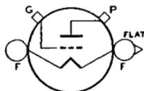
Mc with forced-air cooling), and with reduced input up to 75 Mc. Class C Telegraphy maximum plate dissipation with natural cooling, CCS 300 watts, ICAS 350 watts; with forced-air cooling, CCS 400 watts, ICAS 450 watts.
