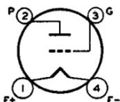
Coated-filament type used as a power amplifier and modulator and as rf power amplifier and oscillator. May be used with full input up to 45 Mc and with reduced input up to 100 Mc. Requires Small four-contact socket and may be mounted in vertical position with base down, or in horizontal position with pins 1 and 4 in vertical plane. **OUTLINE 29, Outlines Section.** Filament volts (ac/dc), 2.5; amperes, 2.5.
