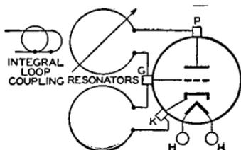
Pencil-type tube having integral resonators used in radiosonde service at 1680 Mc. Fixed-Tuned Oscillator maximum plate dissipation, 3.6 watts. May be mounted in any position. The 5794
