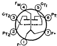
full input up to 40 Mc. Class C Telegraphy maximum CCS plate dissipation (each unit), 1 watt. Requires miniature seven-contact socket and may be mounted in any position. OUTLINE 6, *Outlines* Section. For filament considerations, refer to type 3A4, noting that for type 3A5 pin 4 is the filament mid-tap. Plates of the 3A5 show no color when the tube is operated at CCS ratings.
