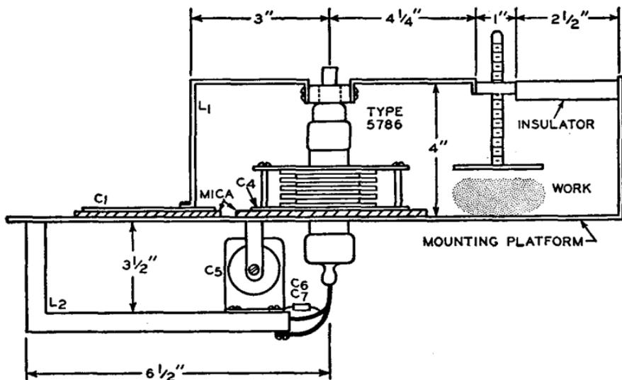
C<sub>1</sub>=250 μμf, mica 0.005 inch thick, 3 inches x 3 3/4 inches copper plate, held to mounting platform by insulated pressure clamps
