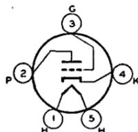
Heater-cathode type used as rf power amplifier and oscillator. May be used with full input up to 6 Mc and with reduced input up to 30 Mc. Requires Small five-contact socket and may be mounted in any position. **OUTLINE 29, Outlines Section.** Heater volts (ac/dc), 2.5; amperes, 2.5. Direct interelectrode capacitances: grid to plate, 3.9  $\mu\mu\text{f}$ ; grid to cathode and heater, 4  $\mu\mu\text{f}$ ; plate to cathode and heater,
