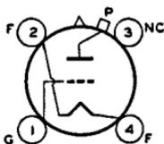
Thoriated-tungsten-filament type used as af power amplifier and modulator and as rf power amplifier and oscillator. May be used with full input up to 30 Mc and with reduced input up to 50 Mc. Requires Jumbo four-contact socket and may be mounted in vertical position with base down, or in horizontal position with pins 1 and 3 in vertical plane. *OUTLINE 50, Outlines Section.* For operation at 50 Mc,
