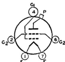
input up to 250 Mc. Class C Telephony maximum CCS plate dissipation, 65 watts. Requires Septar seven-contact socket and may be mounted in vertical position only, base up or down. OUTLINE 23, *Outlines* Section. Plate shows an orange-red color when the tube is operated at maximum CCS ratings.
