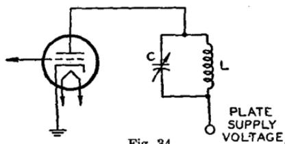
frequency,  $f$ , of such a circuit in megacycles per second is given by
