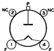
Coated-filament type used in power supply of transmitting and industrial equipment. Maximum peak inverse plate volts, 6000; maximum average plate amperes, 0.13. Requires a
