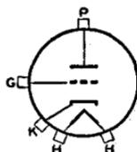
3300 Mc. Designed for use in coaxial-cylinder-type circuits, it may also be used in parallel-line and lumped circuits. Class C Telegraphy maximum plate dissipation, CCS 7 watts, ICAS 8 watts. May be mounted in any position. OUTLINE 66, *Outlines* Section.
