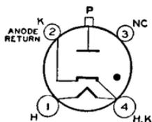
Heater-cathode type used in power supply of transmitting and industrial equipment. Maximum peak inverse anode volts, 5,000; maximum average anode amperes, 2.5. Requires
