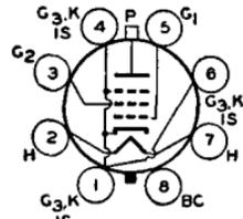
reduced input up to 175 Mc. Class C Telegraphy maximum plate dissipation, CCS 20 watts, ICAS 25 watts. OUTLINE 17, *Outlines* Section. Heater volts, 26.5 ± 10%; amperes, 0.3. Except for heater rating, this type is identical with type 6146.
