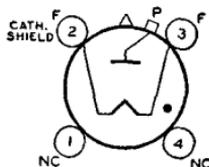
Super-Jumbo four-contact socket and may be mounted in vertical position only, base down. **OUTLINE 62**, *Outlines* Section. The 673 is electrically identical with the 575-A.
