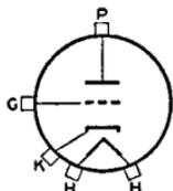
Pencil-type tube used in cathode-drive circuits as rf power amplifier and oscillator. Designed for use in coaxial-cylinder-type circuits, it may also be used in parallel-line or lumped circuits.
