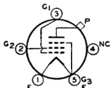
Coated-filament type used as rf power amplifier and oscillator. May be used with full input up to 60 Mc. For operation at 80 Mc, plate voltage and plate input should be reduced to 80 per cent of maximum ratings; at 125 Mc, to 55 per cent. Requires Small five-contact socket and may be mounted in vertical position only, base up or down. OUTLINE 31, *Outlines* Section, except has no bayonet pin. Plate shows
