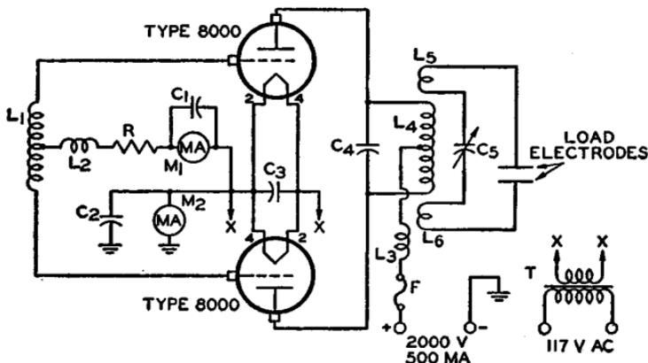
$C_1 C_2 C_3 = 0.005 \mu f$ , mica, 600 v.
