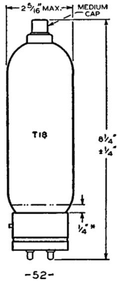
\* Zone where condensed-mercury temperature should be measured.
