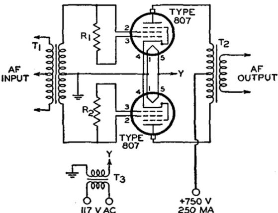
R<sub>1</sub> R<sub>2</sub>=20000 ohms, 1 watt, carbon
