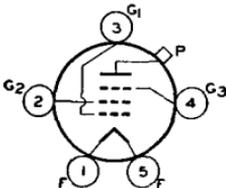
Thoriated-tungsten-filament type used as af power amplifier and modulator and as rf power amplifier and oscillator. May be used with full input up to 30 Mc. For operation at 50 Mc,
