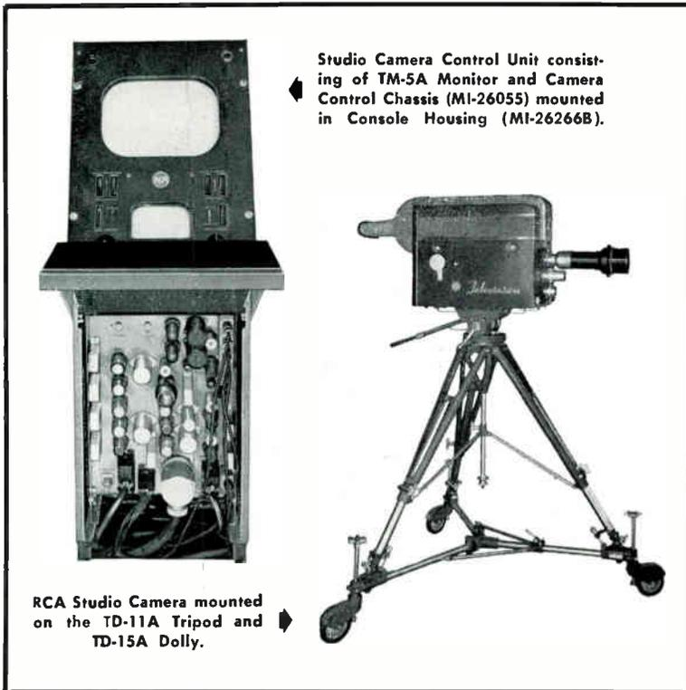
Studio Camera Control Unit consisting of TM-5A Monitor and Camera Control Chassis (MI-26055) mounted in Console Housing (MI-26266B).
