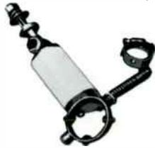
Spring hanger for single line. Complete with clamps and pivot bolt to compensate for line misalignment. Spring must be preloaded at installation.
