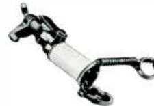
Spring hanger for single line. Complete with clamp and pivot bolt to compensate for line misalignment. Spring must be preloaded at installation.
