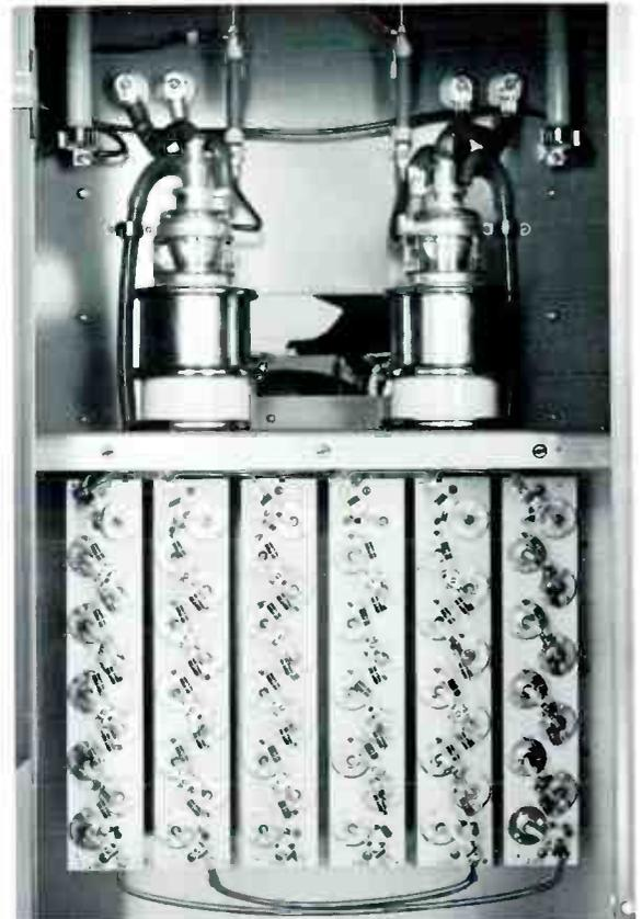
Modulator tubes and silicon high voltage rectifiers with cover removed.
