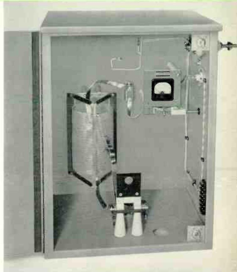
Basic 1 KW Antenna Tuning Unit, MI-27767-A.
