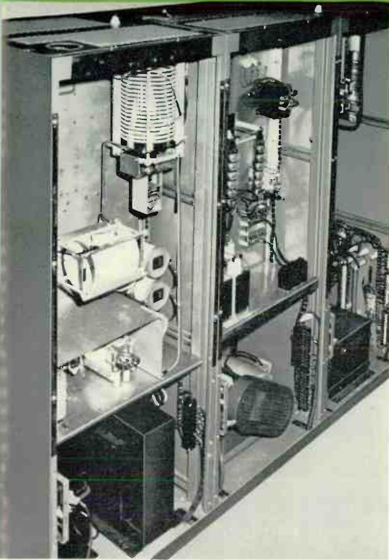
Rear view of transmitter showing reach-in accessibility to transmitter facilities. The modulation transformer and final PA tank circuitry are seen in foreground, rear of modulator and blower in center cabinet, while heavier components of driver are shown mounted on floor of third cabinet.
