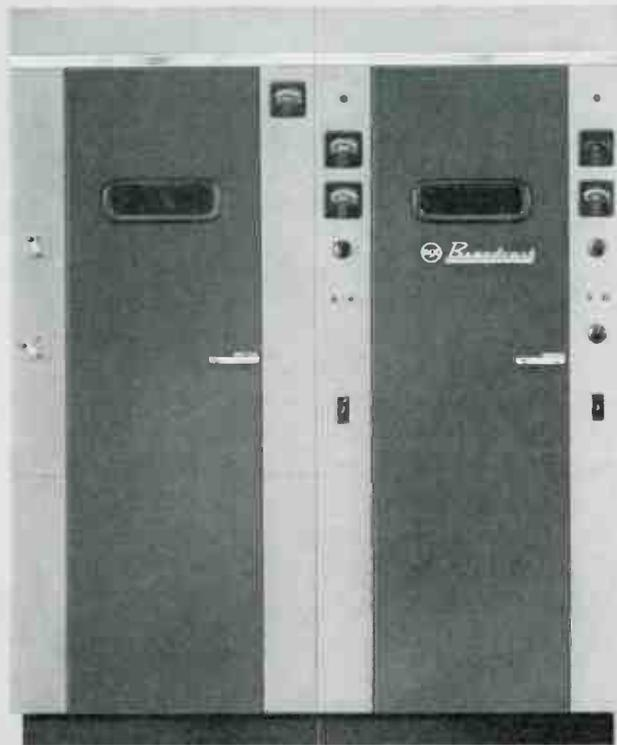
BTA-1R Transmitter with matching left-wing phasing cabinet.
