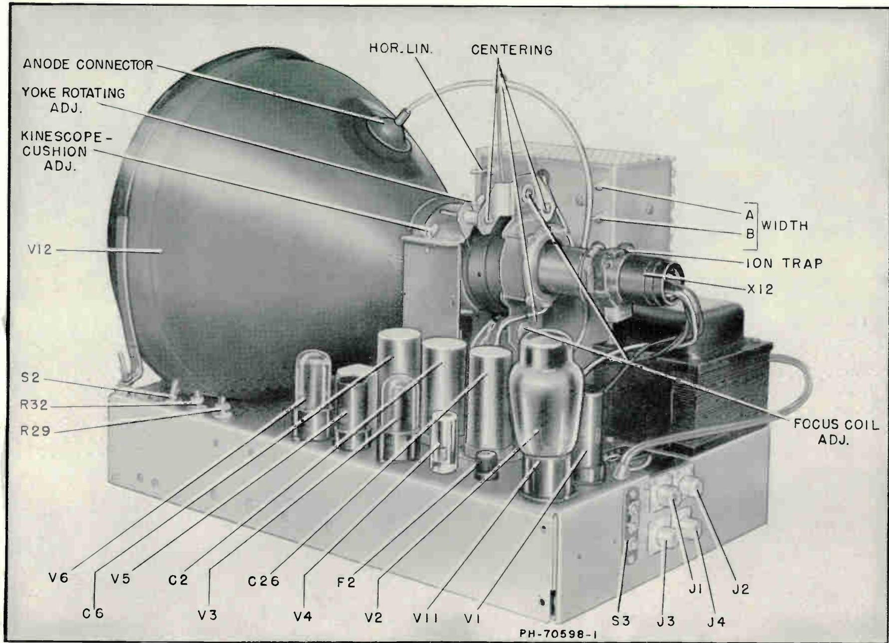
Figure 5. - Utility Monitor, Bottom View
