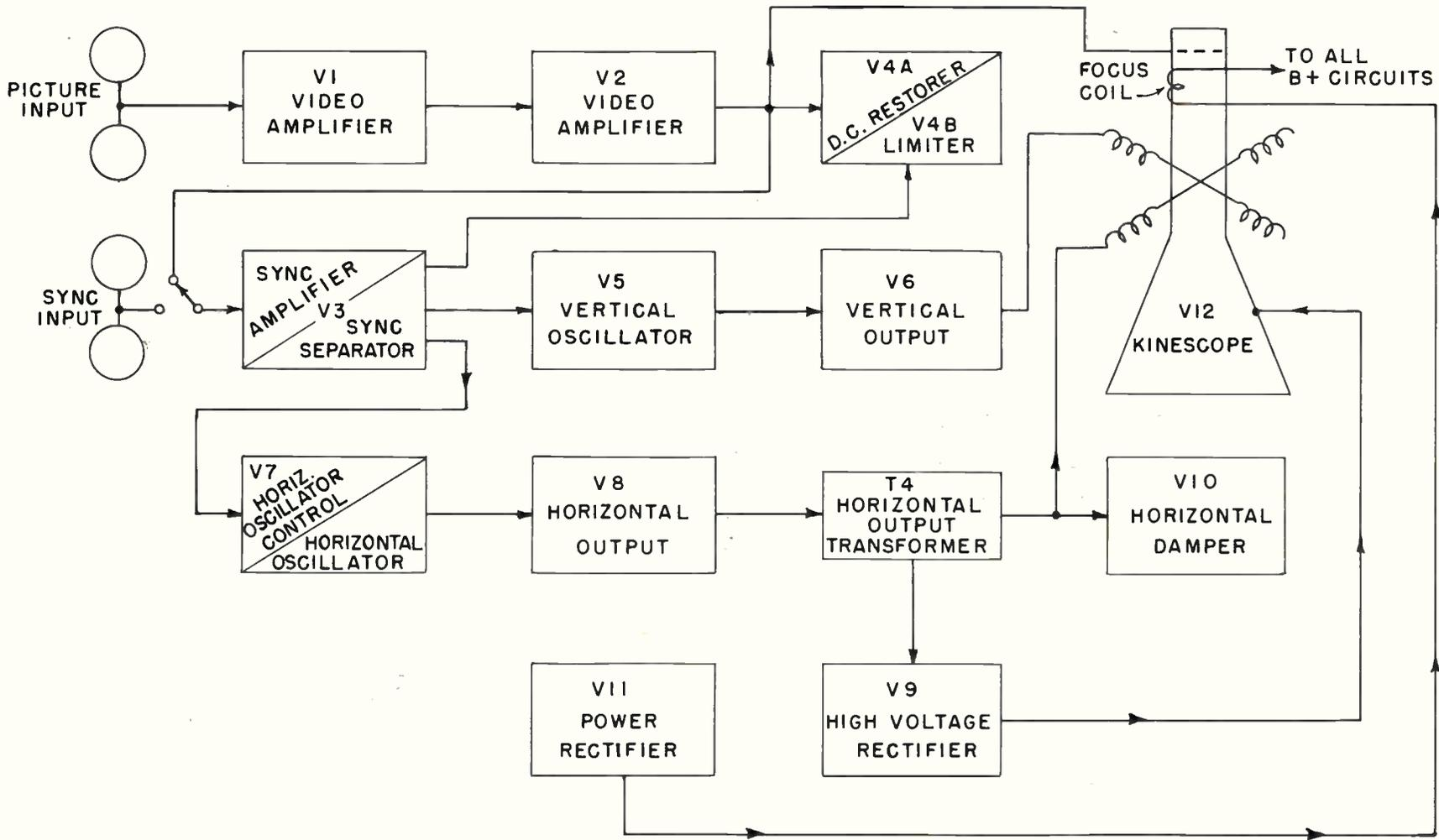
Figure 1. - Utility Monitor, Block Diagram
