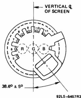
**Figure 5 - Pin Connections and Rear View of Base - EIA No.B8-295-AA**
