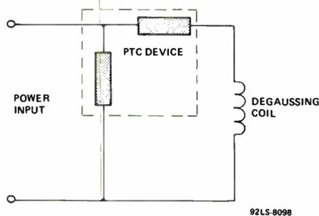
**Figure 7 - Typical Degaussing Circuit**
