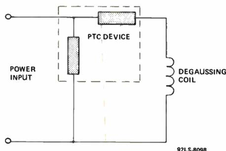
**Figure 7 - Typical Degaussing Circuit**
