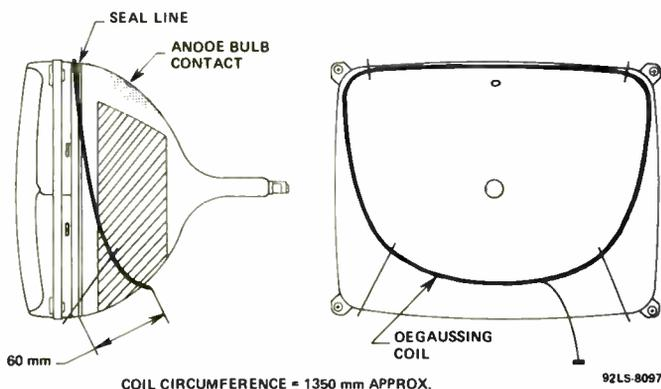
**Figure 6 - Relative Placement of Typical Tilted "Z" Degaussing Coil**
