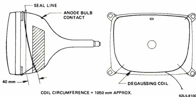
**Figure 6 - Relative Placement of Typical Tilted "Z" Degaussing Coil**
