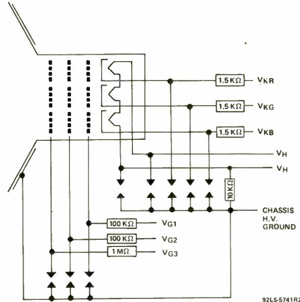
**Figure 8 - Picture-Tube Connections Showing Spark-Gap Recommendations and Typical Isolation-Resistor Values**
