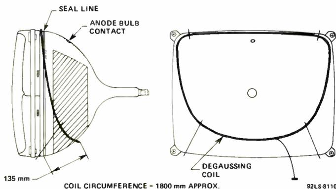
**Figure 6 - Relative Placement of Typical Tilted "Z" Degaussing Coil**
