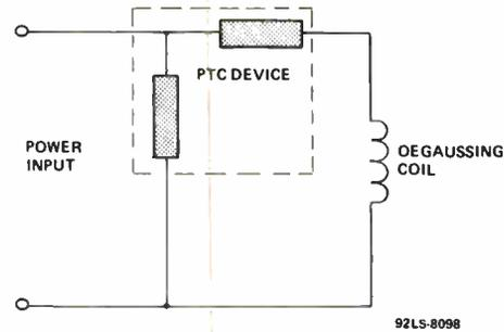
**Figure 7 - Typical Degaussing Circuit**
