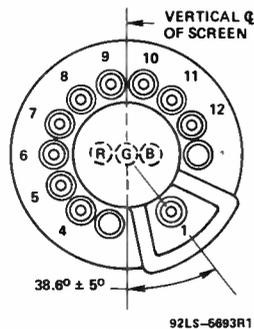
Figure 5 - Pin Connections and Rear View of Base - EIA No.B10-276-AB
