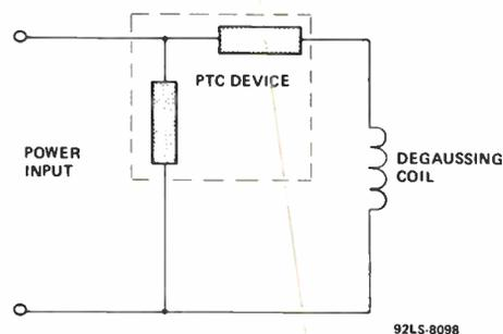
**Figure 7 - Typical Degaussing Circuit**
