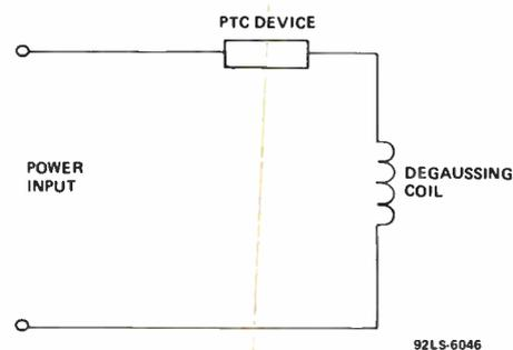
**Figure 7 - Typical Degaussing Circuit**
