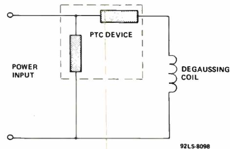
**Figure 7 - Typical Degaussing Circuit**
