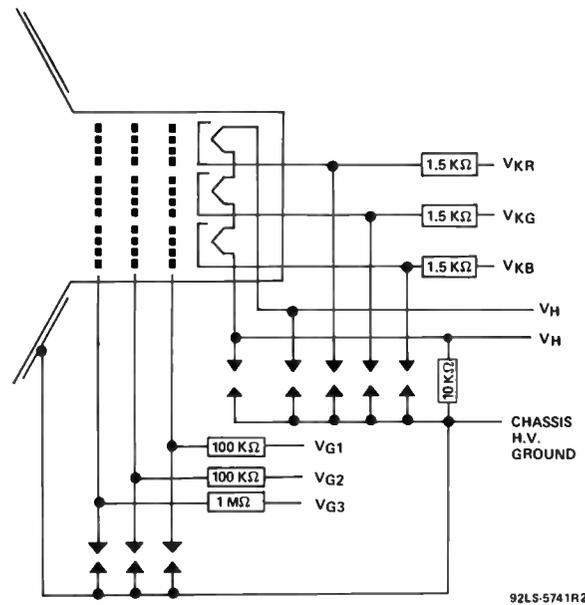
**Figure 8 - Picture-Tube Connections Showing Spark-Gap Recommendations and Typical Isolation-Resistor Values**
