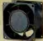
(1) 3" Brushless DC Fan. Surprisingly light weight yet powerful. Produces 27 cubic feet per minute airflow. Ideal for cooling circuitry sensitive to hum or AC fields created by 120 VAC fans. Ball bearings for long life and low noise. -34 dB, max. 3<sup>5</sup>/<sub>32</sub> x 3<sup>5</sup>/<sub>32</sub> x 1<sup>1</sup>/<sub>2</sub>". Requires 7 to 13.8 VDC. 273-243 ..... 14.95
