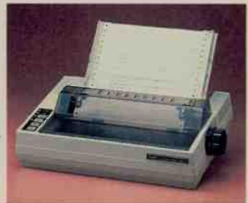
DMP 130. Correspondence printing for under \$350! Prints in four character styles: standard or italic cursive in draft or correspondence modes. Supports super/subscripts, double-width, bold, double-strike, plus cursive and microfont styles. Prints up to 100 characters per second. Built-in tractor. Parallel and Color Computer serial interfaces. UL listed AC. 26-1280 ..... 349.95
