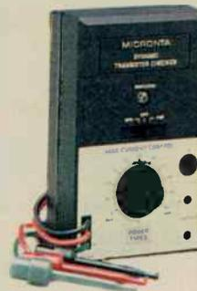
An inexpensive yet very useful addition to your workbench! Lets you make fast good/bad tests on small-signal and power transistors. Also allows you to match similar transistors. Lamp indicates relative current gain, "opens" and "shorts". Has a front-panel pin socket plus color-coded hook-clip leads for in-circuit tests. Output jacks let you connect to an external meter or scope for more in-depth tests. 2 3/4" x 4 3/8" x 1 3/16". With instructions. Requires "AA" battery. 22-025 ..... 14.95
