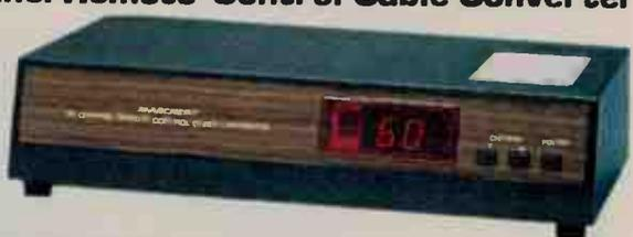
Pushbutton wireless remote lets you scan cable channels in two directions, access them directly, fine-tune and turn TV on/off. PLL tuning system assures optimum performance. Has standard/HRC switch for use on all cable systems, LED digital display, channel 3 output. 2<sup>3</sup>/<sub>8</sub> x 11<sup>1</sup>/<sub>2</sub> x 6<sup>1</sup>/<sub>2</sub>". FCC registered. UL listed AC. Remote requires 9V battery. 15-1285 . . . . . 119.95
