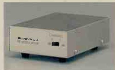
Converts line-level (baseband) signals from a satellite TV receiver, portable VCR, computer or video camera to VHF for reception on a standard TV. 1k/75-ohm video input selector matches most equipment. RCA-type phono jacks for video and audio input. 75-ohm "F" connector for output to TV. FCC registered. 1<sup>1</sup>/<sub>2</sub> x 3<sup>9</sup>/<sub>16</sub> x 4<sup>3</sup>/<sub>4</sub>". UL listed AC. 15-1273 ..... 24.95
