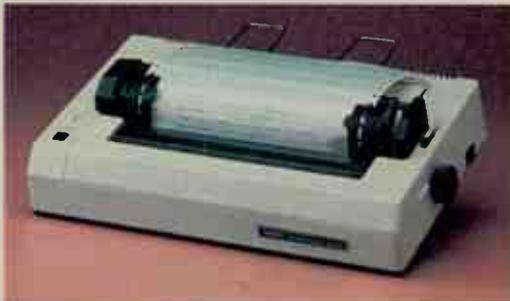
DMP 105. Another Radio Shack price breakthrough! Ideal for data processing and general-purpose use. Produces crisp 8 x 9 characters on an 8" line. Bidirectional—prints 80 upper and lowercase characters per line at 43 lines per minute (10 characters per inch). Features elongated and condensed modes. Parallel and Color Computer-compatible serial interfaces. UL listed AC. 26-1276 ..... 199.95
