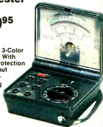
Fuse/surge-absorber protected. Sensitivity: 20,000 ohms per volt DC. Measures to 1200 volts DC in seven ranges, 1200 volts AC in five ranges, DC current to 300 mA in four ranges, resistance to two megohms in four ranges, and decibels - 20 to + 63 in five ranges. Accuracy ± 3% DC, ± 4% AC. Open, 7<sup>1</sup>/<sub>4</sub> x 4<sup>5</sup>/<sub>16</sub> x 1<sup>1</sup>/<sub>4</sub>". Requires "AA" battery. 22-211 ..... 29.95
