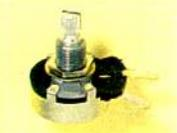
25 Ohms. Wirewound pot useful for speaker attenuation and fine circuit adjustment. Tolerance:  $\pm 20\%$ . Rated 2 watts continuous, 5 watts intermittent. 271-265 Pkg. of 2/79¢
